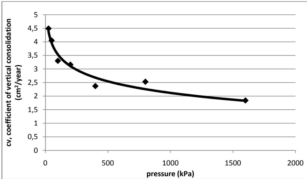
*Figure 3.14  $c_v$  versus  $\sigma$  graph*
