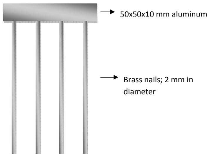
*Figure 3.3 Schematic representation of the simple case*
