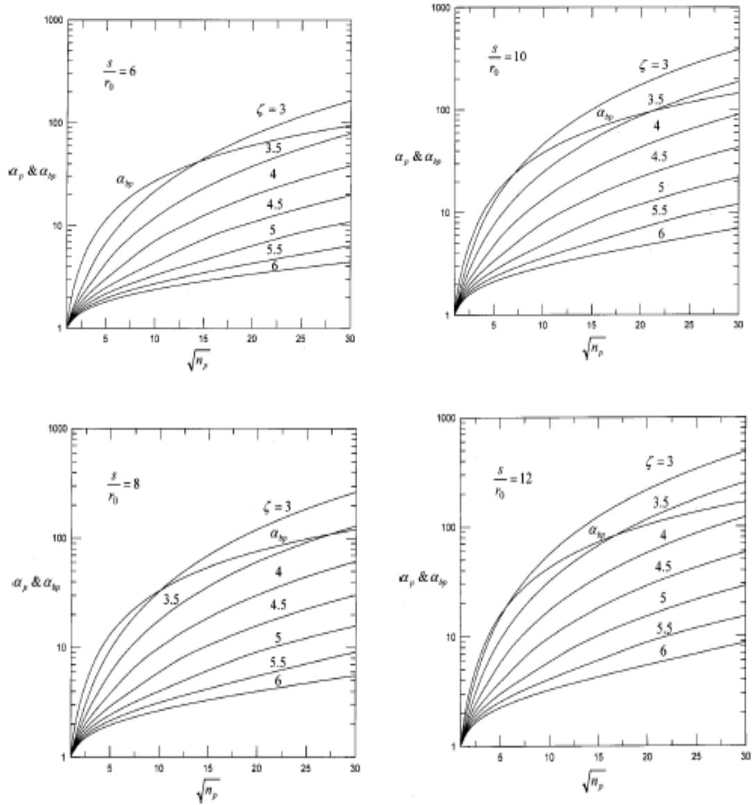
Figure 2.12 Coefficients  $\alpha_p$  and  $\alpha_{bp}$  versus number of piles (Shen and Teh, 2002)
