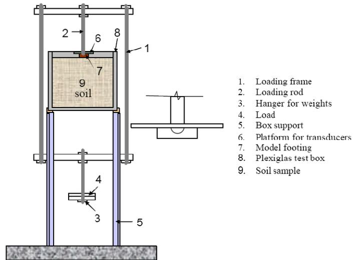
*Figure 3.10 Schematic representation of the system (Engin, 2005 after Kul, 2003)*
