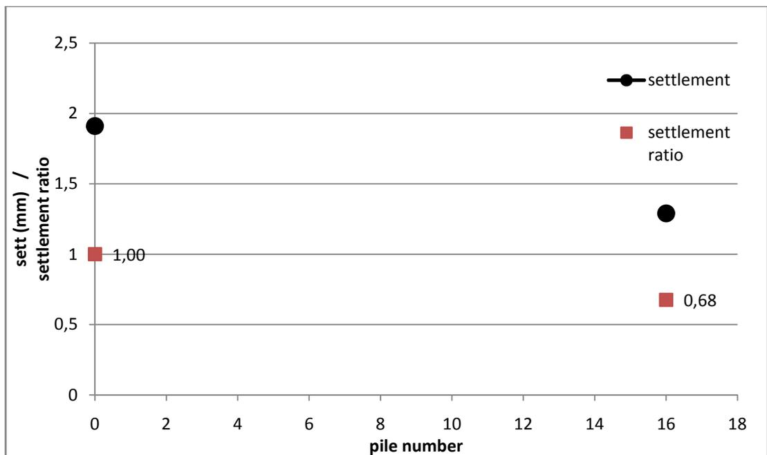
*Figure 3.19 Pile number versus settlement graph at 40 kPa pressure*
