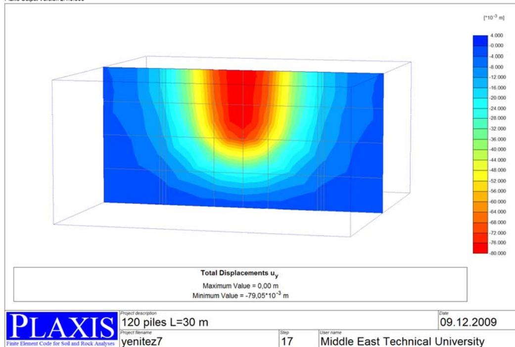
Figure 4.8 Output graph for 120 piles L=30 m
