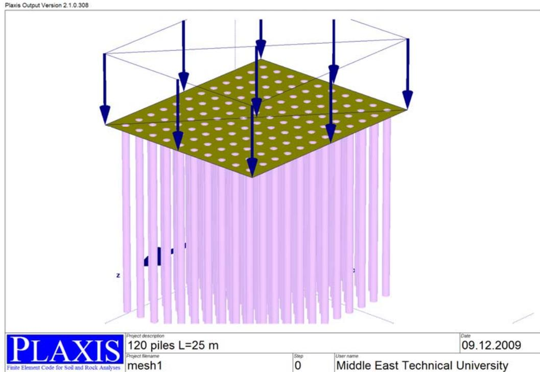
**Figure 4.3 Model designed for 120 piles in Plaxis 3D Foundation**
