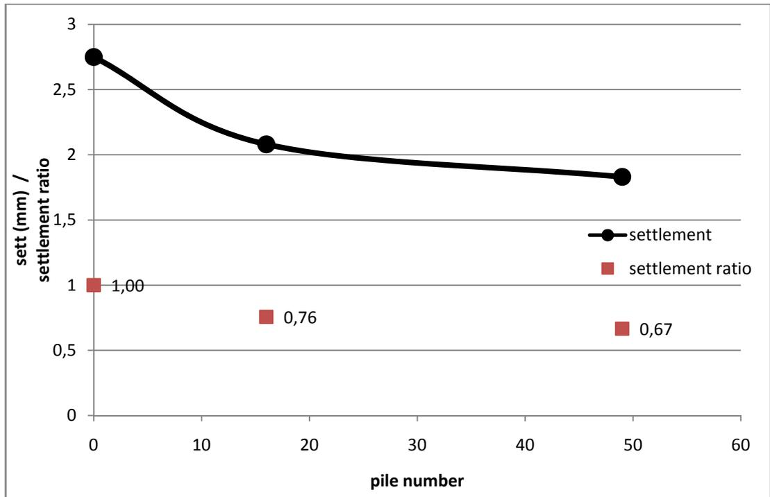
*Figure 3.20 Pile number versus settlement graph at 75 kPa pressure*
