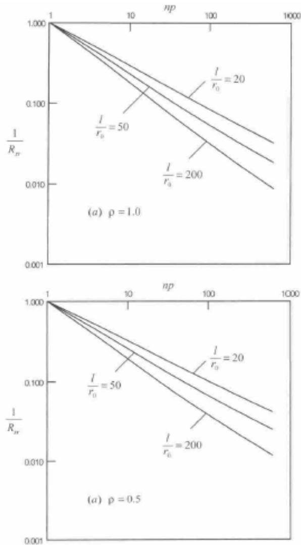
Figure 2.10 Graph of  $1/R_{sr}$  versus number of piles for  $s/r_0=10$ ,  $v_s=0.2$  (Shen et al, 2000)
