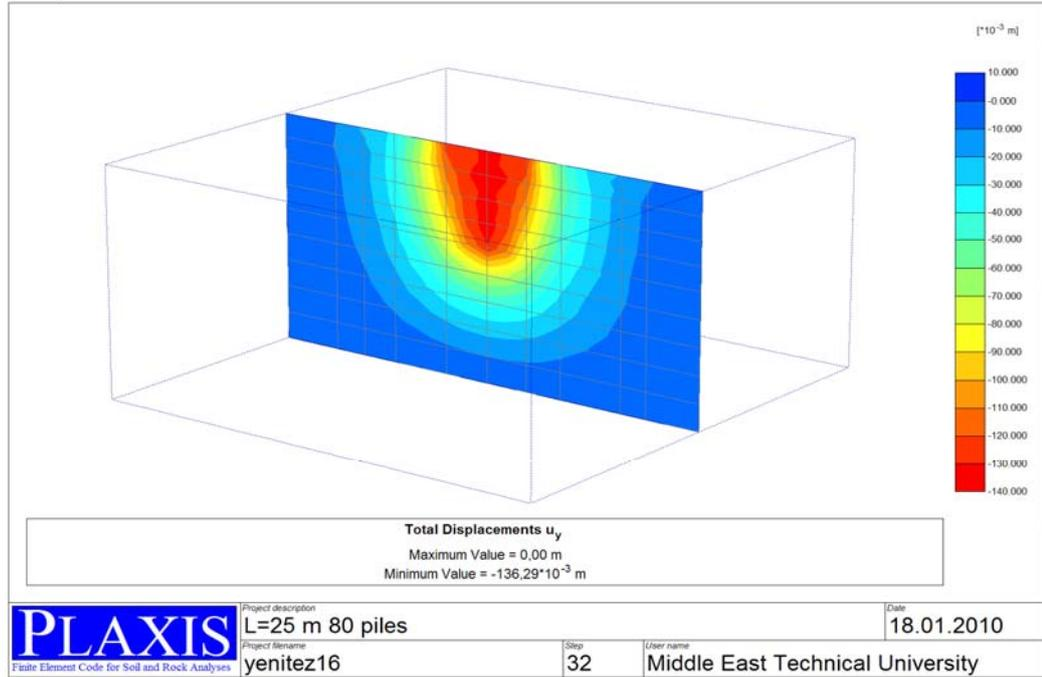
Figure 4.7 Output graph for 80 piles L=25
