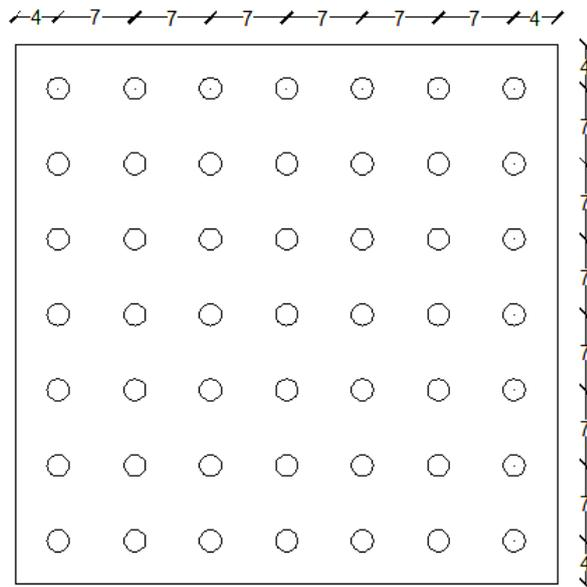
**Figure 3.22 Pattern for 49 piles (all in m)**
