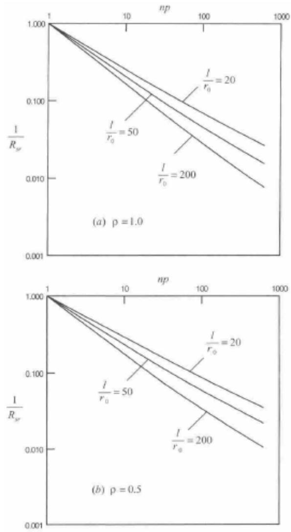
**Figure 2.9 Graph of  $1/R_{sr}$  versus number of piles for  $s/r_0=6$ ,  $v_s=0.5$  (Shen et al, 2000)**
