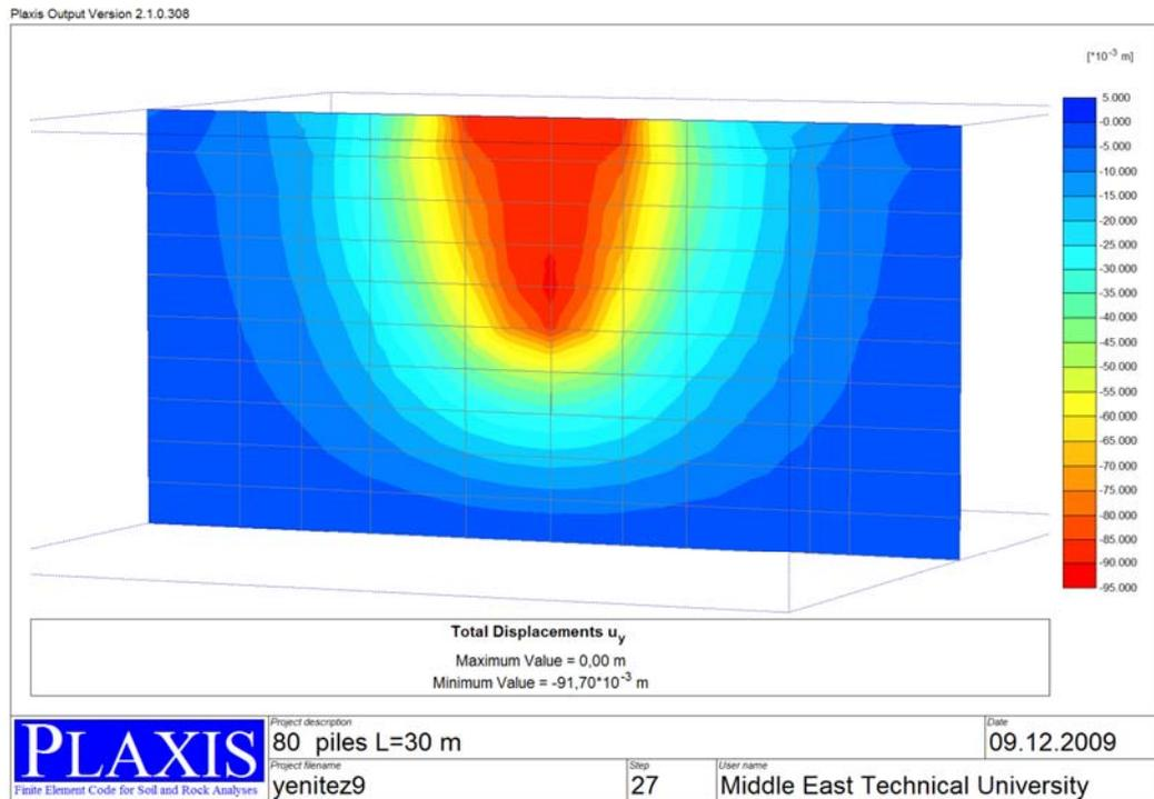
*Figure 4.10 Output graph for 80 piles L=30 m*
