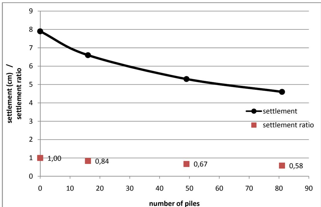
*Figure 3.24 Settlement versus pile number relationship for 40 kPa pressure*
