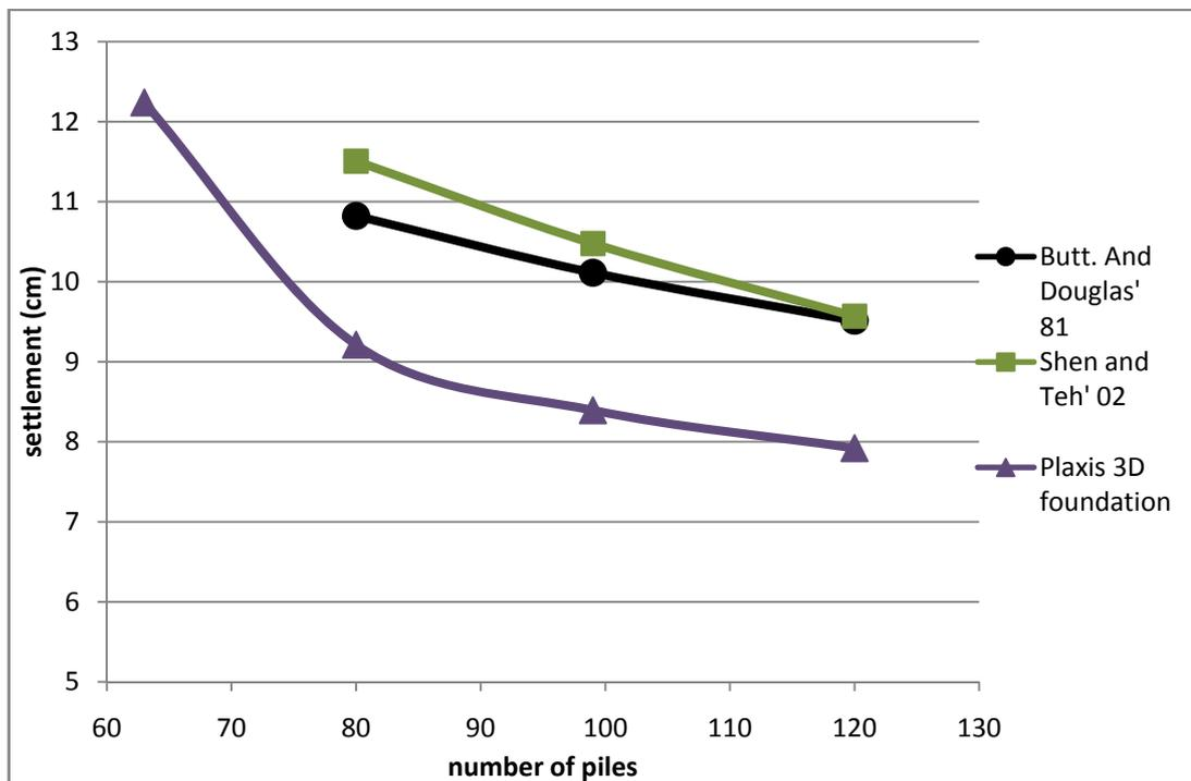
*Figure 5.3 Graphical representation of the combined results for 30 m piles*
