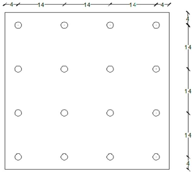
**Figure 3.21 Pattern for 16 piles (all in m)**
