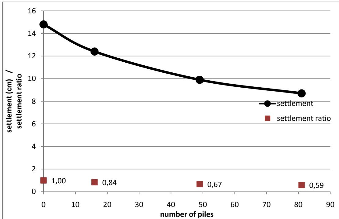
*Figure 3.23 Settlement versus pile number relationship for 75 kPa pressure*
