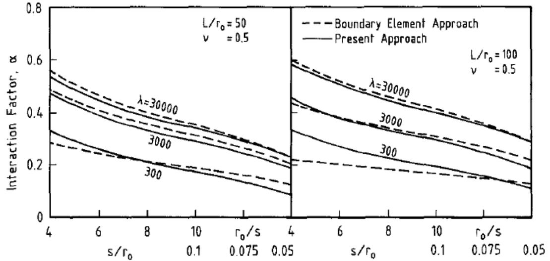
*Figure 2.5 Effects of pile spacing and stiffness relative to soil for nonhomogeneous soil*
