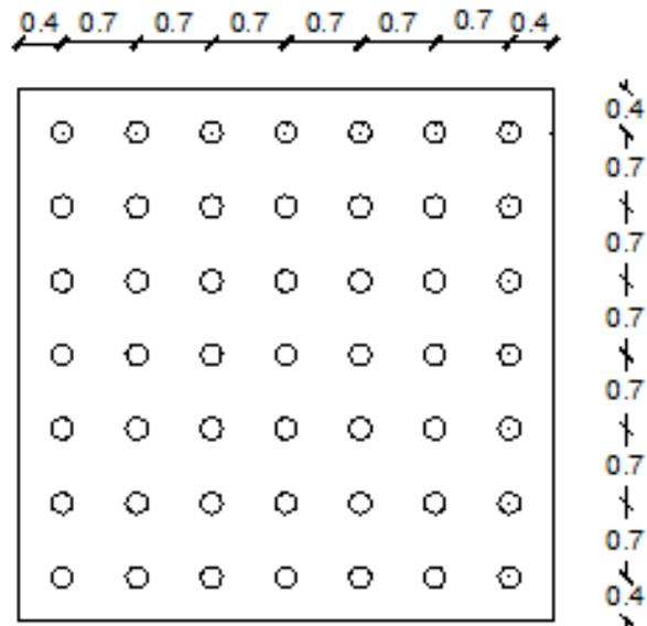
*Figure 3.17 Pattern for 49 piles (all in cm)*
