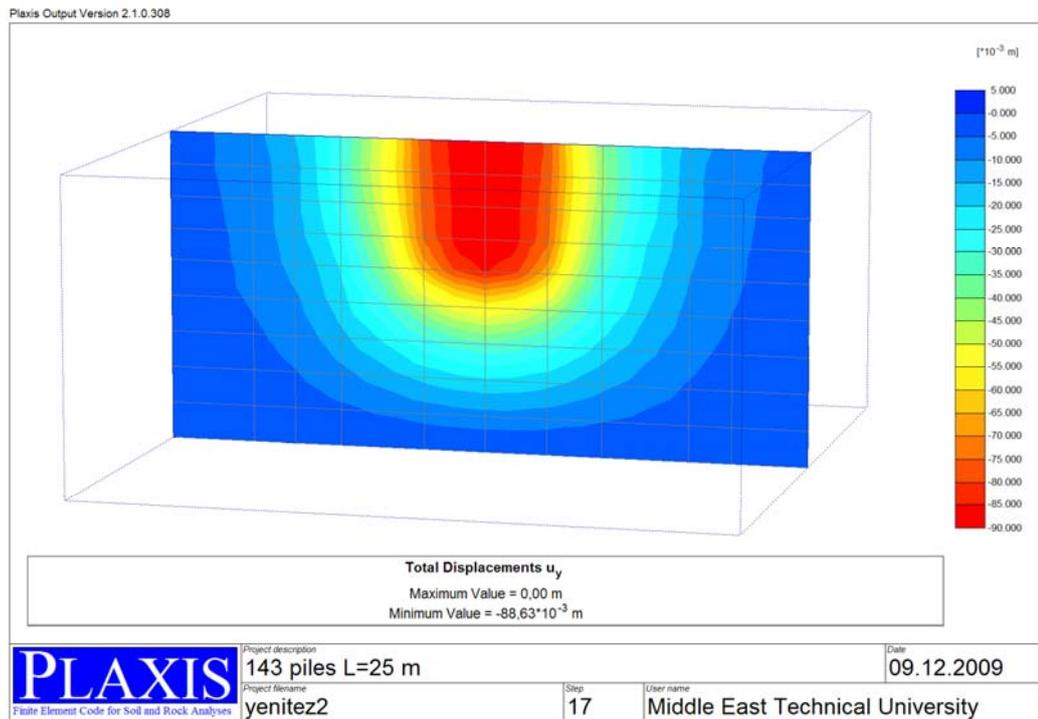
**Figure 4.4 Output graph for 143 piles L=25 m**
