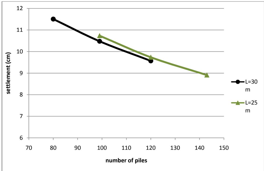
*Figure 4.2 Graphical results for load transfer curve analysis*
