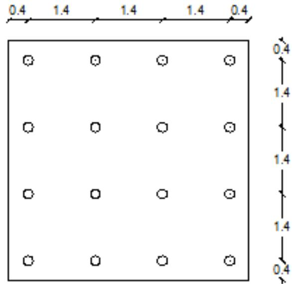
*Figure 3.16 Pattern for 16 piles (all in cm)*
