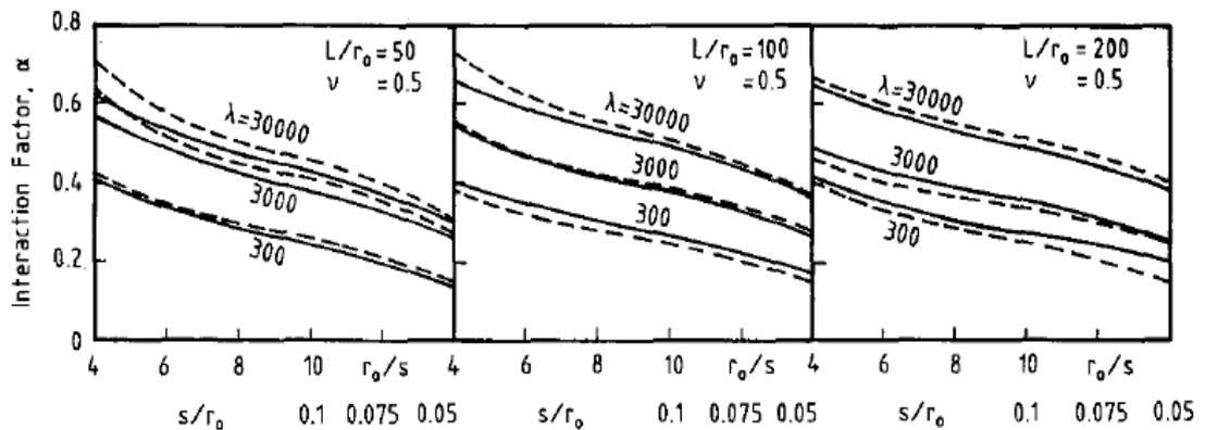
**Figure 2.4 Effects of pile spacing and stiffness relative to soil for homogeneous soil (Lee, 1993)**
