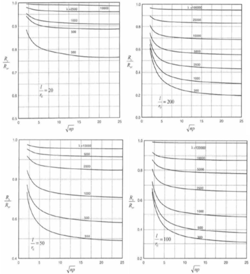
Figure 2.11 Normalized group settlement ratio versus number of piles (Shen et al, 2000)
