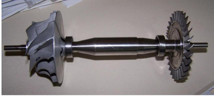
**Figure 3-11 AMT OLYMPUS HP Engine's Shaft**
