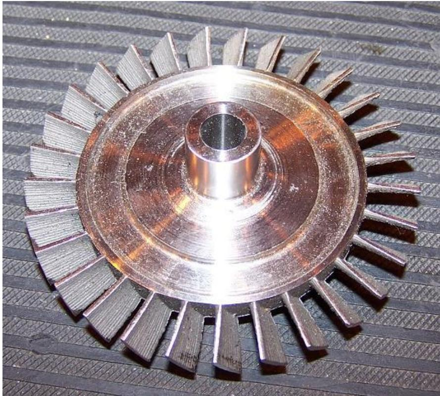
**Figure 3-9 Turbine of AMT Olympus HP**
