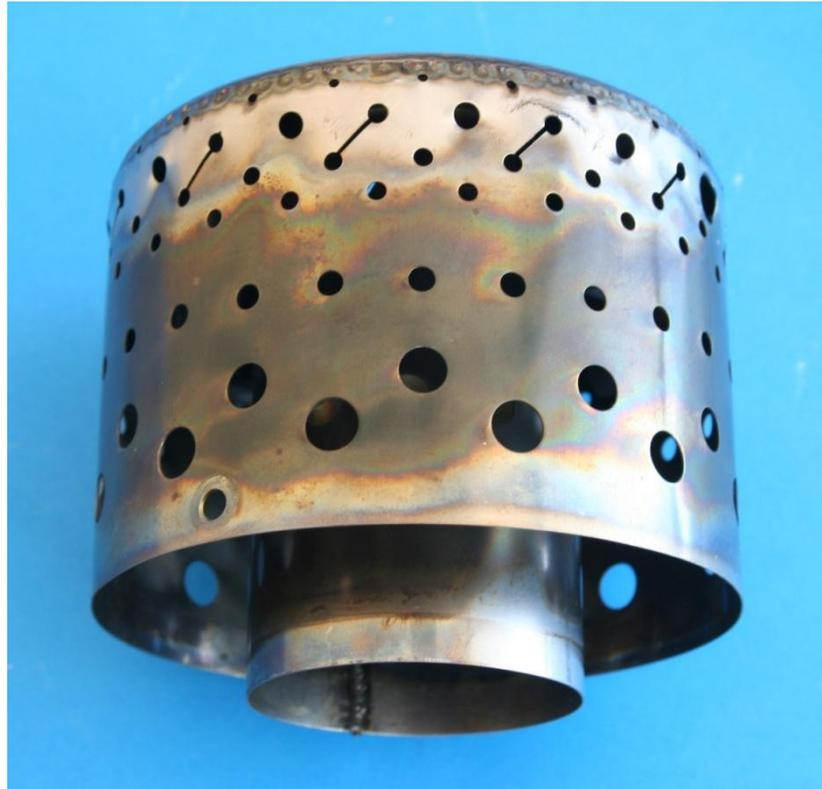
**Figure 3-7 Combustion Chamber of AMT Olympus HP**
