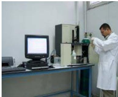
Figure 2.14: Quantachrome Corporation, Poremaster 60 [41]
