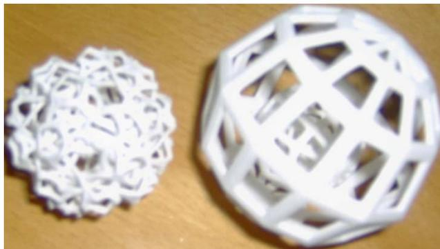
Figure 1.2: Examples of complex geometry parts produced via RP methods produced at the Biltir Center; METU
