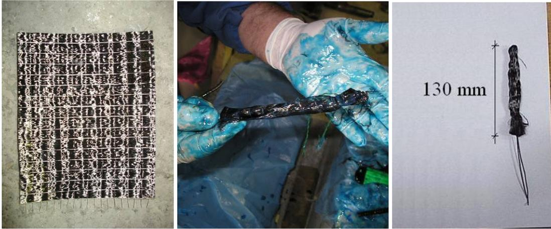
(a) CFRP anchor dowel preparation
