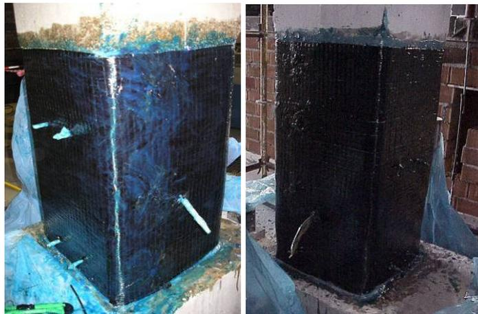
Figure 2.9 CFRP strengthened and repaired columns ready for the test
