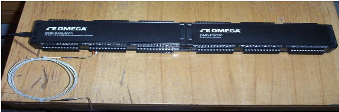
**Figure 3.9 Omega OMB-DAQ-3005 with QMB-PDQ 30 Expansion Module**
