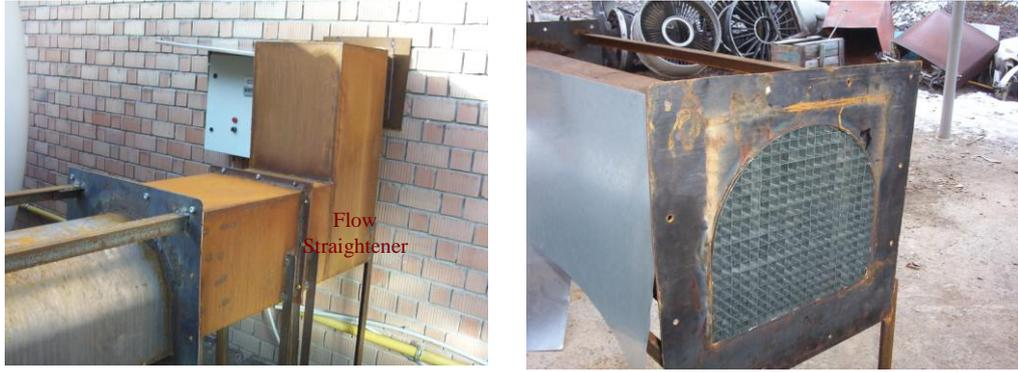
**Figure 3.5 Flow Straightener**
