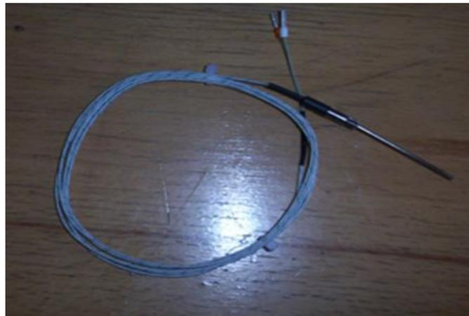
**Figure 3.8 K Type Thermocouple**
