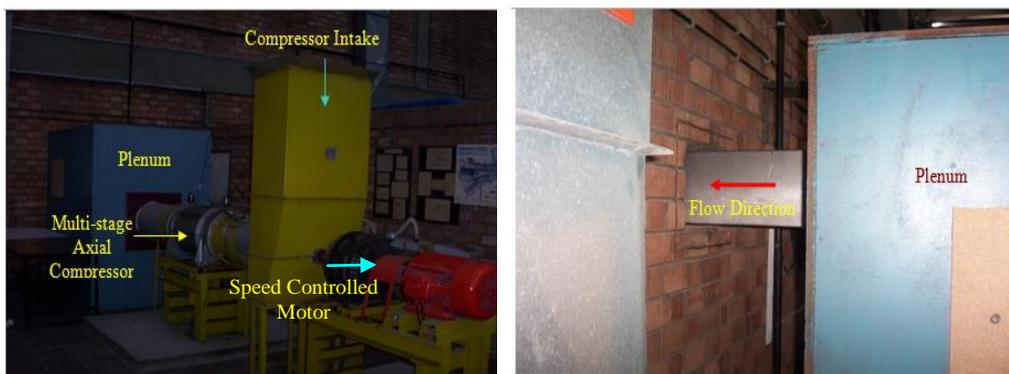
**Figure 3.4 Flow Driven System and Auxiliary Connections**
