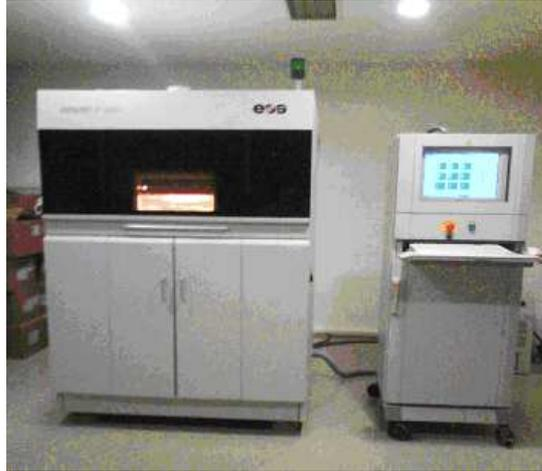
Figure 3.1: EOSINT P380 Laser sintering machine in Biltir, METU
