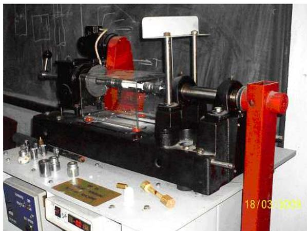
Figure 3.29: SM21 Torsion test machine, Mechanics and Strength Lab, Gazi Uni.
