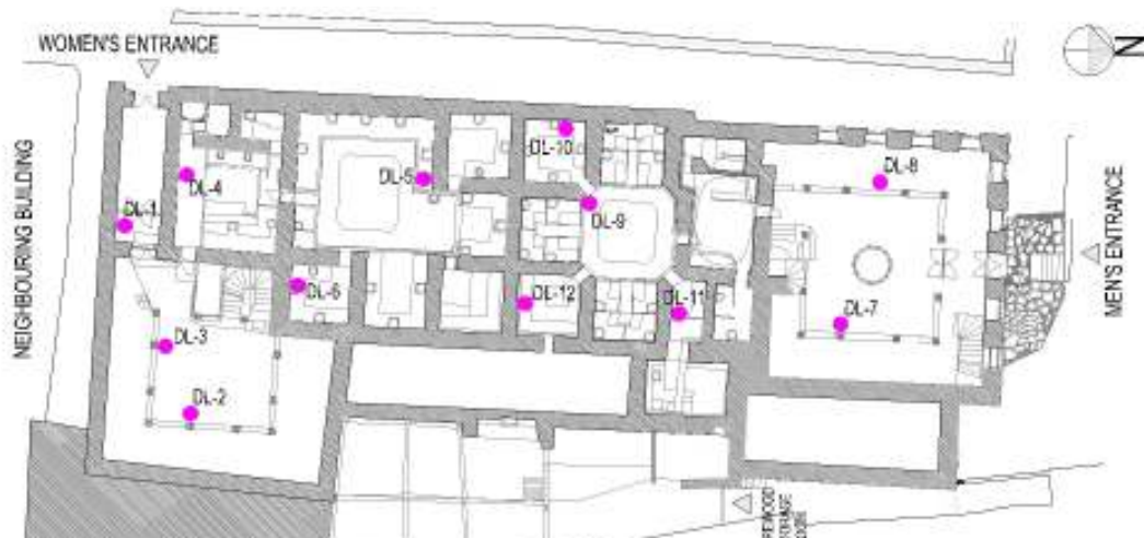
Figure 3.14 Plan showing the distribution of data loggers in different parts of Şengül Hamamı (Source: Archives of the General Directorate of Pious Foundations, 2008; produced by the author).
