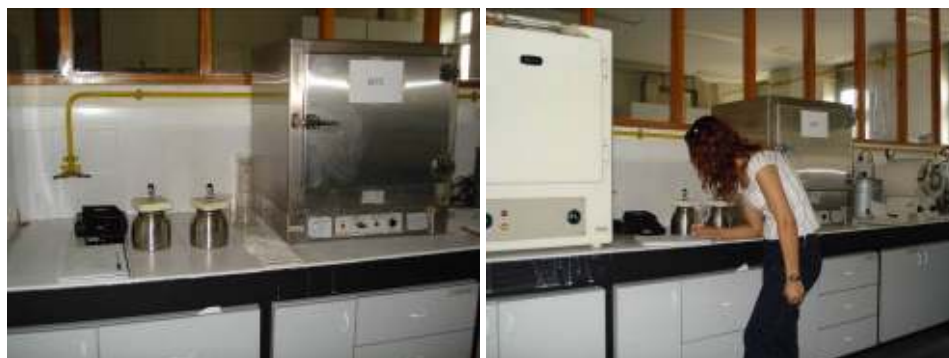
Figure 3.13 Photographs showing the experimental setup for the determination of specific heat capacity values of historic samples.
