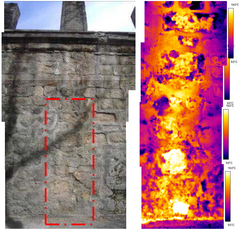
Figure 4.11 A partial view from the west wall of men's hot space on the axis of chimney and its IR image showing that surface temperatures of the wall were warmer than the ambient temperature of 2.8°C in February, at night, with a temperature difference of 12.5°C.
