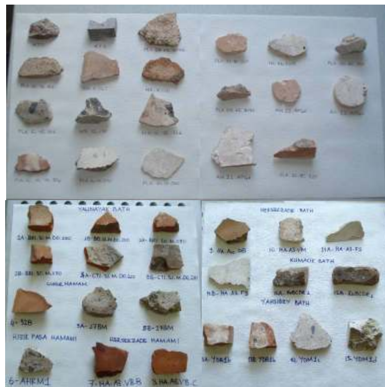
Figure 3.11 Samples of historic brick, stone, brick and stone mortar, interior and exterior plasters collected from the historical baths belonging to the same period with Şengül Hamamı.
