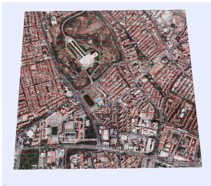
Figure 36 Base Texture with intensity value 1.0. Base texture is seen but tile textures are not seen.
