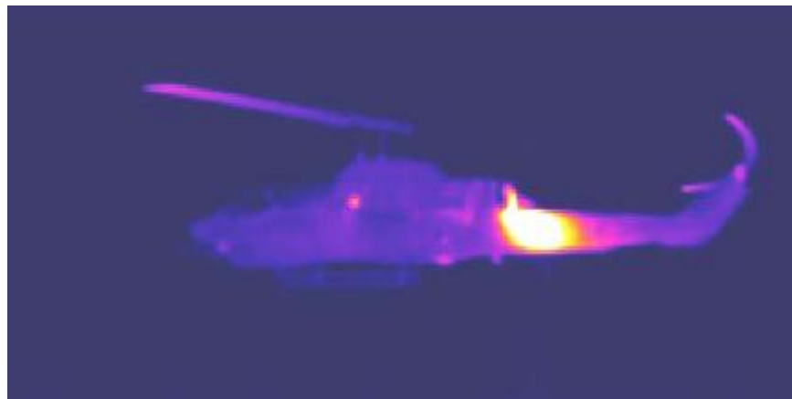
Figure 2 – IR image of AH-1W in hover [2]
