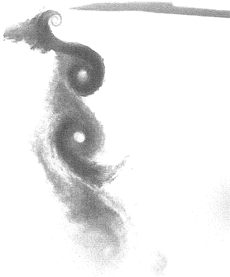
Figure 6 – Blade tip vortices [11]
