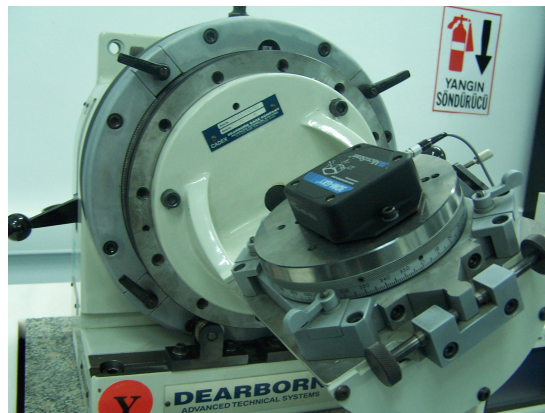
Figure 2- Index table with 3DM-GX1 shown on top (330 degrees orientation around the sensor y-axis)
