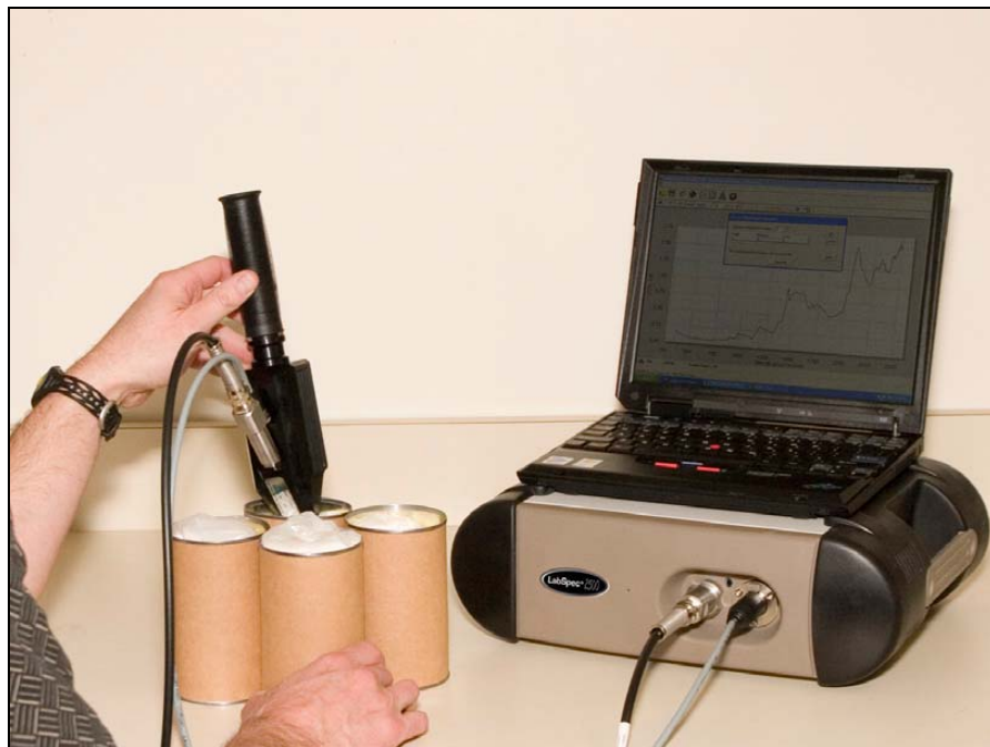
Figure 4.4 General view of ASD Labspec 2600 portable spectrometer (ASD, 2009).
