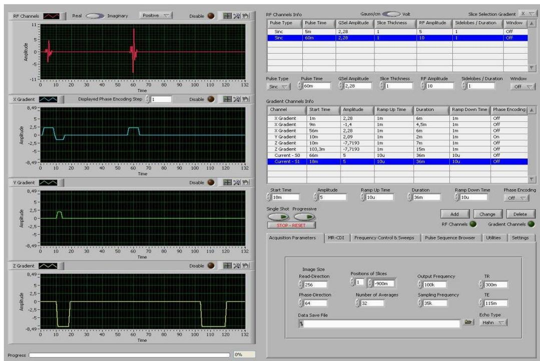
Figure A.10 Screen Shot Image of MRI software for  $B_x$  imaging
