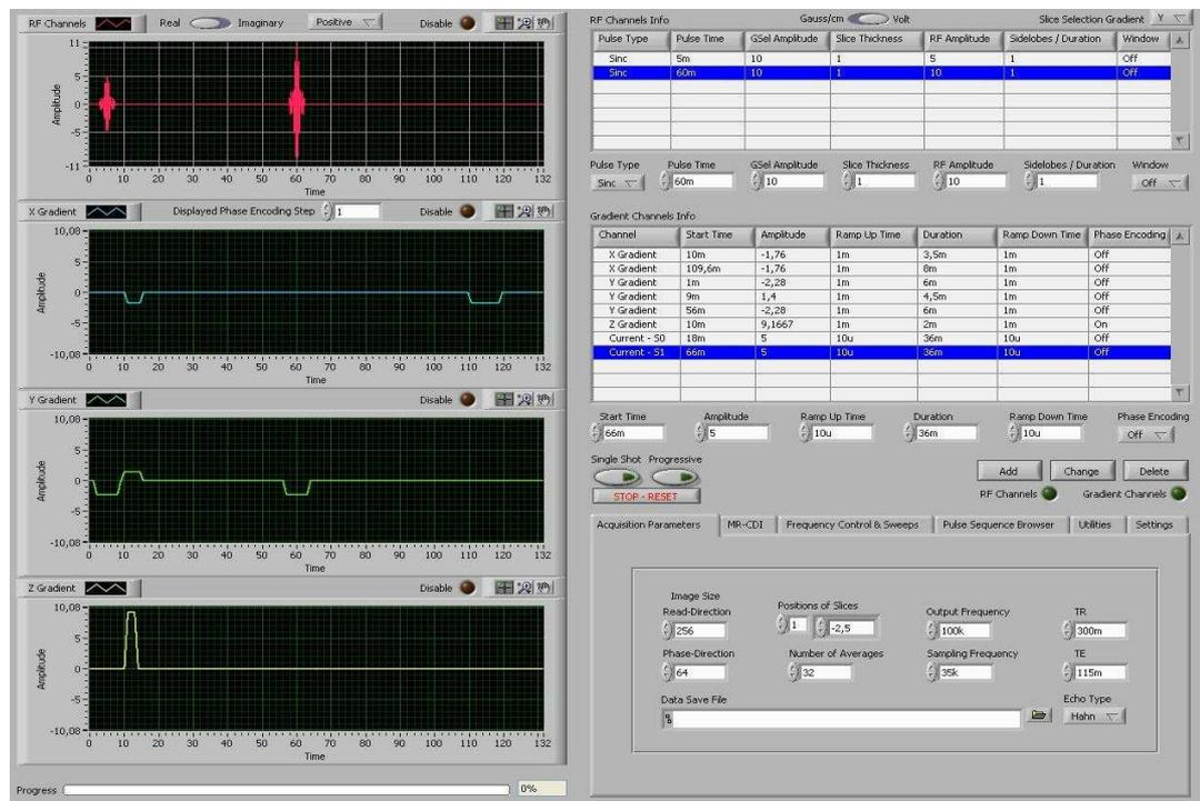
Figure A.11 Screen Shot Image of MRI software for  $B_y$  imaging
