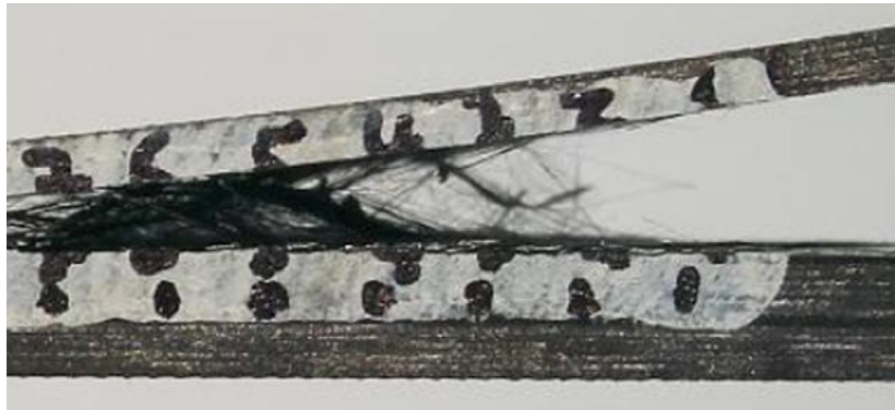
Figure 17: Fiber bridging during DCB test [70].
