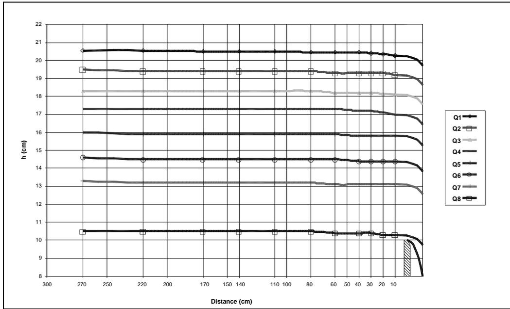
Figure 4.14 Water Surface for Different Discharges
