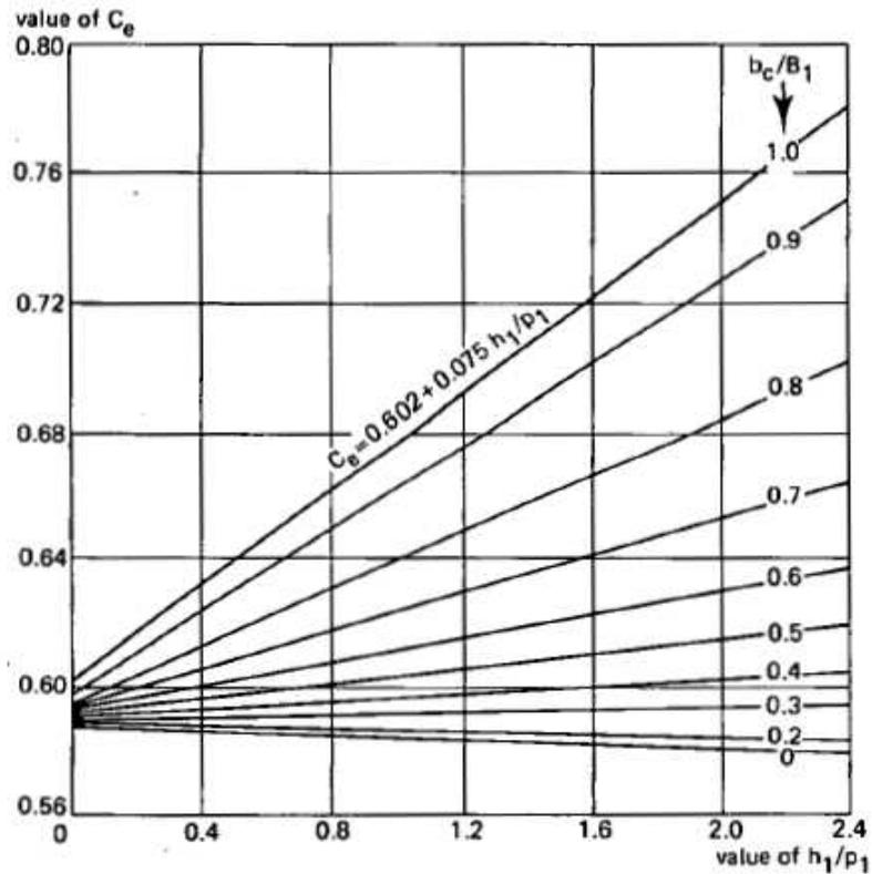
Figure 3.2 Graph of  $C_e$  versus  $h_1/P_1$  for values of  $b_c/B_1$
