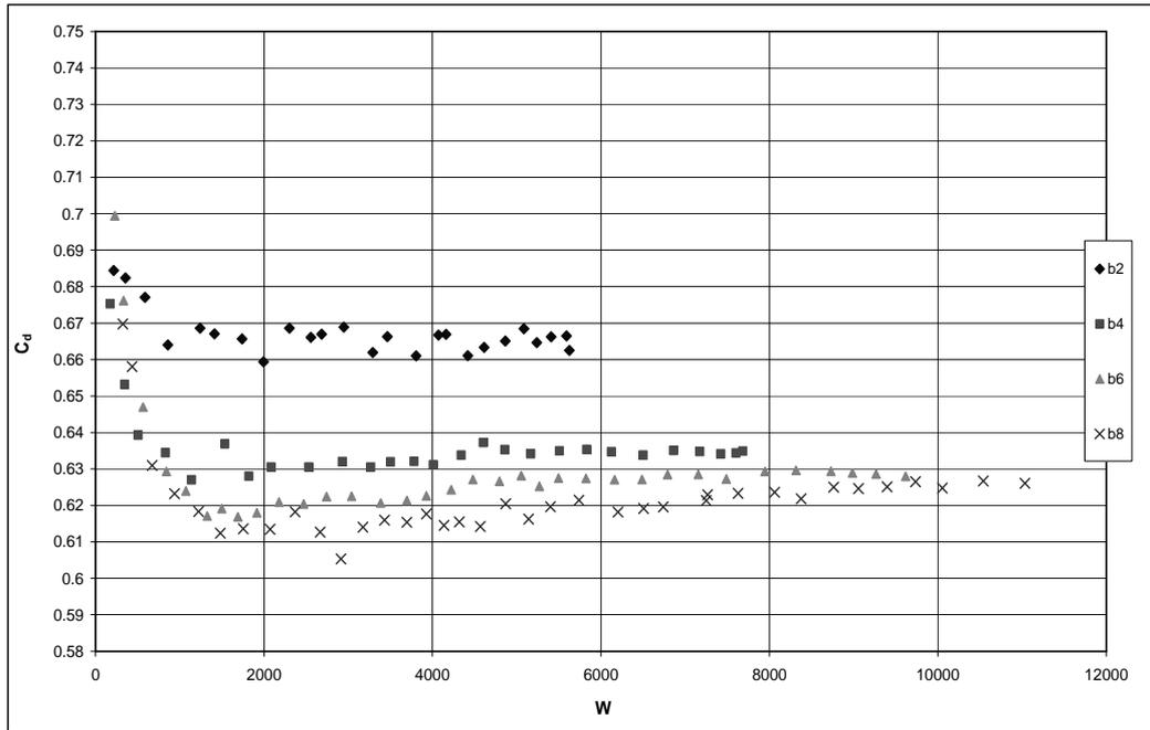
Figure 5.8  $C_d$  versus  $W$  for Slit Weir
