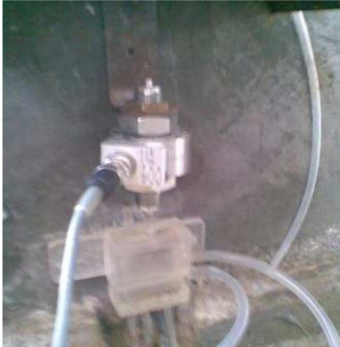
Figure 4.11 Pressure Transducer
