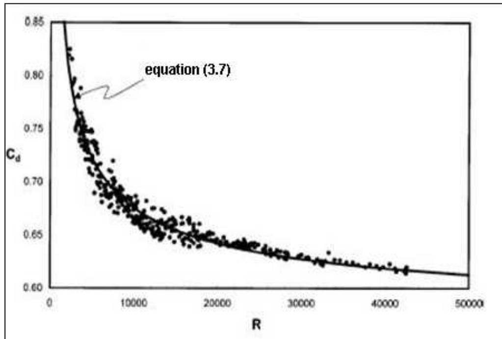
Figure 3.4 Graph of  $C_d$  versus  $R$  with both data points and equation line (Aydın et al., 2002)
