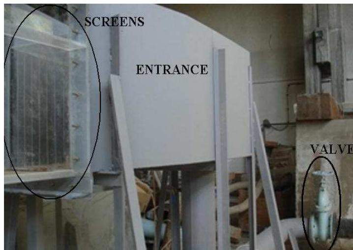
Figure 4.3 Valve and Entrance Structure
