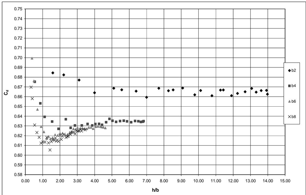
Figure 5.6  $C_d$  versus  $h/b$  for Slit Weir
