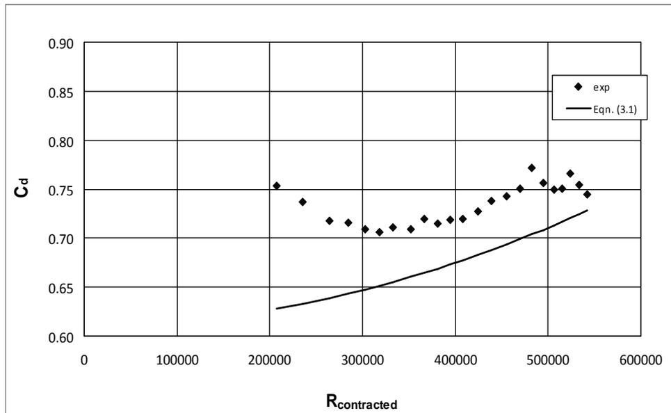
Figure 5.13 Comparison of Contracted Weir Data with Eqn. (3.1)
