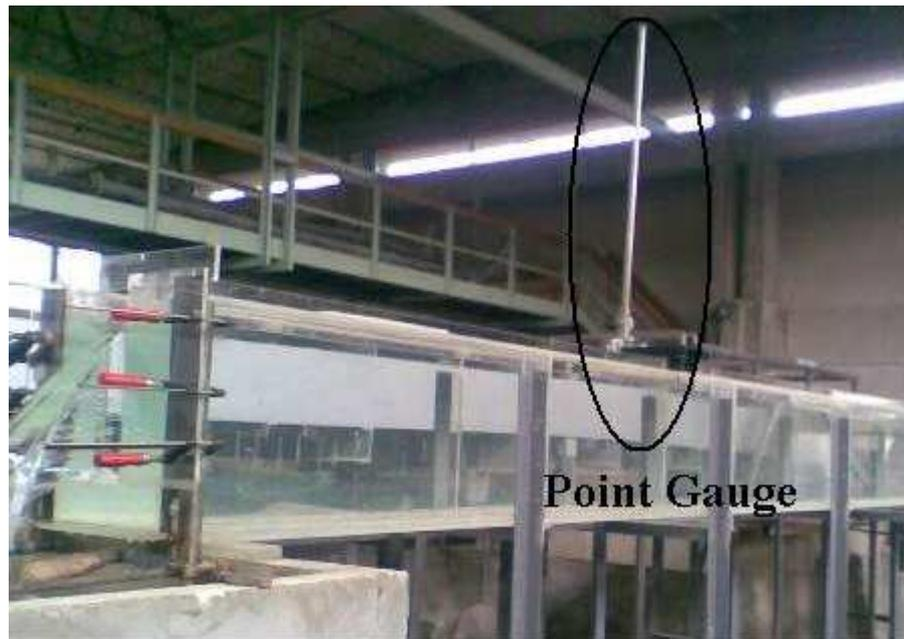
Figure 4.6 Location of Point Gauge on the Channel
