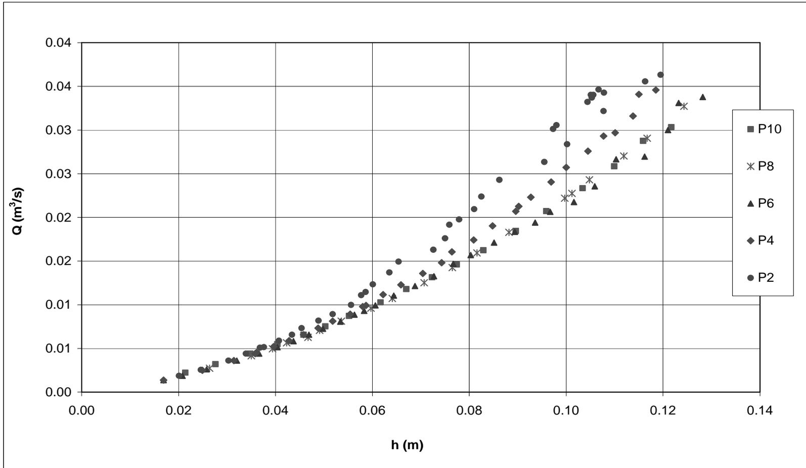
Figure 5.1 Relationship Between Discharge ( $Q$ ) and Head on the Weir ( $h$ ) for All Collected Data of Different Weir Heights
