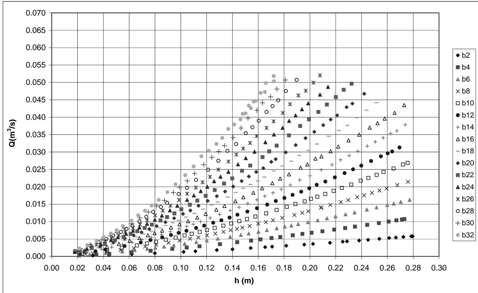
Figure 5.3 Relationship Between Discharge ( $Q$ ) and Head on the Weir ( $h$ ) for Collected Data Excluding Outliers
