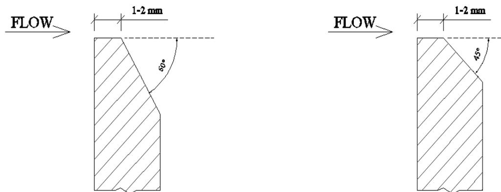
Figure 2.1 The Cross-section Details of Sharp Crested Weirs
