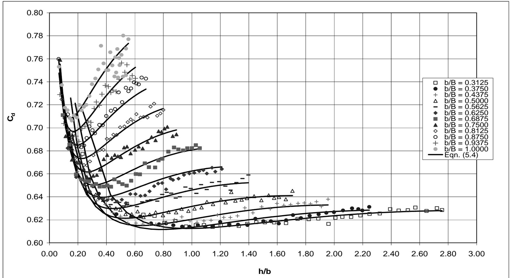
Figure 5.21  $C_d$  and  $h/b$  Relation for Comparison of Measured Data with Those Calculated by Eqn. (5.4)
