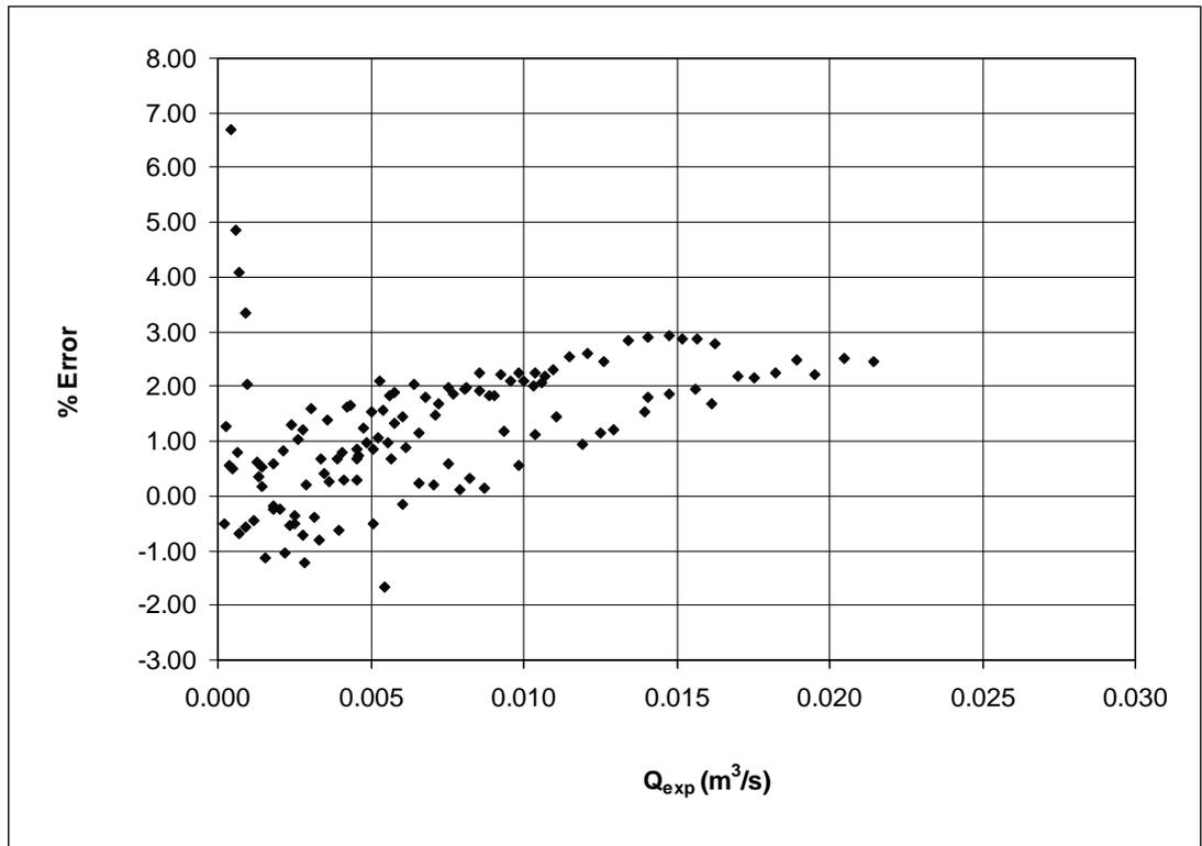
Figure 5.10 Percent Error with respect to Experimental Discharge
