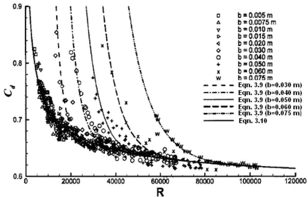
Figure 3.5 Graph of  $C_d$  versus  $R$  for different weir openings ( $b$ ) with both data points and equation lines (Aydın et al., 2006)
