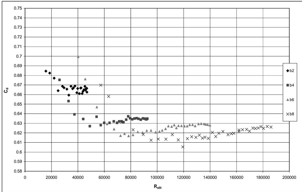
Figure 5.7  $C_d$  versus  $R_{slit}$  for Slit Weir
