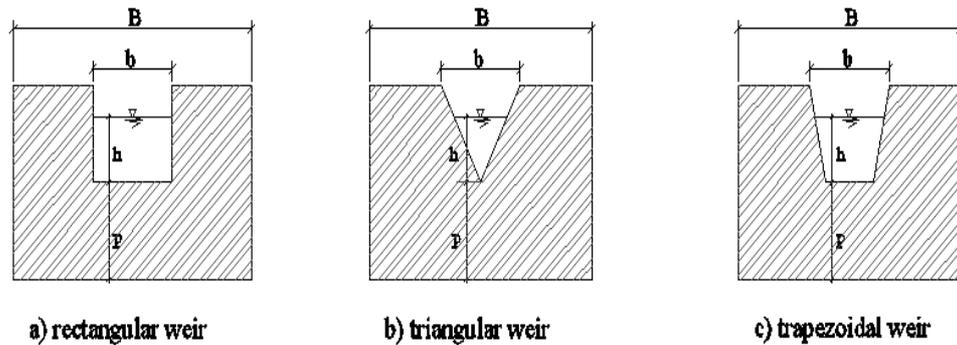
Figure 2.3. Types of Sharp Crested Weirs
