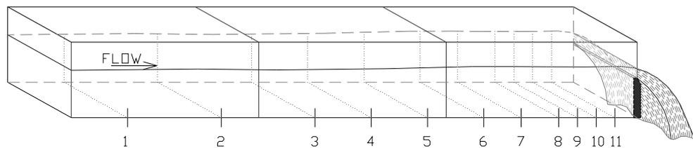
Figure 4.13 Sections where Water Depths are Measured in Channel
