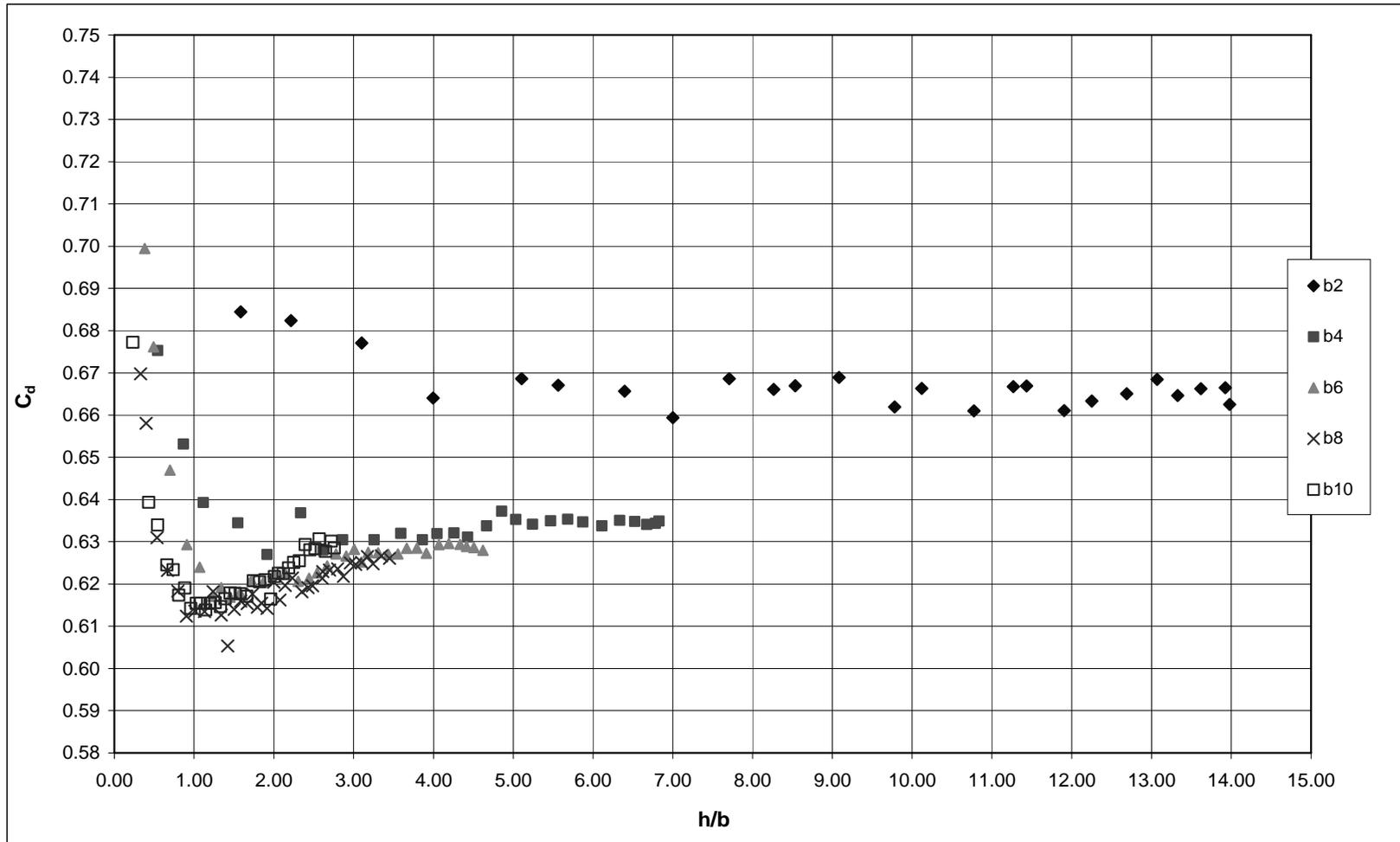
Figure 5.5 Difference between Slit and Contracted Weir
