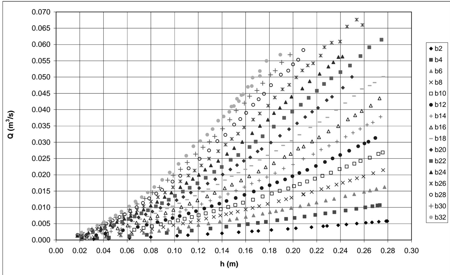
Figure 5.2 Relationship Between Discharge ( $Q$ ) and Head on the Weir ( $h$ ) for All Collected Data
