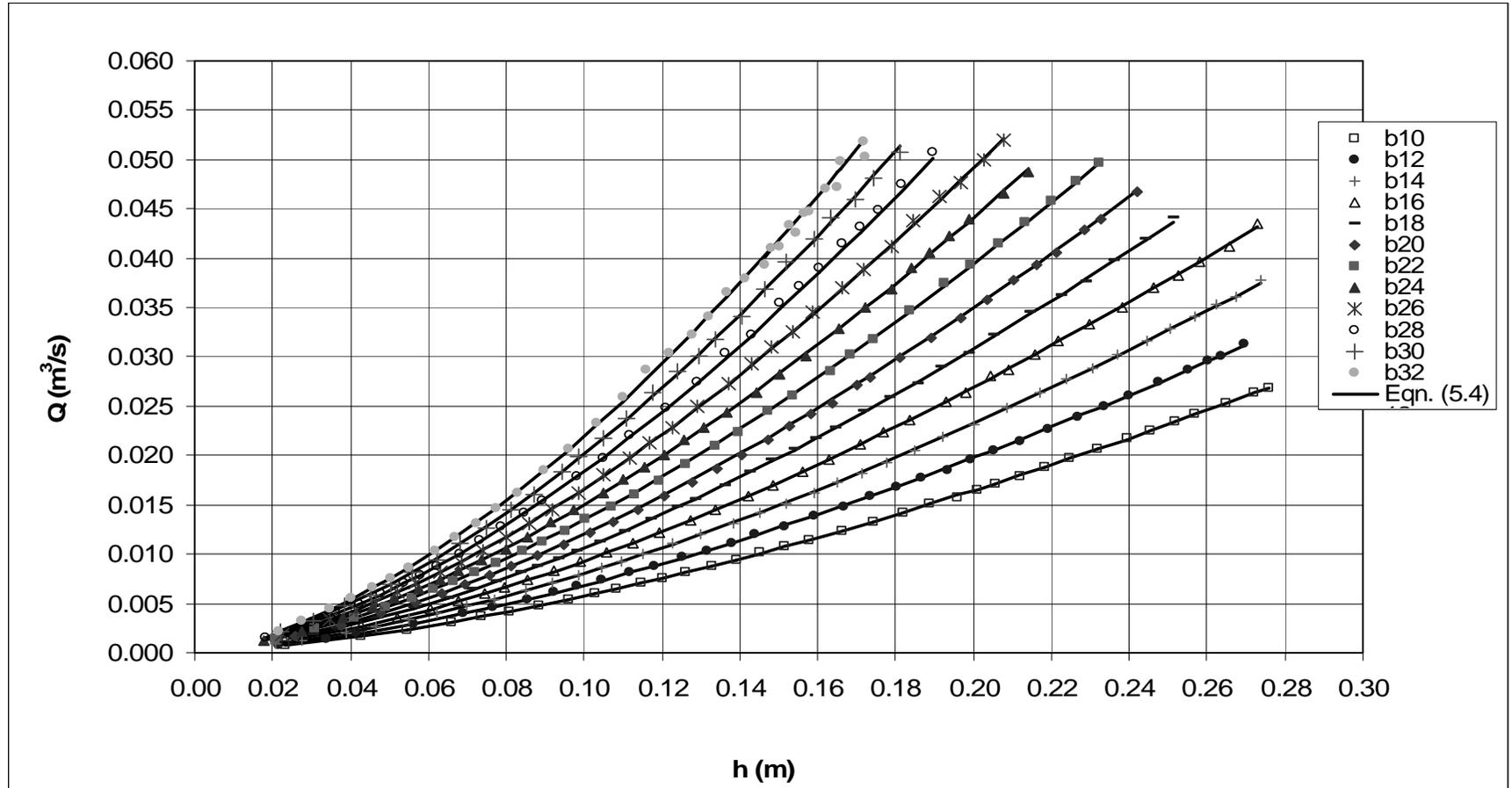
Figure 5.20  $Q$  and  $h$  Relation for Comparison of Measured with Eqn. (5.4)
