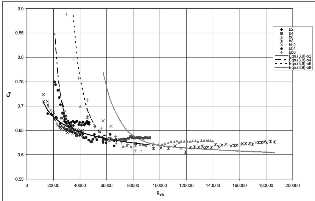
Figure 5.11 Comparison of New Experimental Data, Old Experimental Data (Aydın et al. (2006)) and Slit Weir Equation (Eqn. (3.9))
