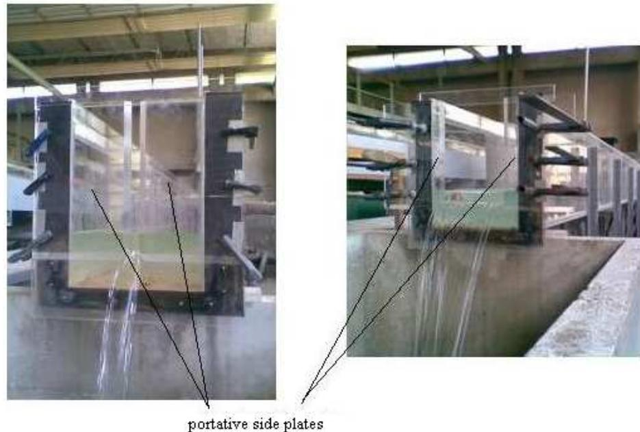
Figure 4.8 Side Plates of Weir for Different Weir Openings
