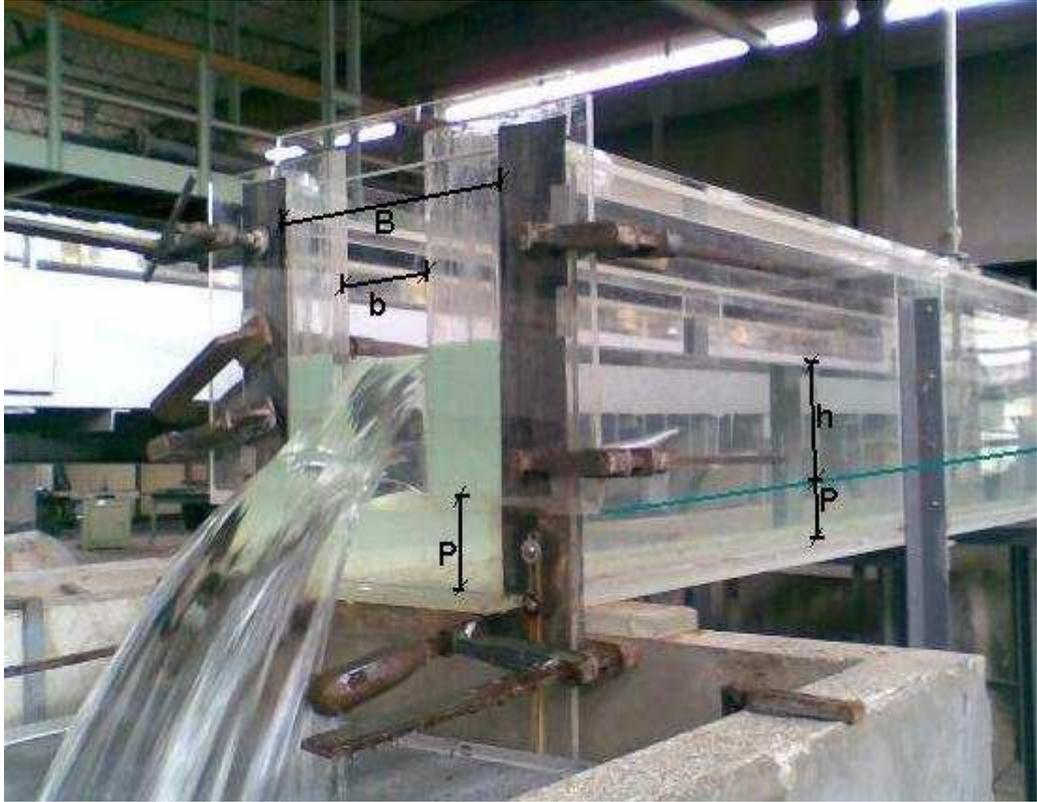
Figure 2.2. The Parameters of Sharp Crested Rectangular Weirs
