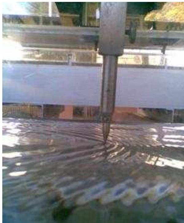
Figure 4.7 Closer View of Point Gauge
