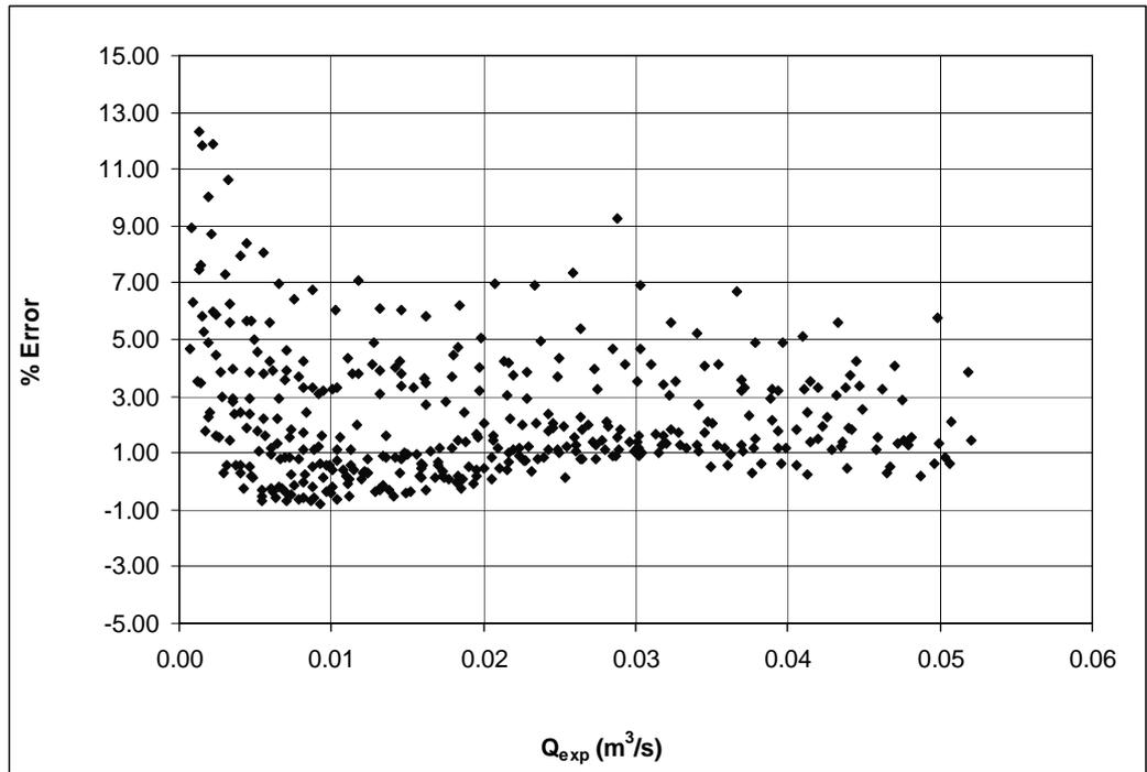
Figure 5.16 Percent Error with respect to Experimental Discharge and Eqn. (3.3)
