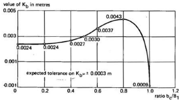
Figure 3.1 The value of  $K_b$  with respect to  $b_c/B_1$  (Bos, 1989)
