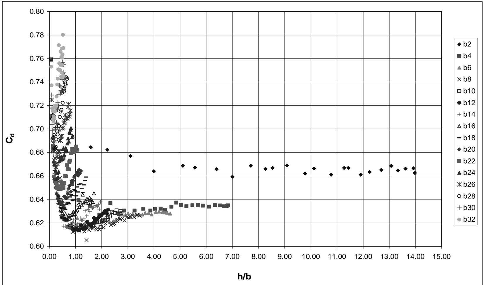
Figure 5.4  $C_d$  versus  $h/b$  for All Width Openings
