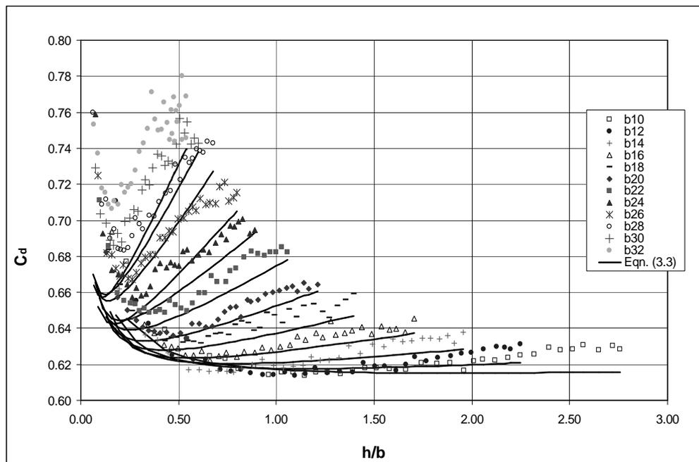
Figure 5.15 Comparison of Contracted Weir Data with Eqn. (3.3)
