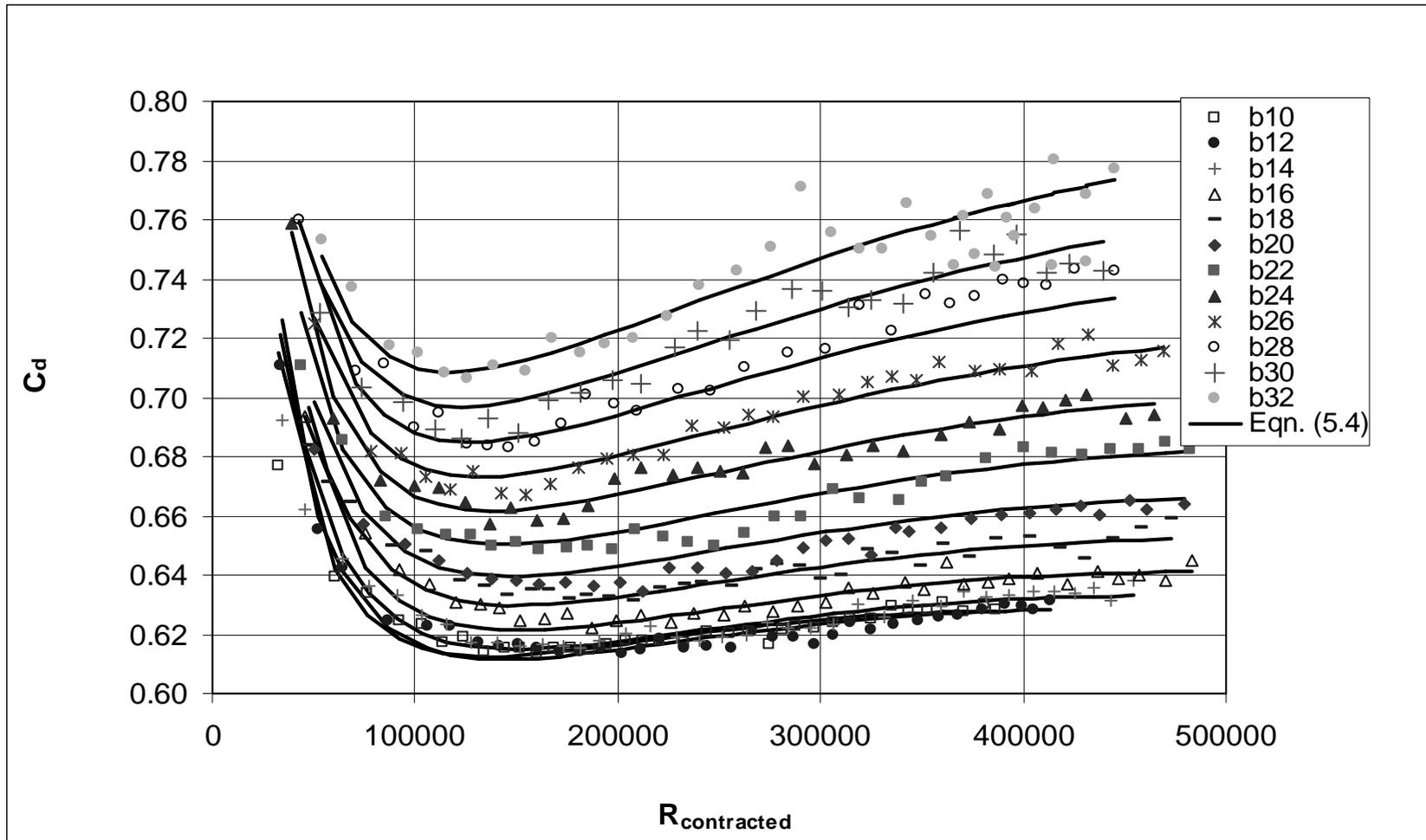
Figure 5.22  $C_d$  and  $R_{contracted}$  Relation for Comparison of Measured Data with Those Calculated by Eqn. (5.4)
