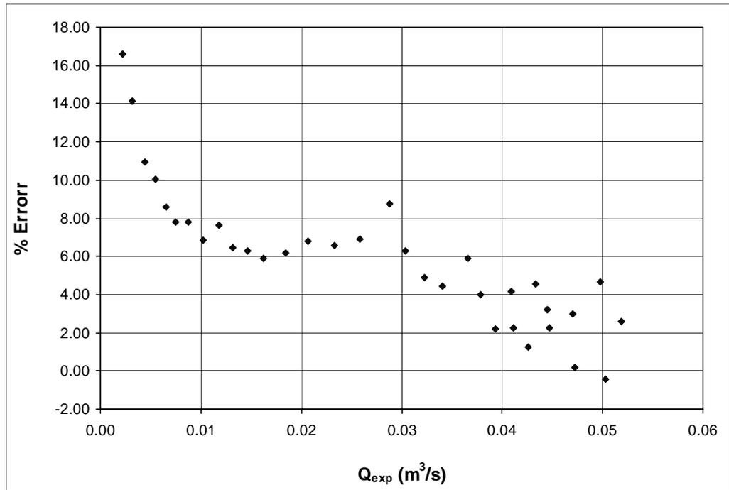
Figure 5.14 Percent Error with respect to Experimental Discharge and Eqn. (3.1)
