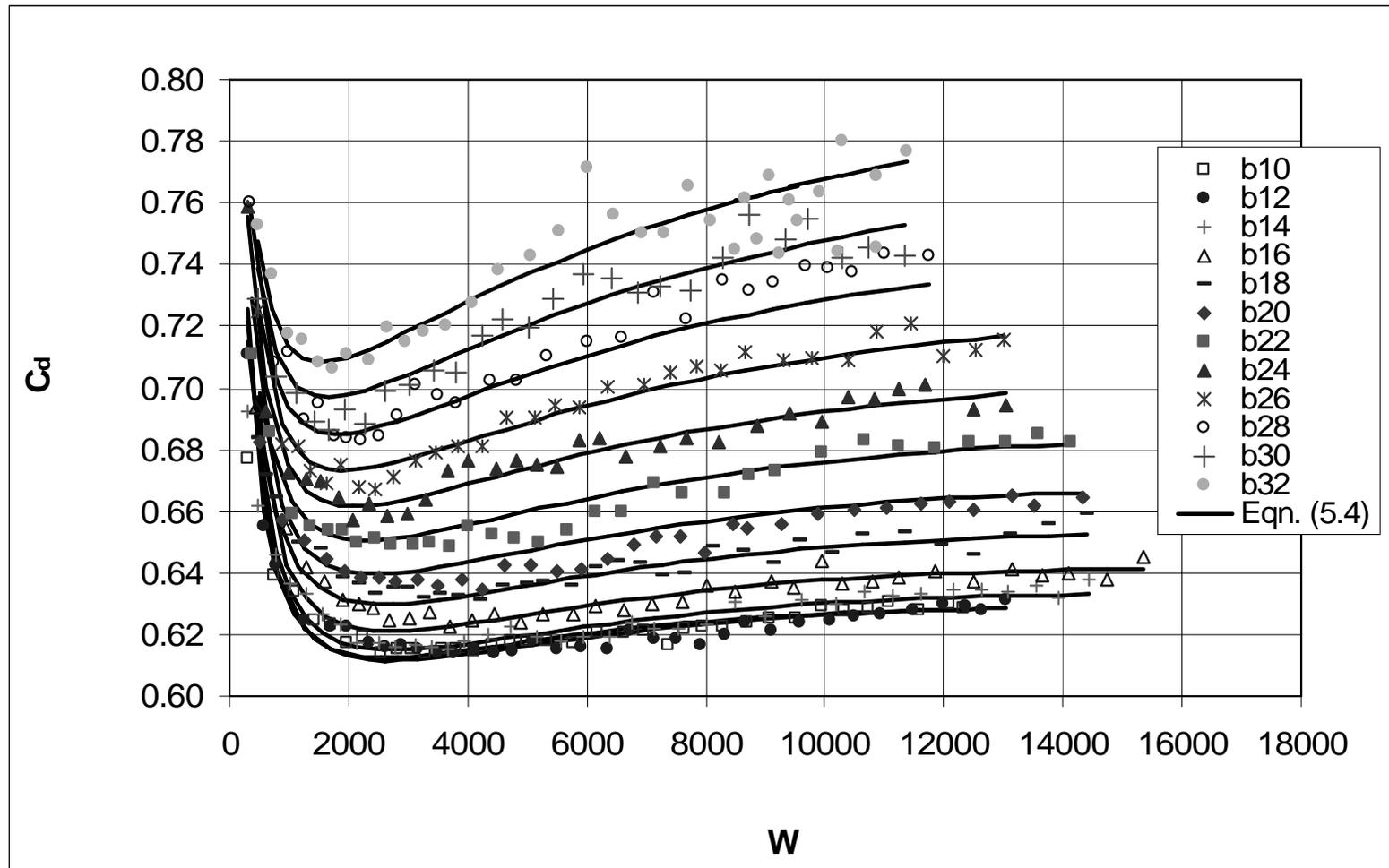
Figure 5.23  $C_d$  and  $W$  Relation for Comparison of Measured Data with Those Calculated by Eqn. (5.4)
