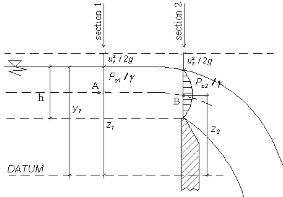
Figure 2.6 Schematic View of Flow Over Weir
