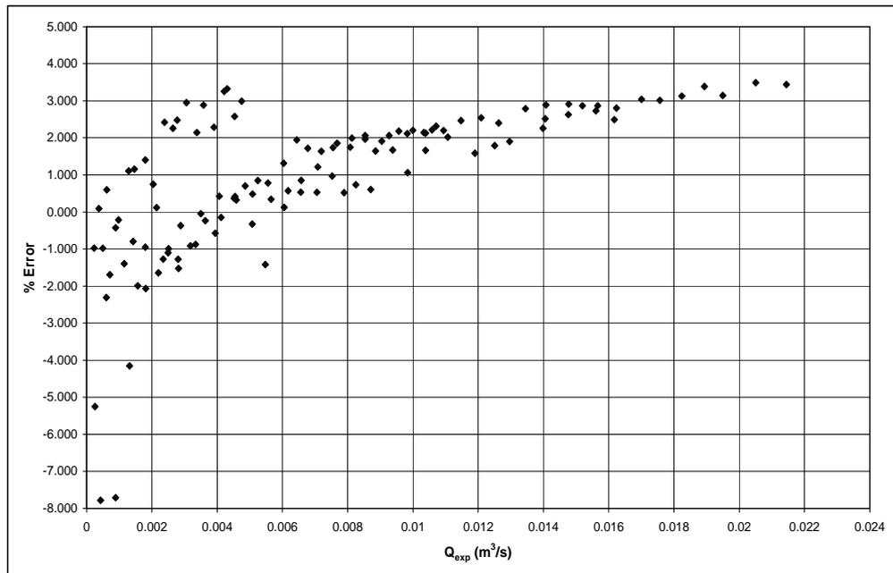
Figure 5.12 Percent Error with respect to Experimental Discharge and Eqn. (3.6)
