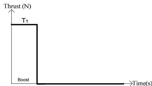
Figure 2.4 Single phase rocket: Boost
