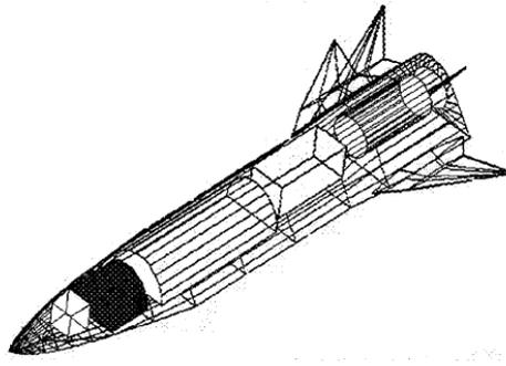
Figure 1.3 Typical Wireframe Geometry Model with Packages
