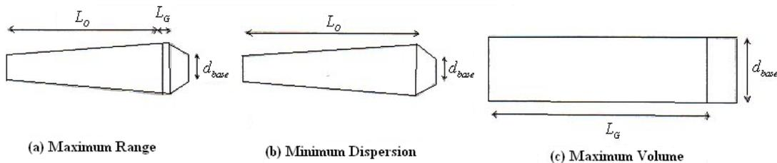
Figure 1.6 Single Objective Optimum Configurations for Artillery Shell
