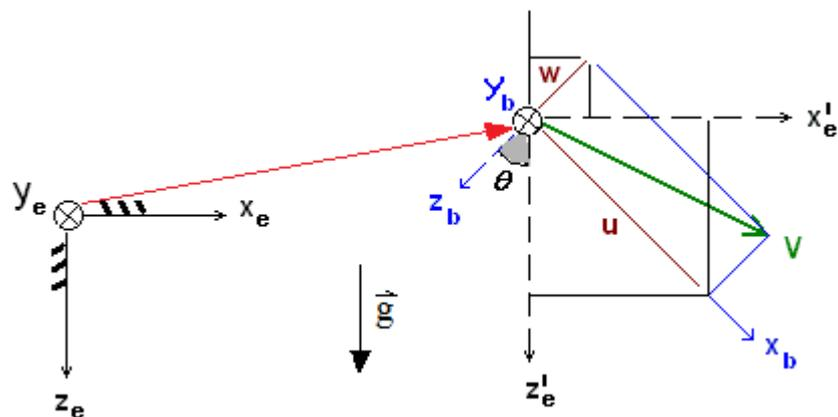
Figure 2.2 Velocity Vector in the Earth and Body Frames
