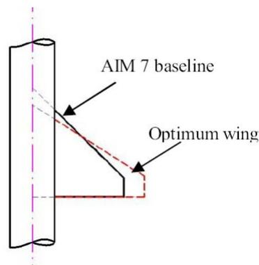
Figure 1.5 Optimum AIM Wing Configuration [13]
