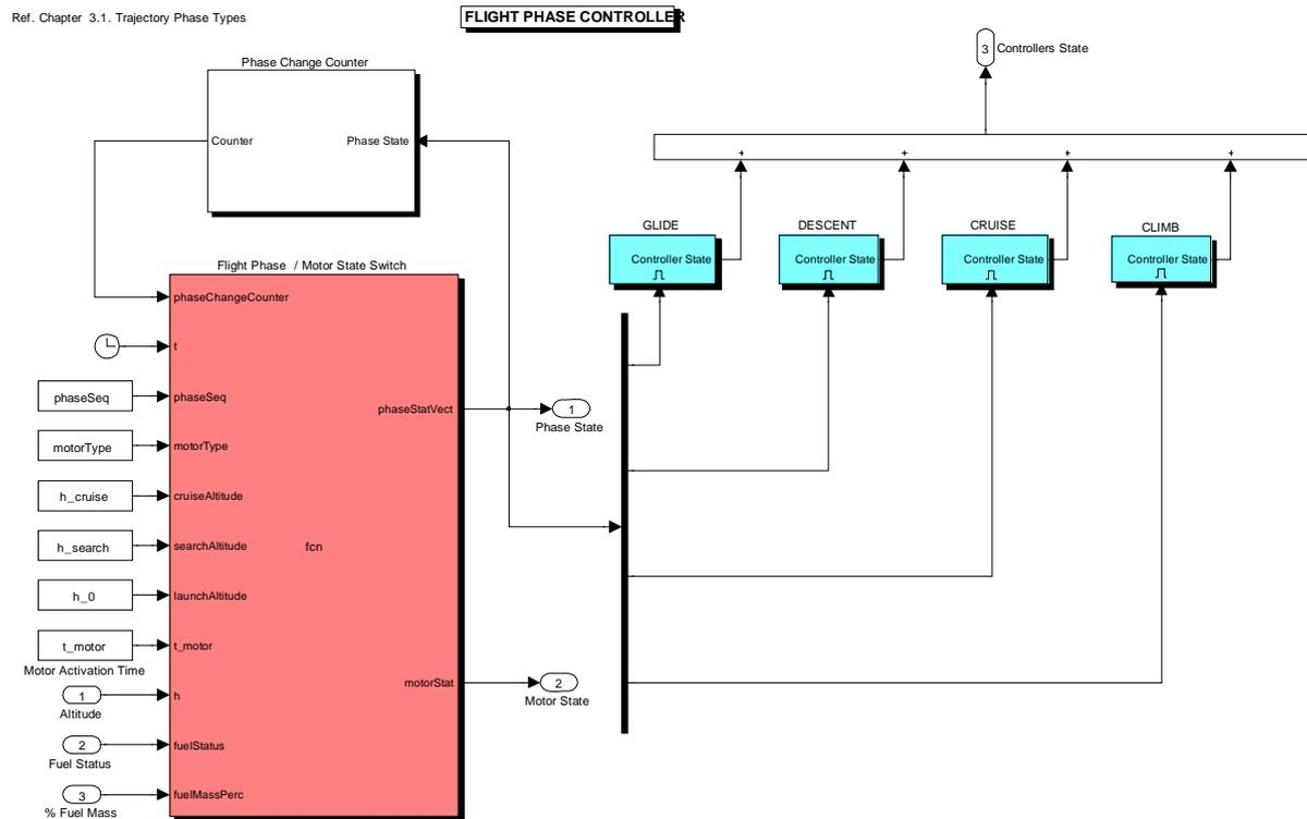
Figure B. 6 Simulink Block Diagram of Flight Phase Controller
