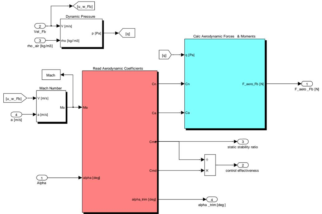
Figure B. 2 Simulink Block Diagram of Aerodynamic Model
