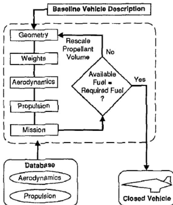
Figure 1.8 Automated Vehicle Closure Process
