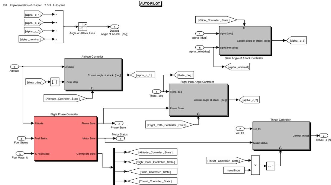
Figure B. 5 Simulink Block Diagram of Autopilot
