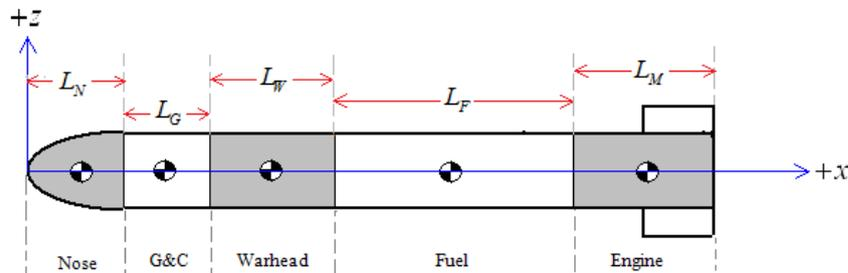
Figure 4.5 Components and their Lengths of a Missile
