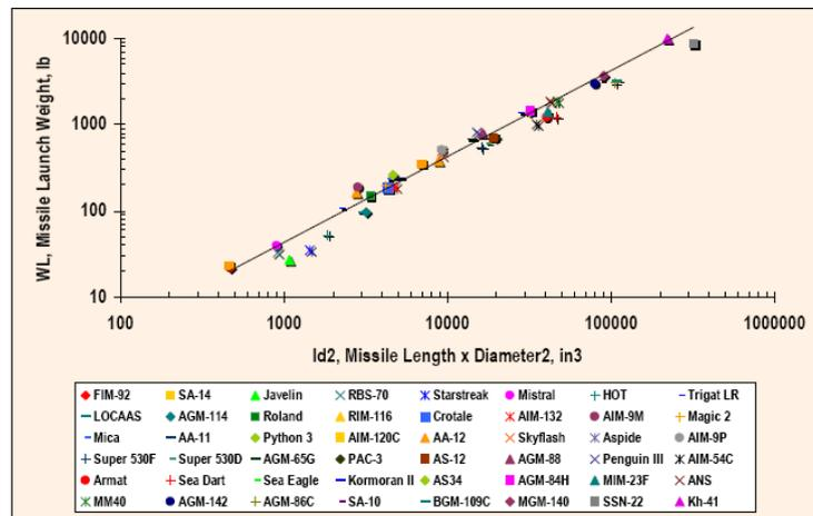
Figure 4.4 Missile mass is a function of diameter and length [8]
