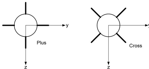
Figure 4.2 Types of Panel Orientations (Back view of missile)
