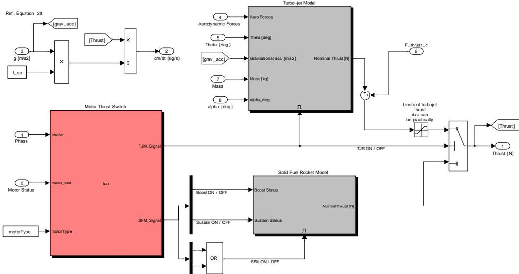
Figure B. 3 Simulink Block Diagram of Thrust Model
