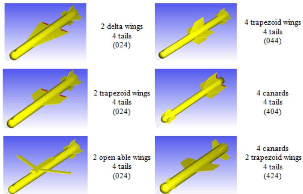
Figure 4.1 Some of the Fin Configuration Alternatives
