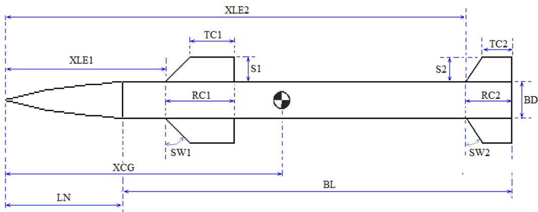
Figure 4.3 External Geometric Dimensions
