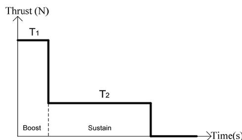
Figure 2.6 Two-phase rocket motor: Boost-Sustain
