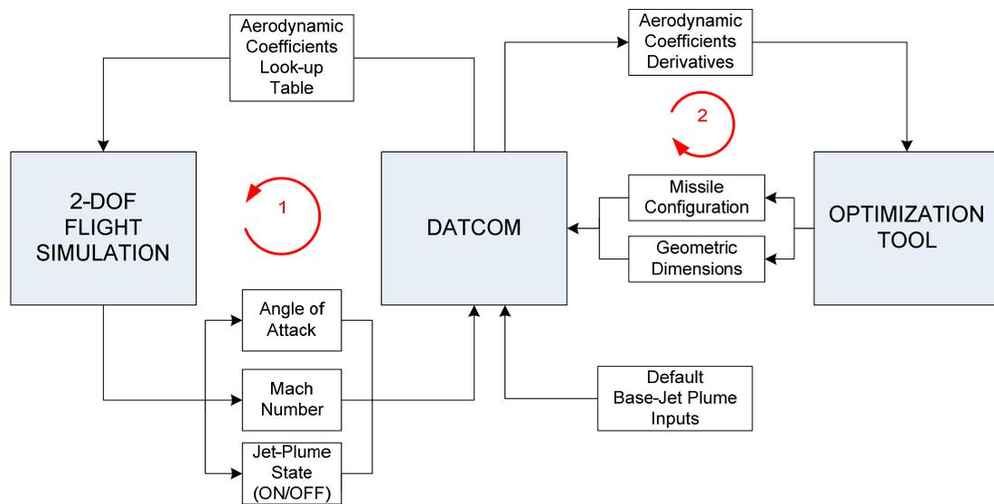
Figure 2.3 Aerodynamic Data Flow
