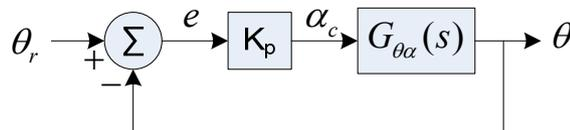
Figure 2.9 Proportional Flight Path Angle Control
