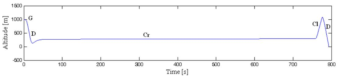
Figure 7.5 Altitude vs. Time Plot of the Baseline Missile in 2 DOF Simulation
