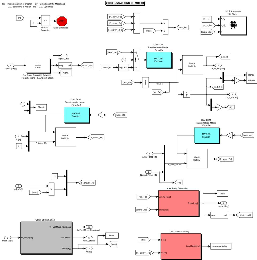
Figure B. 4 Simulink Block Diagram of EOM (Equations of Motion)
