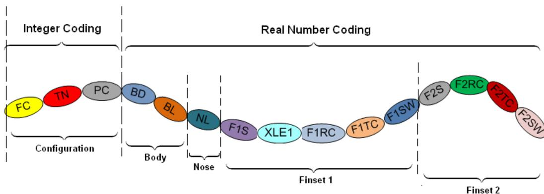
Figure 5.4 Chromosome Representing External Configuration and Geometric Dimensions of a Missile
