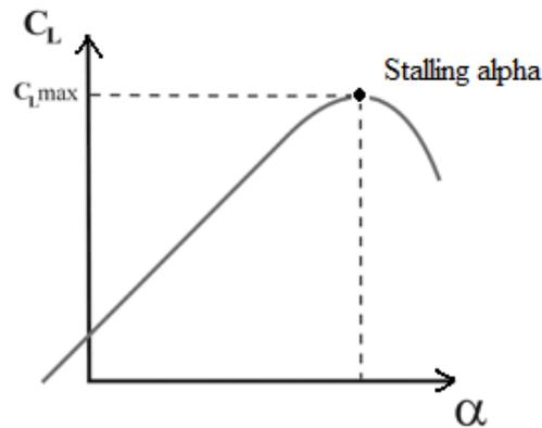
Figure 3.5 A Typical Lift Coefficient Curve
