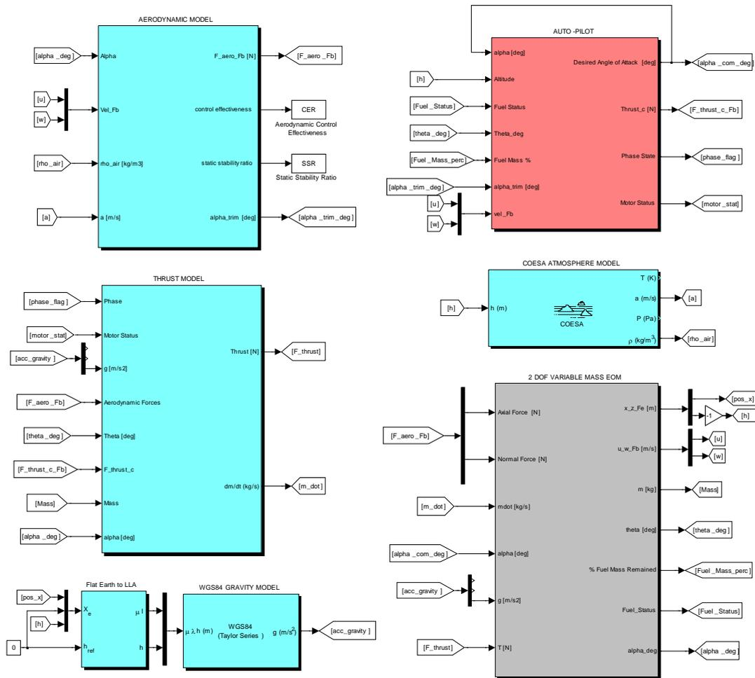
Figure B. 1 Simulink Block Diagram of Flight Simulator
