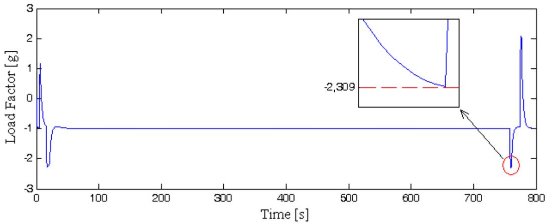
Figure 7.6 Load Factor of Baseline Missile in Pull-up Maneuver
