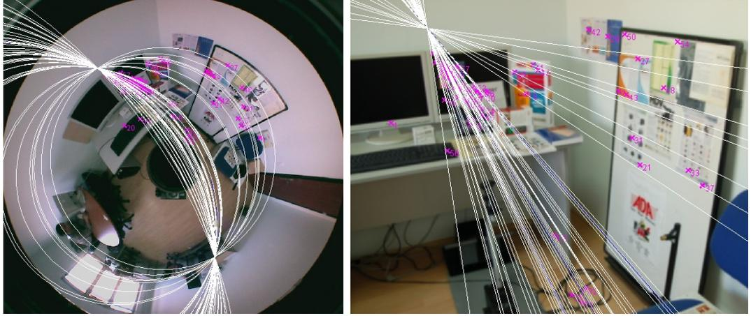
Figure 5.2: Example catadioptric-perspective pair and epipolar conics/lines of point correspondences.
