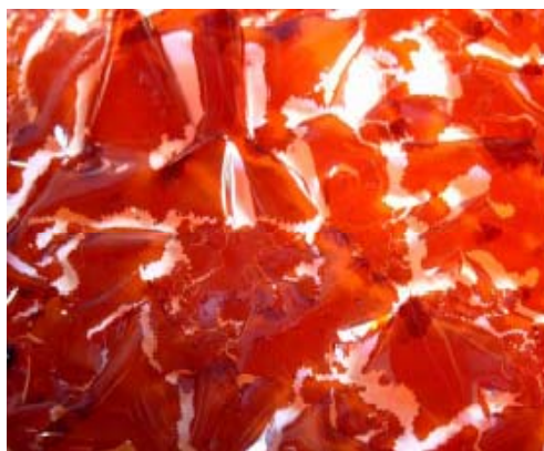
Figure 4. 4 PBI membrane that is cast from the polymer with a molecular weight of < 18000
