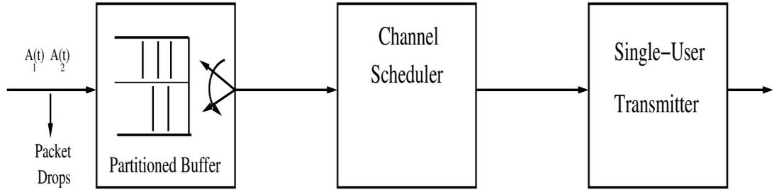
**Figure 5.4:** The model for two user joint buffer management and user scheduling in a time-varying channel
