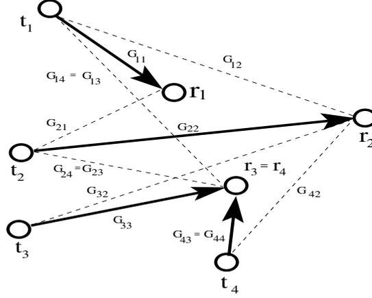
Figure 4.1: The ad-hoc wireless network model: A set of interfering links
