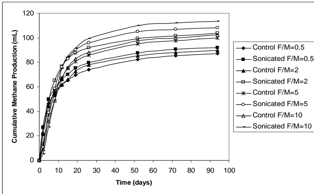
Figure 4.27. The daily change in cumulative methane gas production of 250 mL reactors at different F/M ratios during anaerobic digestion
