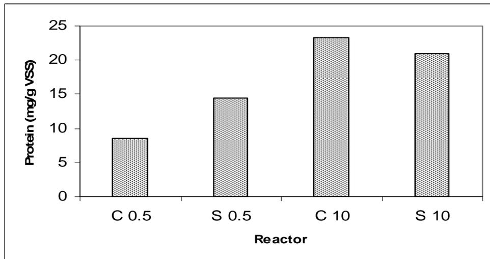
Figure 4.44. Protein content of 3 L reactors at different F/M ratios after digestion
