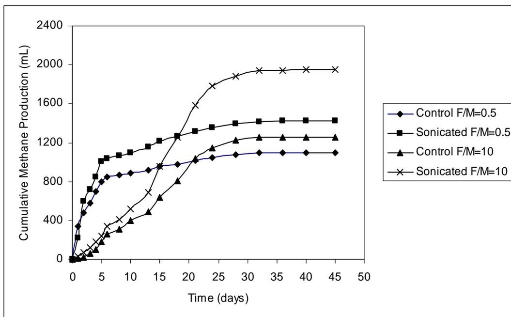
Figure 4.39. The daily change in cumulative methane gas production of 3 L reactors at different F/M ratios during anaerobic digestion
