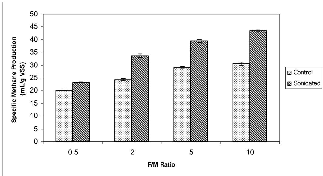
Figure 4.29. Methane gas amount of 250 mL reactors at different F/M ratios as per gram VSS after anaerobic digestion
