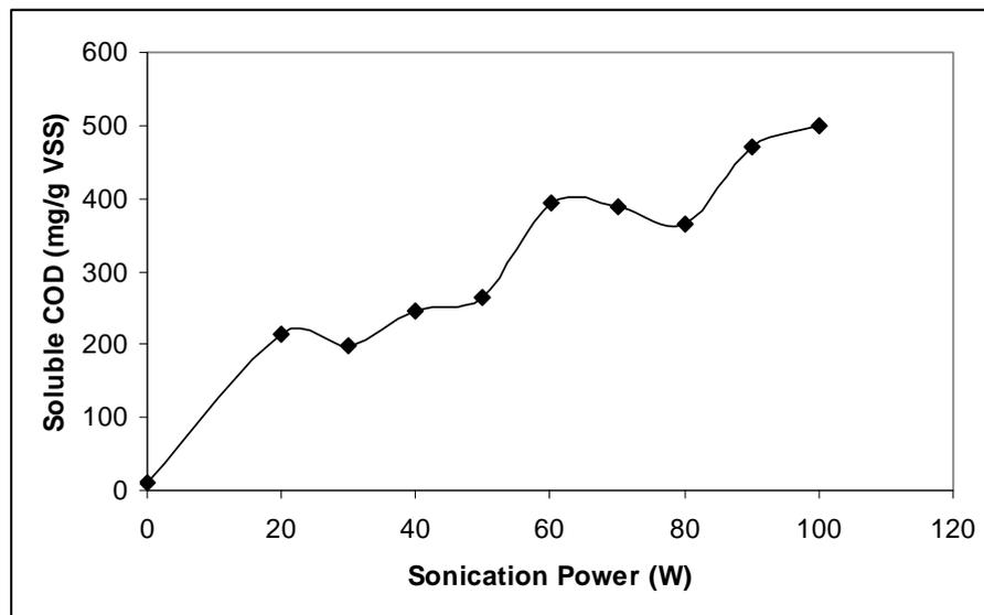
Figure 4.1. The variation in soluble COD according to sonication power (without temperature control)
