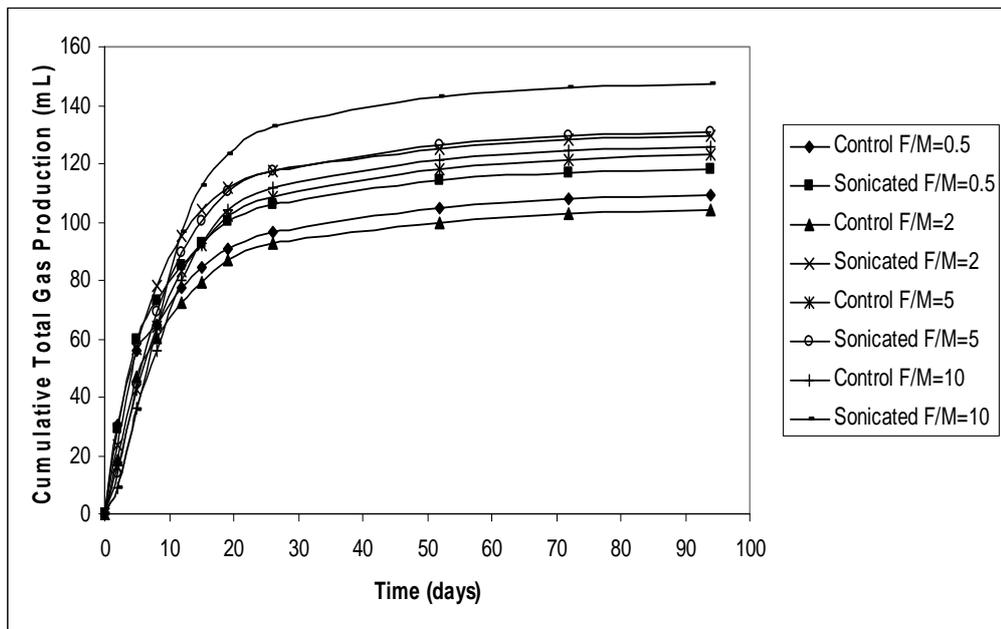
Figure 4.26. The daily change in cumulative total gas production of 250 mL reactors at different F/M ratios during anaerobic digestion
