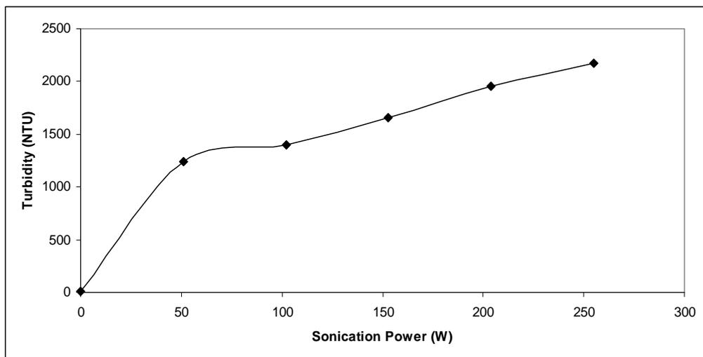
Figure 4.18. The variation in turbidity according to sonication power (using 22 mm probe)
