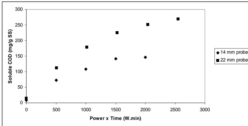
Figure 4.22. The comparison of probes as soluble COD according to sonication power x time
