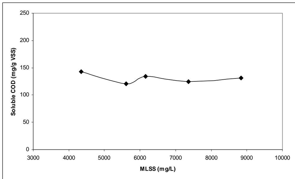
Figure 4.13. Change in normalized soluble COD with respect to MLSS concentration of sludge
