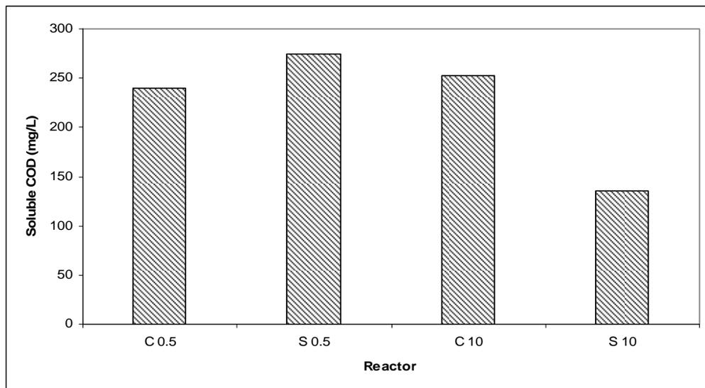
Figure 4.41. Soluble COD of 3 L reactors at different F/M ratios after digestion
