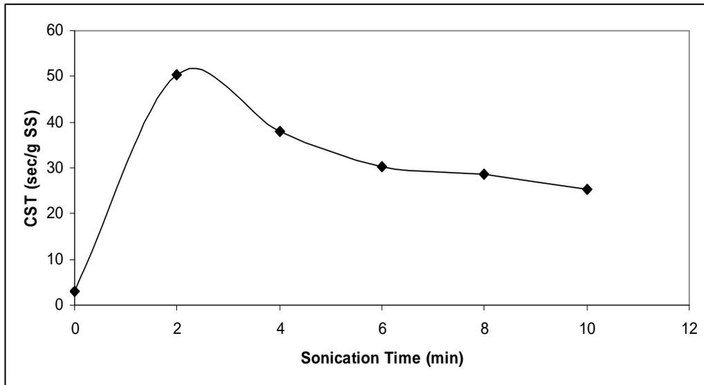
Figure 4.20. The variation in CST according to sonication time (using 22 mm probe)
