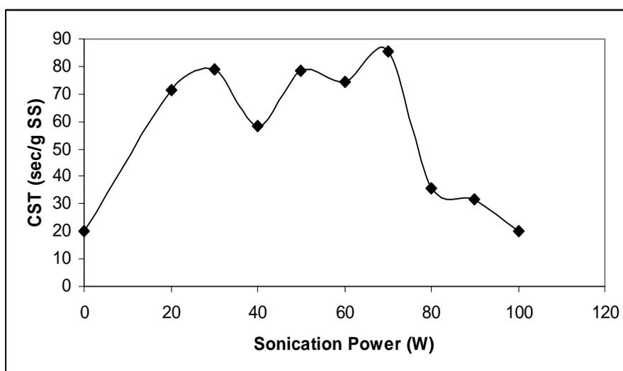
Figure 4.2. The variation in CST according to sonication power (without temperature control)
