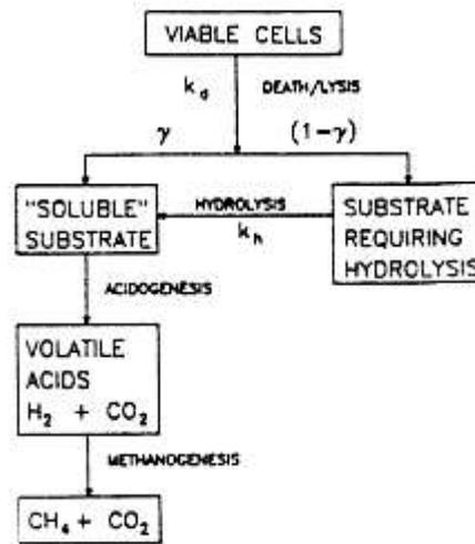
Figure 4.48. Anaerobic digestion model for biological solids (Pavlostathis and Gossett, 1986)
