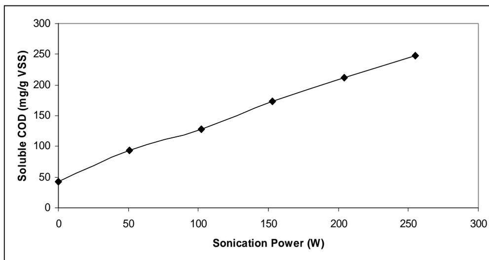
Figure 4.16. The variation in soluble COD according to sonication power (using 22 mm probe)
