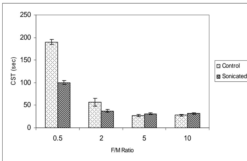
Figure 4.36. CST values of 250 mL reactors at different F/M ratios after digestion
