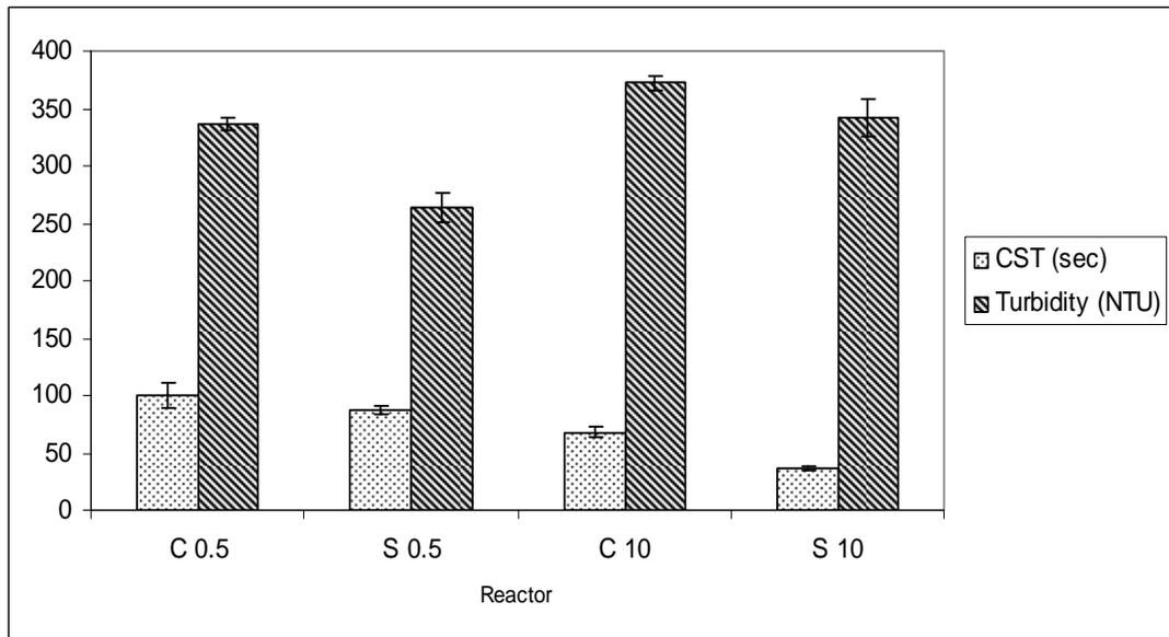
Figure 4.40. CST and turbidity values of 3 L reactors at different F/M ratios after digestion
