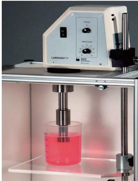
Figure 3.1. Ultrasonic homogenizer
