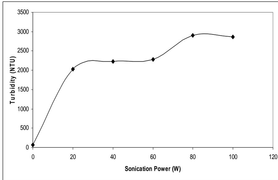
Figure 4.7. The variation in turbidity according to sonication power (using 14 mm probe)
