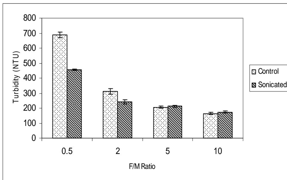
Figure 4.37. Turbidity values of 250 mL reactors at different F/M ratios after digestion
