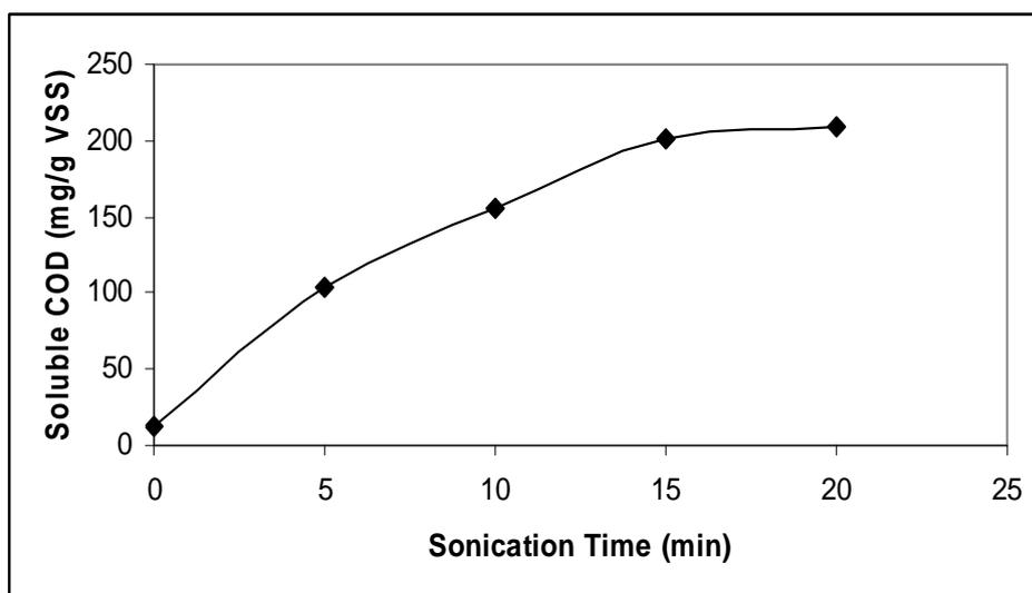
Figure 4.8. The variation in soluble COD according to sonication time (using 14 mm probe)
