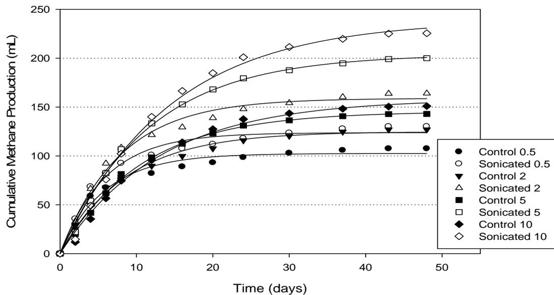
Figure C.2. Representation of non-linear regression analysis of methane gas productions of 250 mL unsonicated and high power-sonicated reactors
