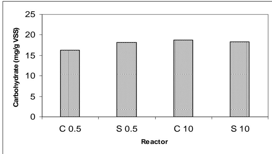
Figure 4.43. Carbohydrate content of 3 L reactors at different F/M ratios after digestion
