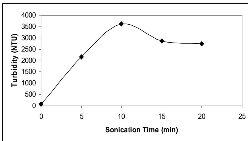
Figure 4.10. The variation in turbidity according to sonication time (using 14 mm probe)
