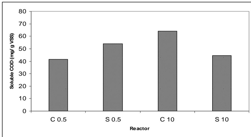
Figure 4.42. Normalized soluble COD of 3 L reactors at different F/M ratios after digestion
