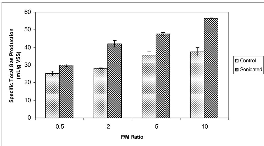
Figure 4.28. Total gas amount of 250 mL reactors at different F/M ratios as per gram VSS after anaerobic digestion
