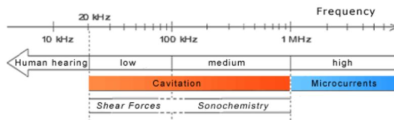
Figure 2.2. The sonication frequency interval (Ultrawaves, 2008)
