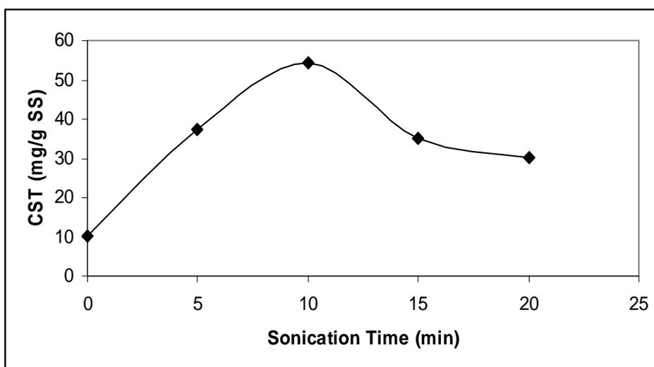
Figure 4.9. The variation in CST according to sonication time (using 14 mm probe)
