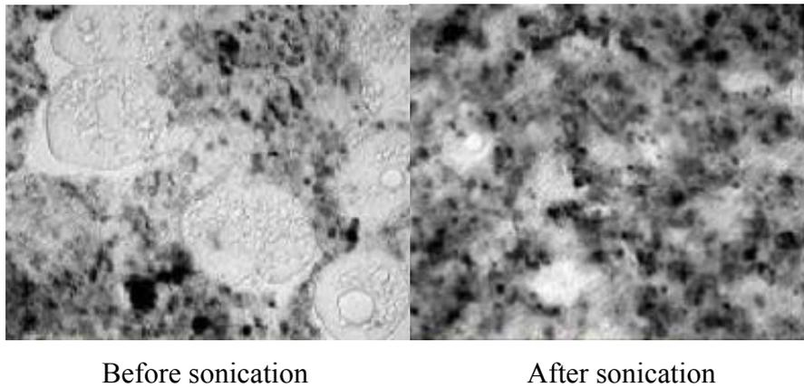
Figure 2.3. The microscopic picture of sludge before and after sonication (VoR, 2008)
