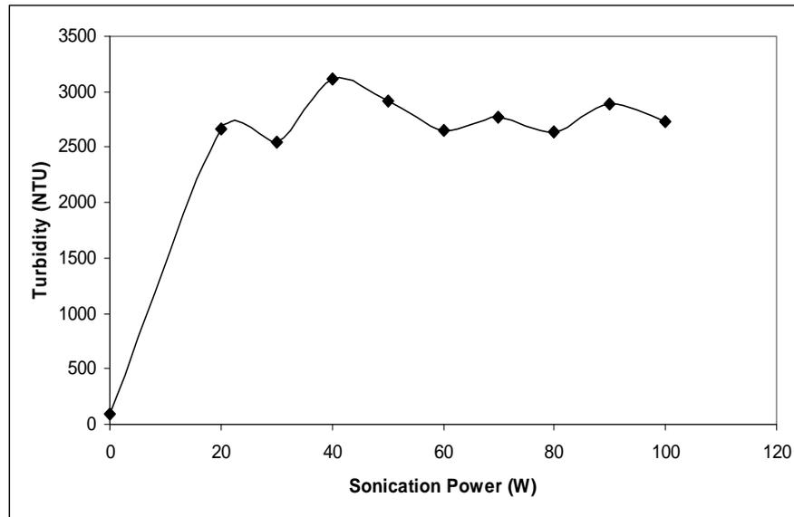
Figure 4.3. The variation in turbidity according to sonication power (without temperature control)
