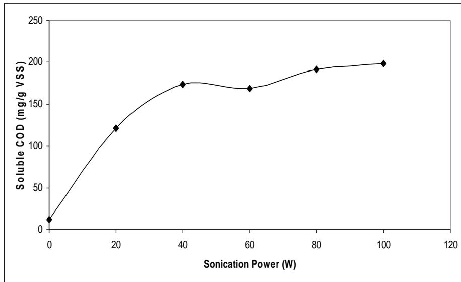
Figure 4.5. The variation in soluble COD according to sonication power (using 14 mm probe)
