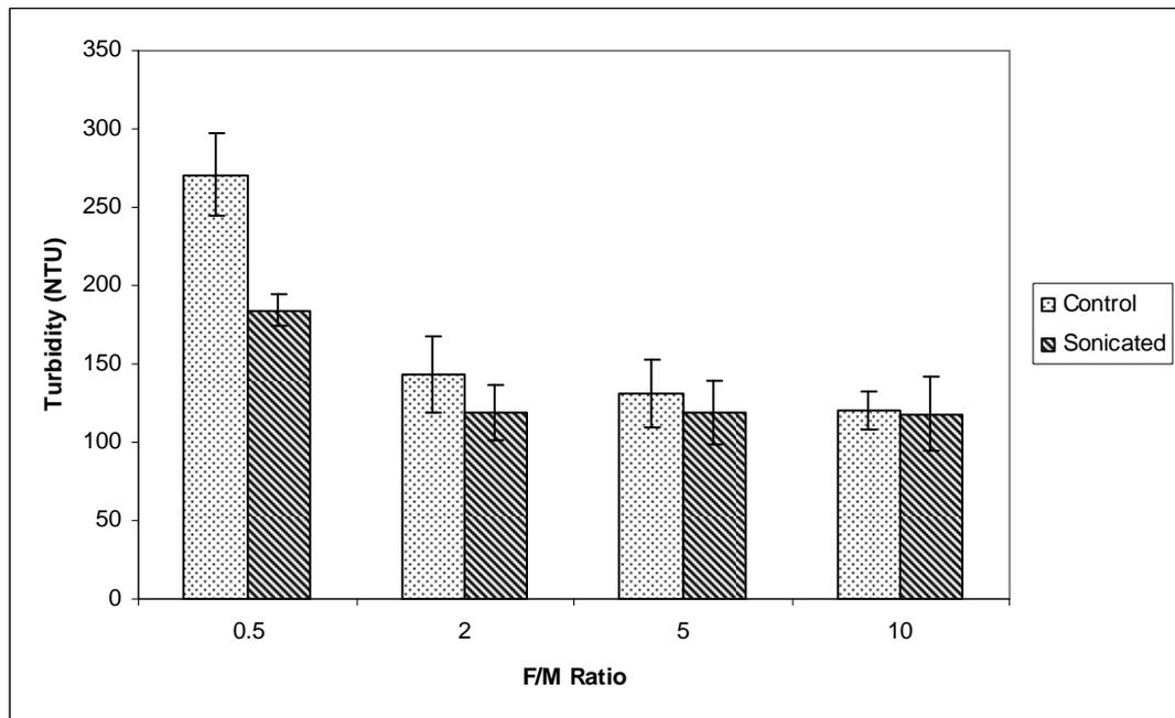
Figure 4.31. Turbidity values of 250 mL reactors at different F/M ratios after digestion
