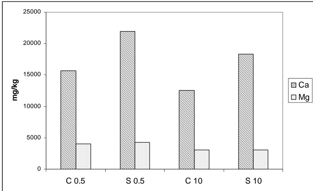
Figure 4.47. Calcium and magnesium concentration in 3 L reactors at different F/M ratios after digestion
