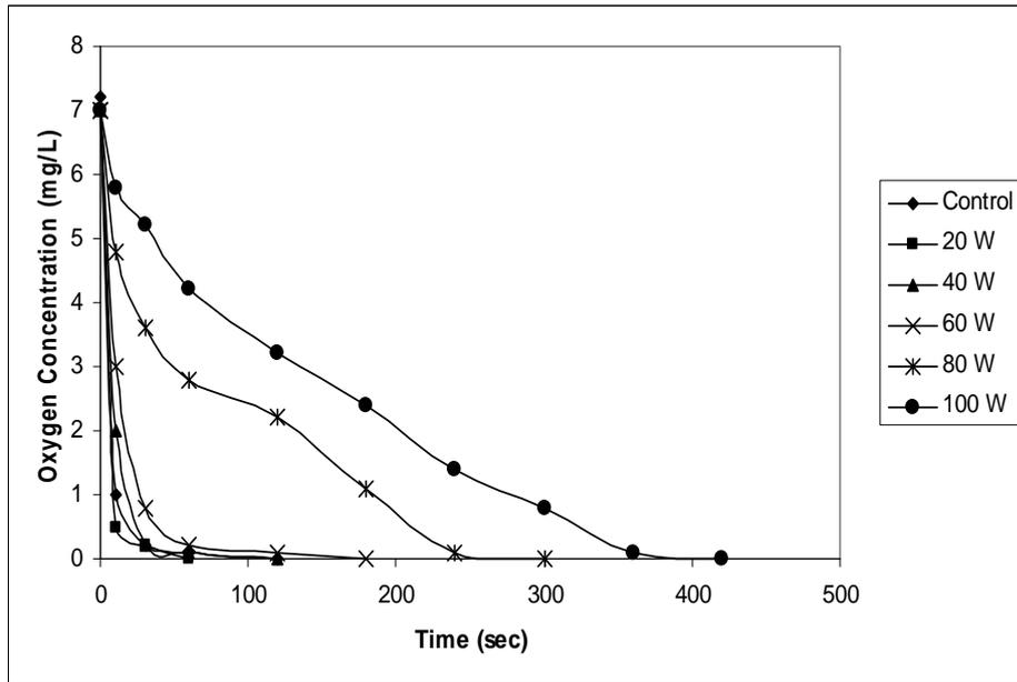
Figure 4.4. The variation in oxygen concentration according to sonication power
