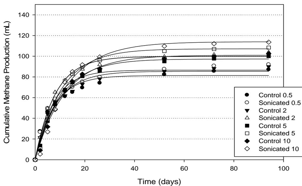
Figure C.1. Representation of non-linear regression analysis of methane gas productions of 250 mL unsonicated and low power-sonicated reactors
