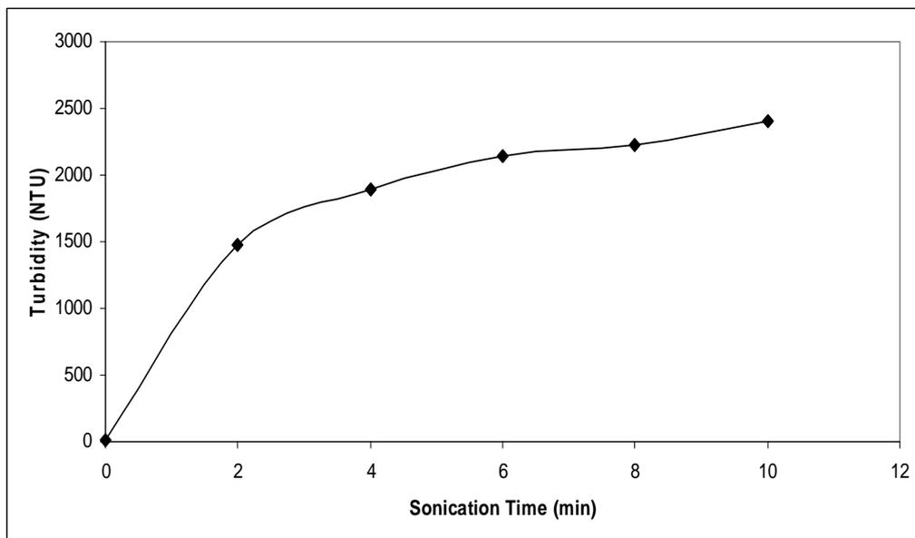
Figure 4.21. The variation in turbidity according to sonication time (using 22 mm probe)
