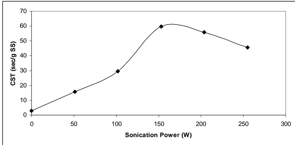
Figure 4.17. The variation in CST according to sonication power (using 22 mm probe)
