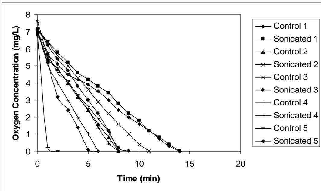
Figure 4.11. Oxygen concentration in sludges at different MLSS concentrations with respect to time
