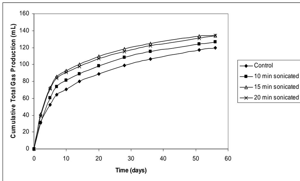
Figure 4.24. Cumulative total gas production of sludges sonicated at different times during anaerobic digestion
