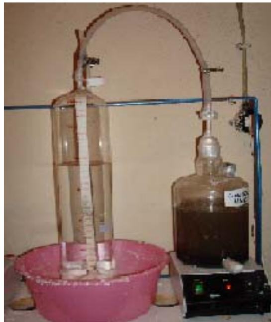
Figure 3.2. 3 L anaerobic reactor with 4L gas collector
