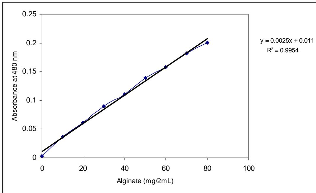
Figure A.1. The calibration curve obtained for the carbohydrate analysis
