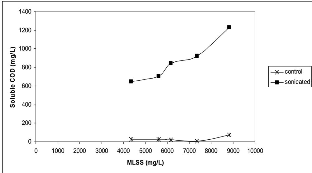
Figure 4.12. Change in soluble COD with respect to MLSS concentration of sludge
