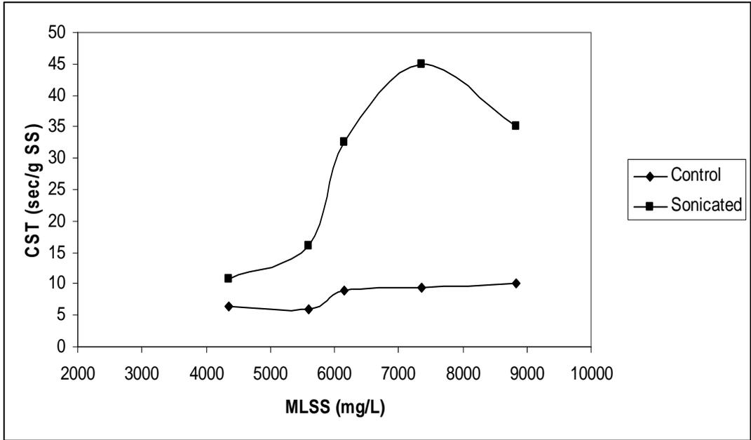
Figure 4.14. Change in CST with respect to MLSS concentration of sludge
