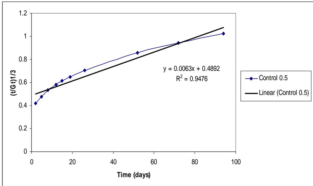
Figure C.4. Representation of regression analysis of methane gas production of control reactor at F/M ratio of 0.5 using Thomas Method
