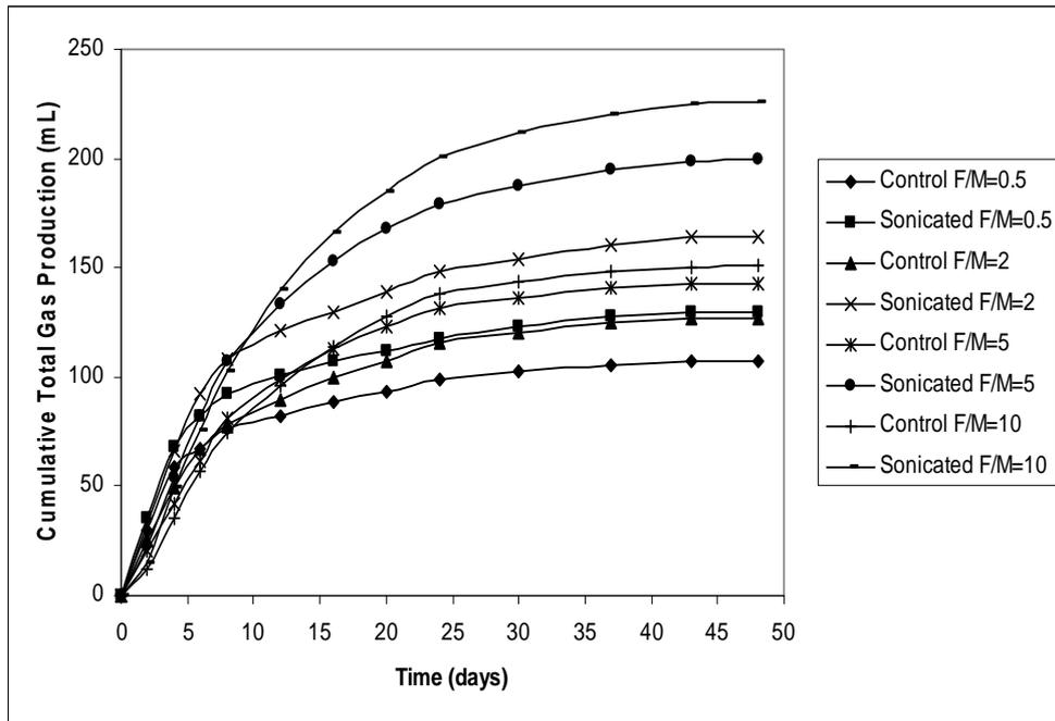
Figure 4.32. The daily change in cumulative total gas production of 250 mL reactors at different F/M ratios during anaerobic digestion
