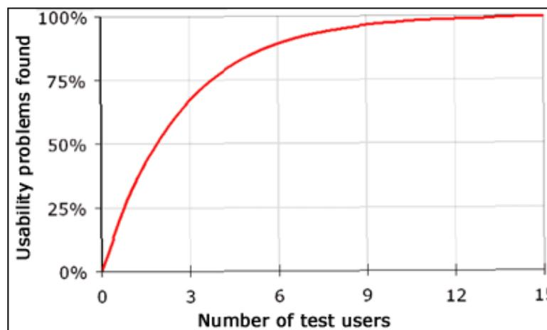
**Figure 5.14 Adequate number of evaluators for usability testing [Nielsen, 2000]**
