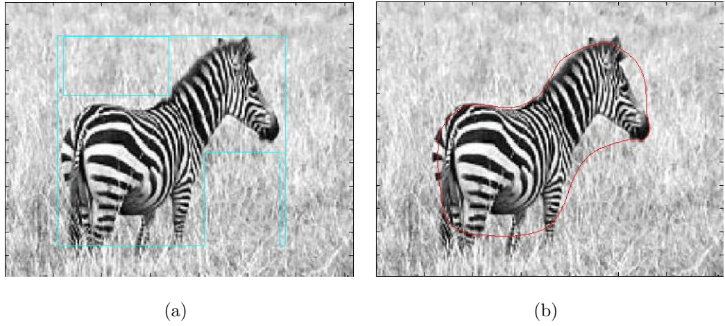
Figure 5.22: Gabor-space geodesics active contour method, zebra-2 image.
