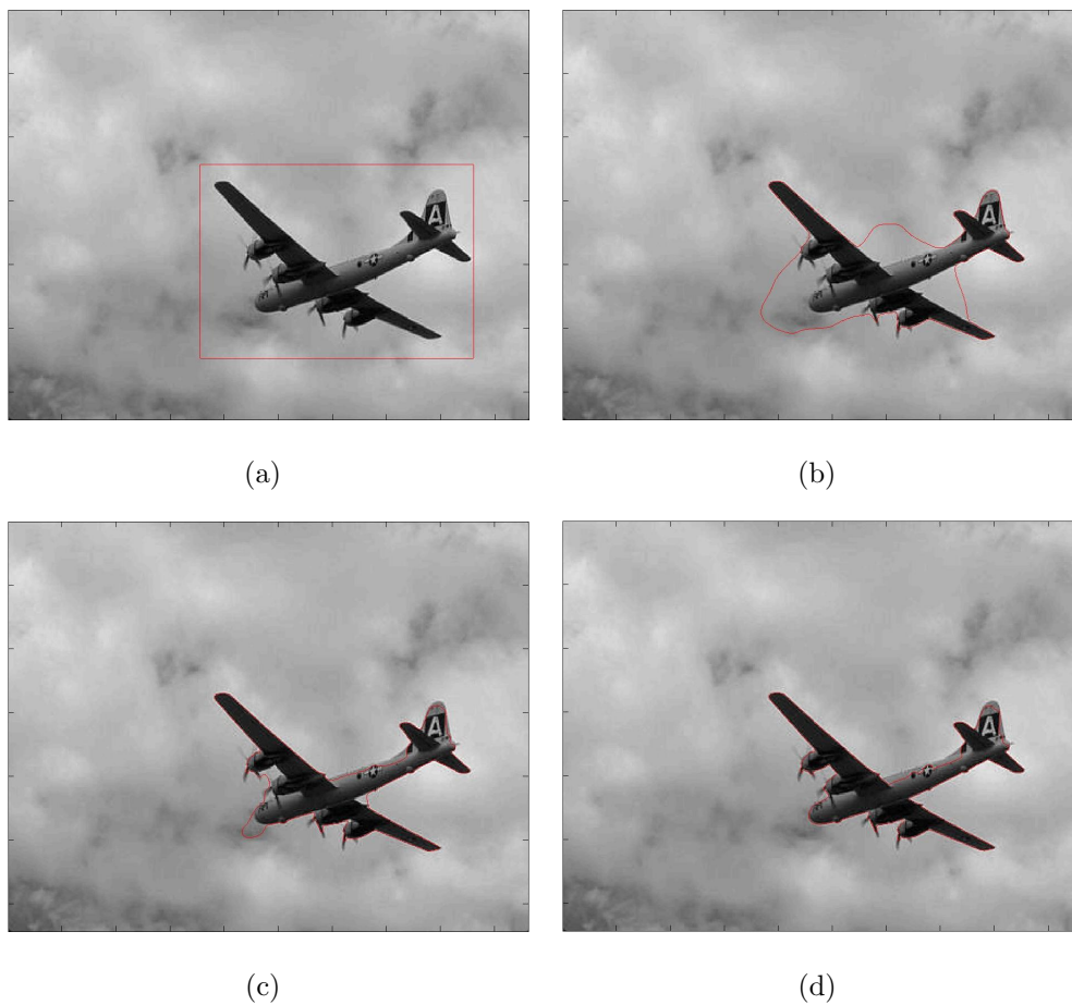
Figure 3.14: Segmentation by the CV method, plane image. (a) Initial contour. (b)- (c)- (d) 800, 1400, 1800 iterations (1211 s).
