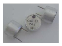
Figure 3-3 C40-12 series ultrasonic transducers
