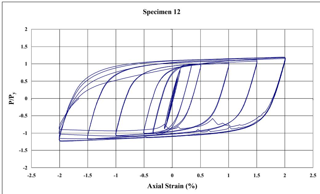
Figure 2.29 – Normalized Axial Load vs. Axial Strain for Specimen 12
