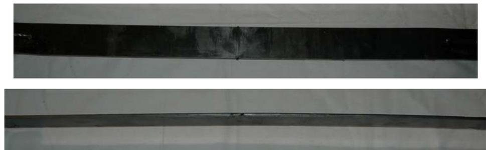
**Figure 2.31 (continued) – Buckling Patterns of Specimens**
