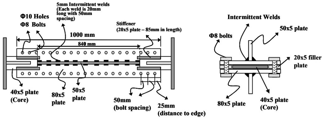
Figure 2.20 – Representative Drawing of Specimen 8 (Not to Scale)
