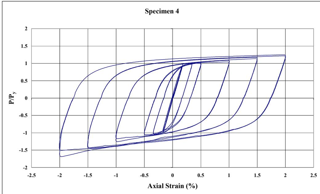
**Figure 2.12 - Normalized Axial Load vs. Axial Strain for Specimen 4**
