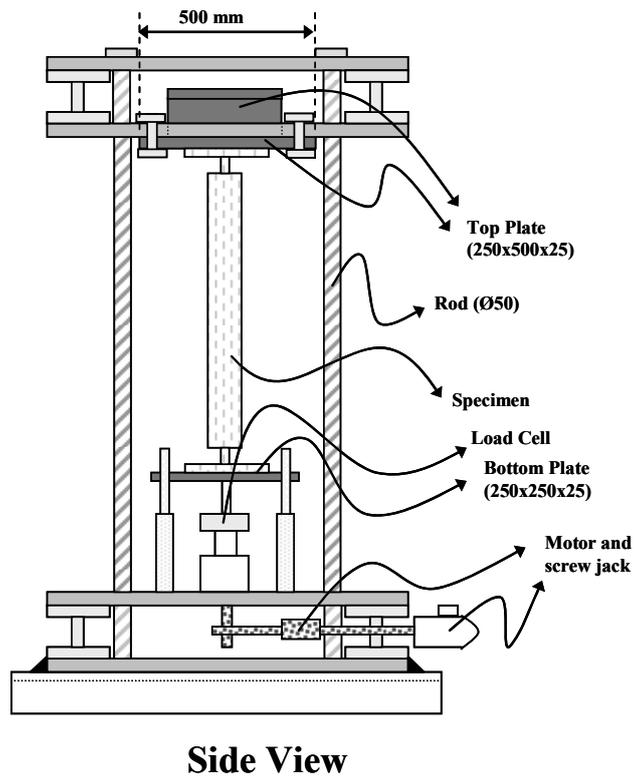
Figure 2.1 - Representative Drawing of the Test Setup (Not to Scale)
