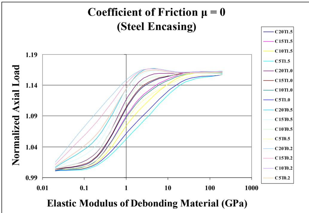
Figure 3.4 – Normalized Axial Loads for Steel Encased Cases
