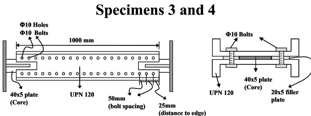
Figure 2.10 – Representative Drawing of Specimens 3 and 4 (Not to Scale)
