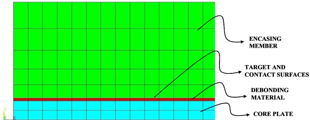
**Figure 3.2 – Typical Finite Element Mesh**
