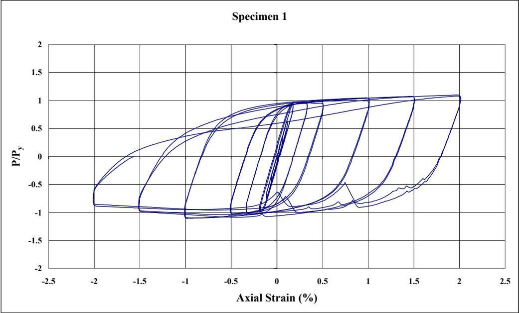
Figure 2.6 – Normalized Axial Load vs. Axial Strain for Specimen 1
