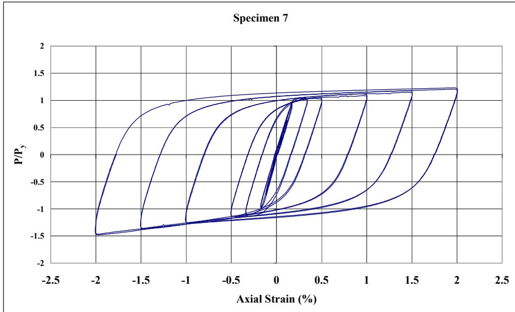
**Figure 2.19 – Normalized Axial Load vs. Axial Strain for Specimen 7**
