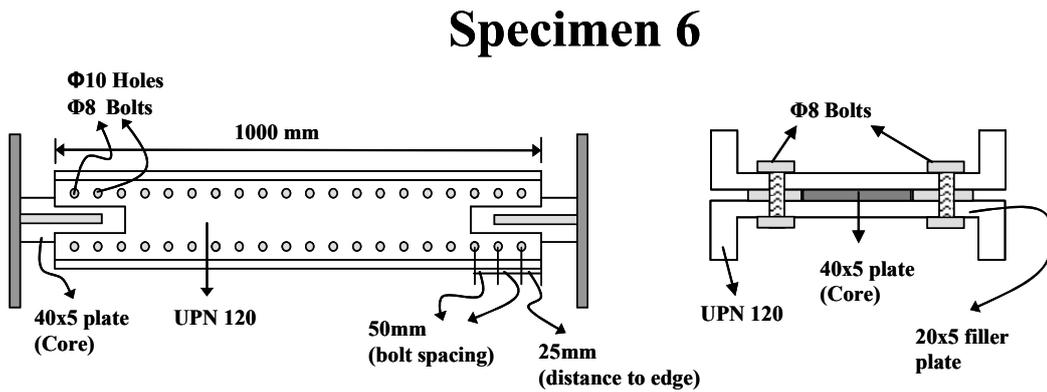
Figure 2.15 – Representative Drawing of Specimen 6 (Not to Scale)
