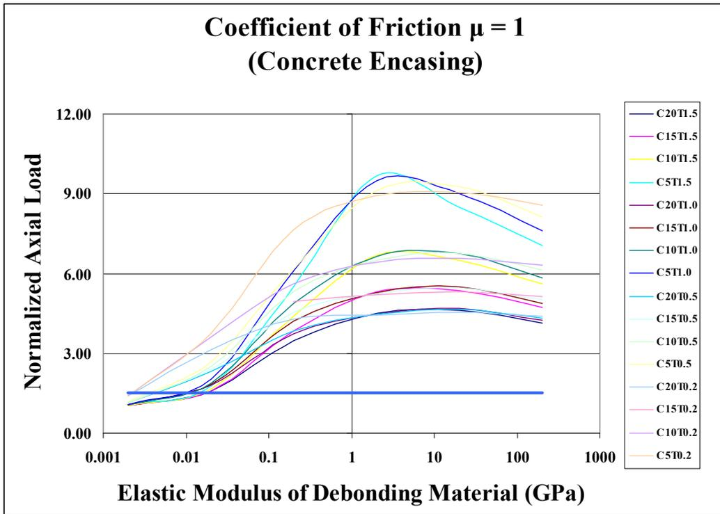
Figure 3.3 (continued) – Normalized Axial Loads for Concrete Encased Cases
