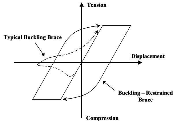
**Figure 1.1 – Comparison of Behavior between a Typical Buckling Brace and a BRB**
