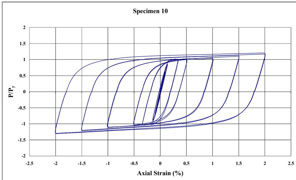
Figure 2.25 – Normalized Axial Load vs. Axial Strain for Specimen 10
