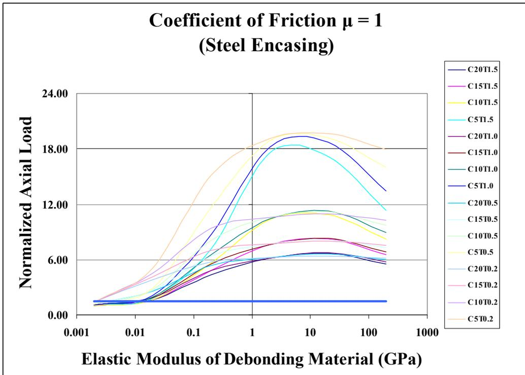
Figure 3.4 (continued) – Normalized Axial Loads for Steel Encased Cases
