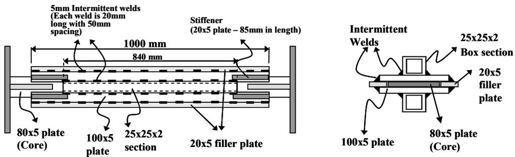
Figure 2.24 – Representative Drawing of Specimen 10 (Not to Scale)
