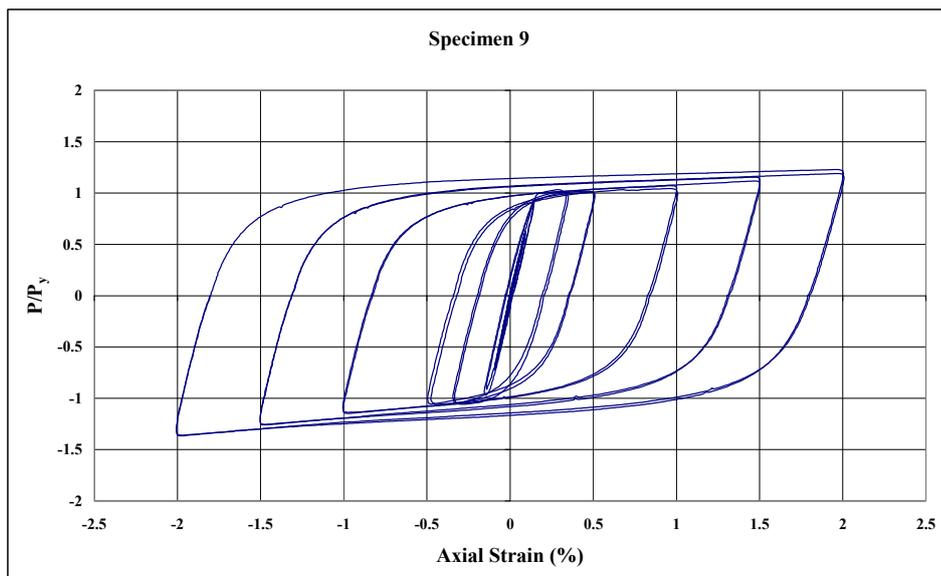
Figure 2.23 – Normalized Axial Load vs. Axial Strain for Specimen 9
