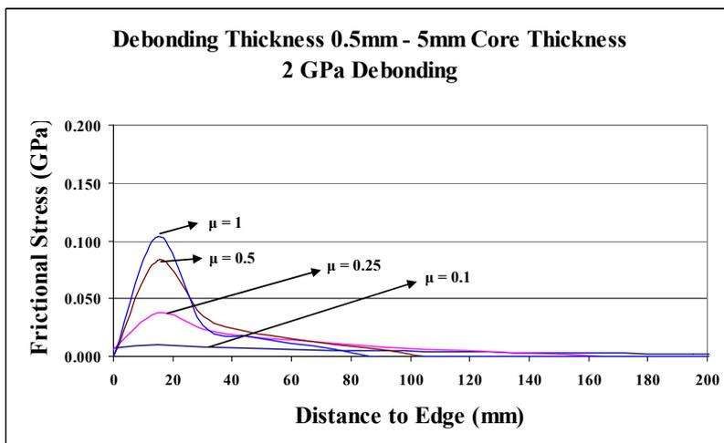
**Figure 3.8 – Frictional Stress Variations for 2 GPa Debonding**
