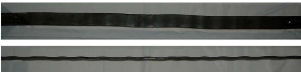
**Figure 2.31 – Buckling Patterns of Specimens**
