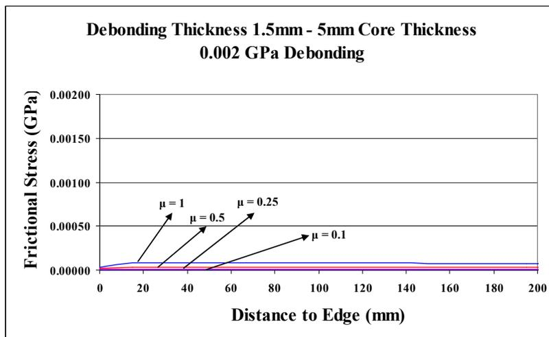
Figure 3.7 – Frictional Stress Variations for 0.002 GPa Debonding
