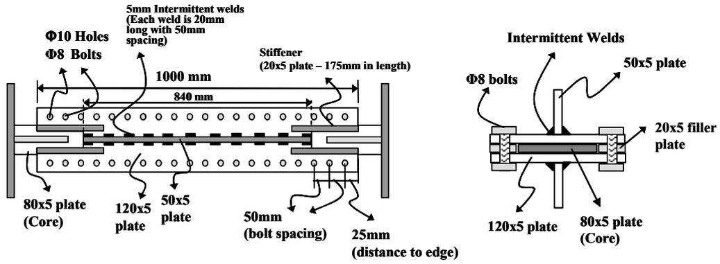
Figure 2.28 – Representative Drawing of Specimen 12 (Not to Scale)
