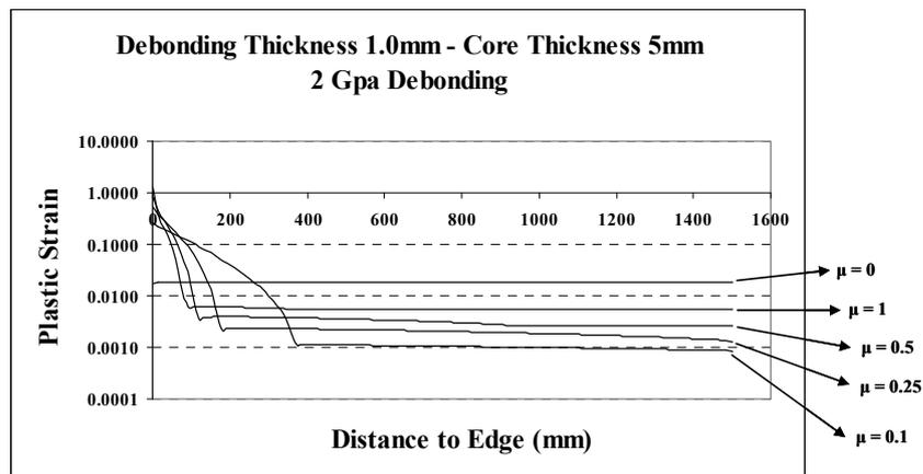
Figure 3.6 – Plastic Strain Variations for 2 GPa Debonding
