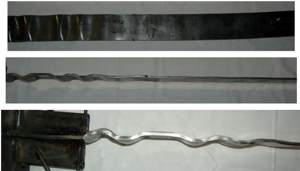
**Figure 2.31 (continued) – Buckling Patterns of Specimens**
