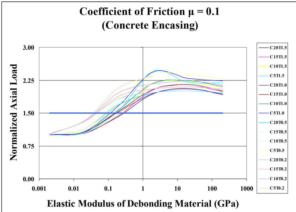
Figure 3.3 – Normalized Axial Loads for Concrete Encased Cases
