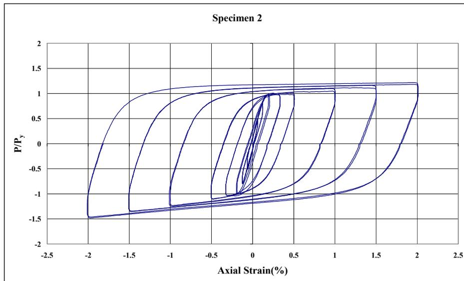
Figure 2.9 - Normalized Axial Load vs. Axial Strain for Specimen 2
