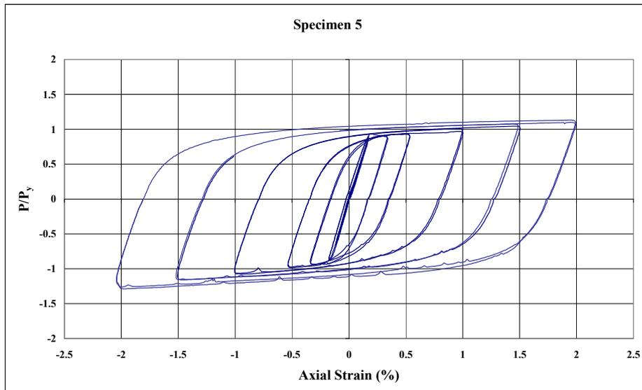
Figure 2.14 - Normalized Axial Load vs. Axial Strain for Specimen 5
