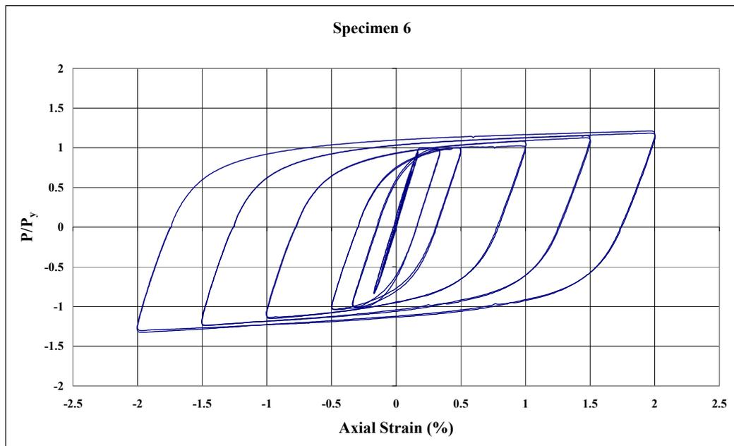
**Figure 2.17 – Normalized Axial Load vs. Axial Strain for Specimen 6**
