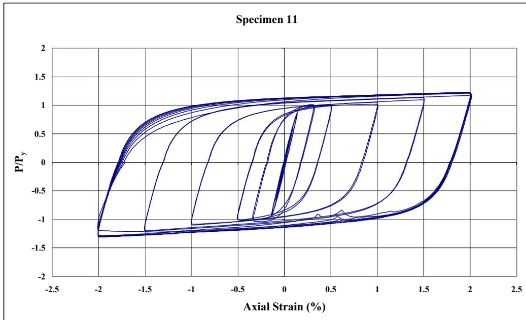
**Figure 2.27 – Normalized Axial Load vs. Axial Strain for Specimen 11**
