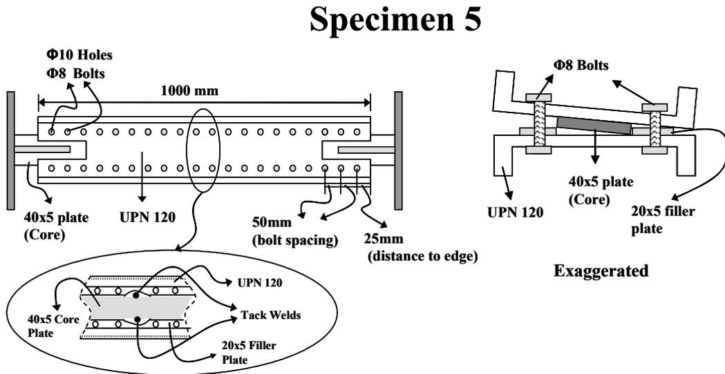
Figure 2.13 – Representative Drawing of Specimen 5 (Not to Scale)
