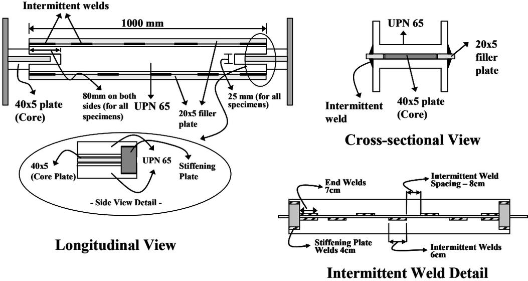
Figure 2.5 – Representative Drawing of Specimen 1 (Not to Scale)
