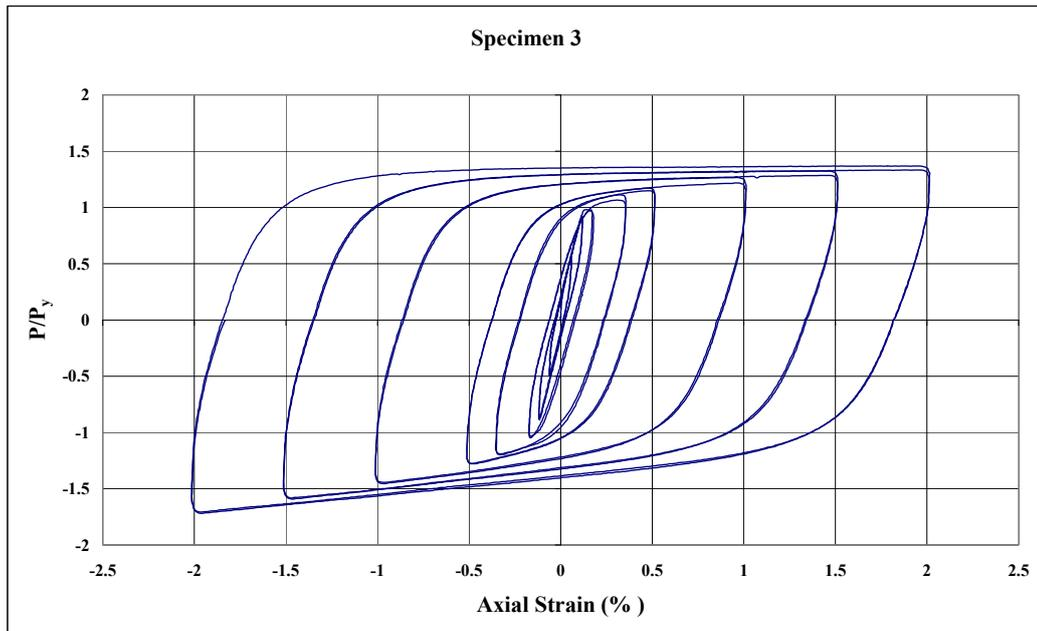
**Figure 2.11 - Normalized Axial Load vs. Axial Strain for Specimen 3**
