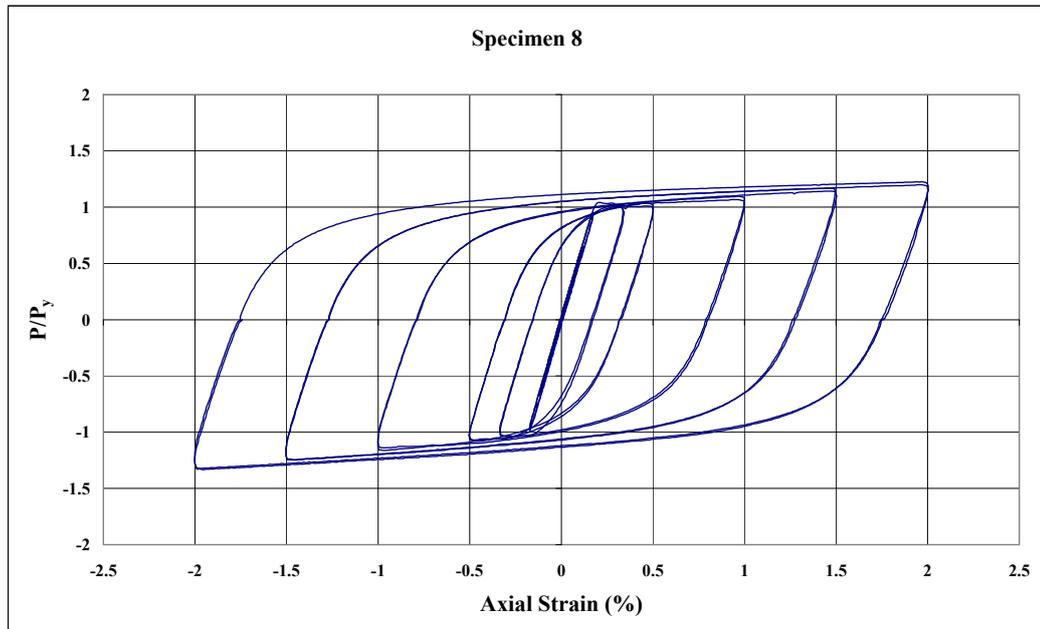
Figure 2.21 – Normalized Axial Load vs. Axial Strain for Specimen 8
