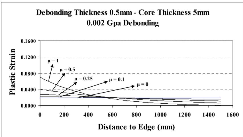
**Figure 3.5 – Plastic Strain Variations for 0.002 GPa Debonding**
