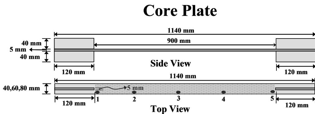
Figure 2.4 – Drawing of Typical Core Plate (Not to Scale)
