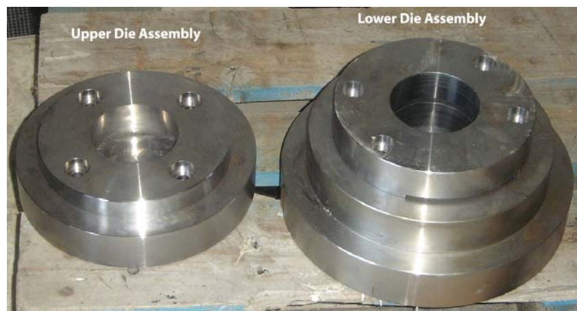
Figure 6.25 A view of Assembly of the Blanking Die Set
