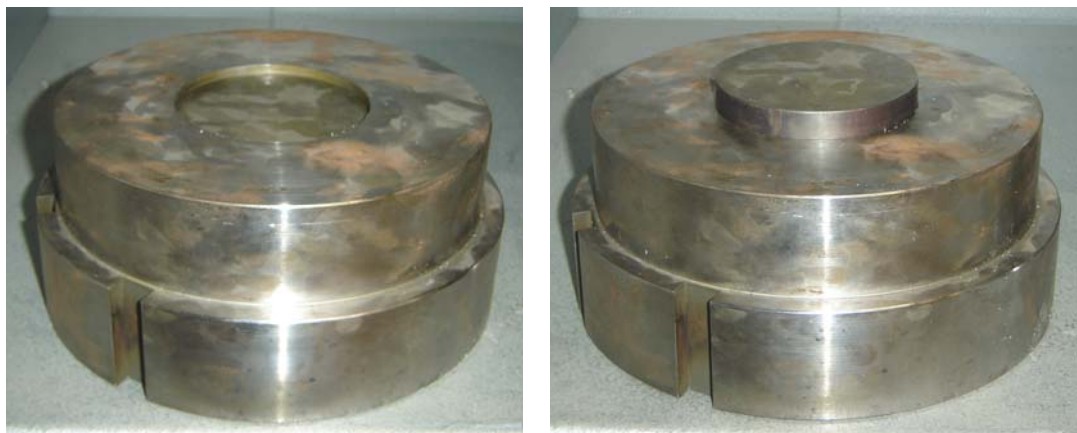
Figure 5.28 A view of Manufactured Lower Coining Die Assembly
