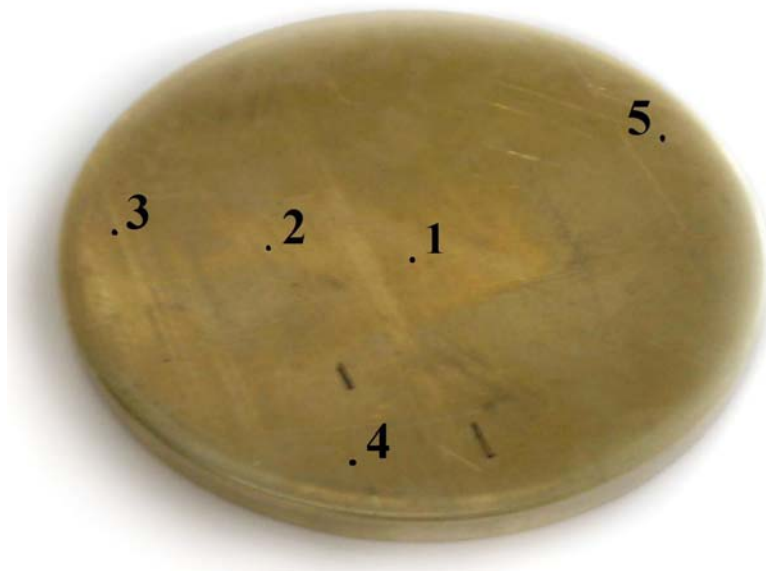
Figure 6.32 Measurement Points after Blanking
