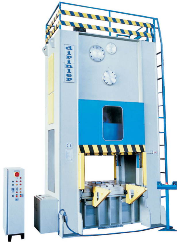
Figure 6.5 A view of Dirinler 200-ton Eccentric Press in METU-BILTIR Center Forging Research and Application Laboratory [34]
