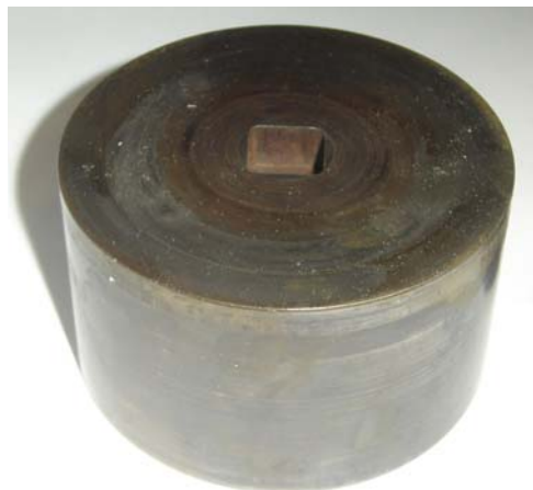
Figure 5.21 A view of Manufactured Lower Die of Coining Die Set
