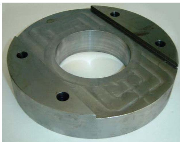
Figure 6.15 A view of Manufactured Guide Plate of Blanking Die Set
