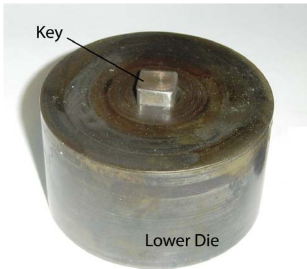
Figure 5.29 A view of Manufactured Lower Coining Die Assembly with the Rectangular Key
