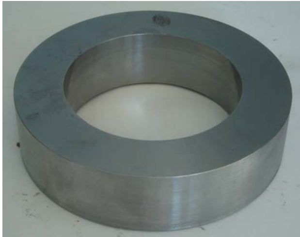
Figure 6.18 A view of Manufactured Lower Blanking Die
