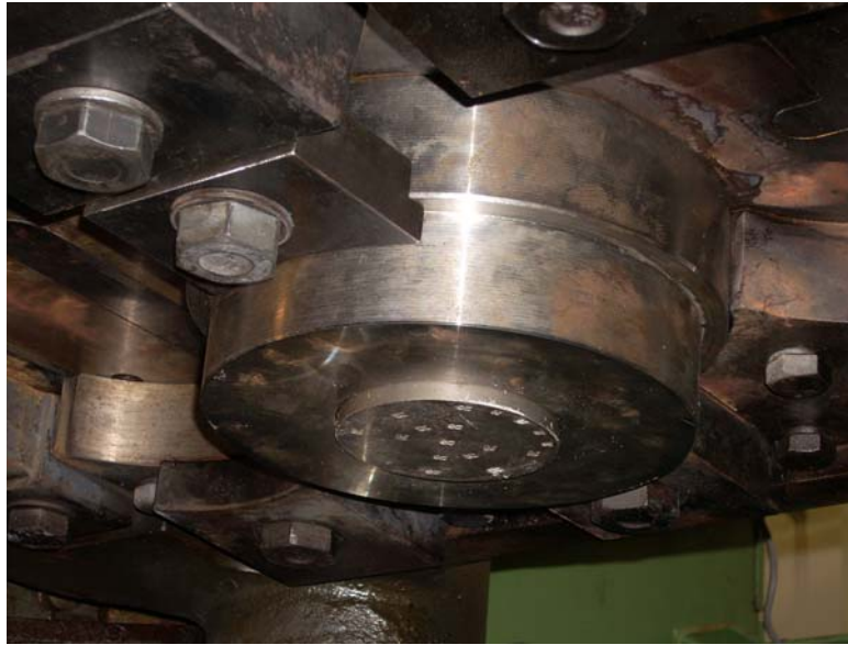
Figure 7.24 Manufactured Interchangeable Upper Die Set for Experimental Medallion
