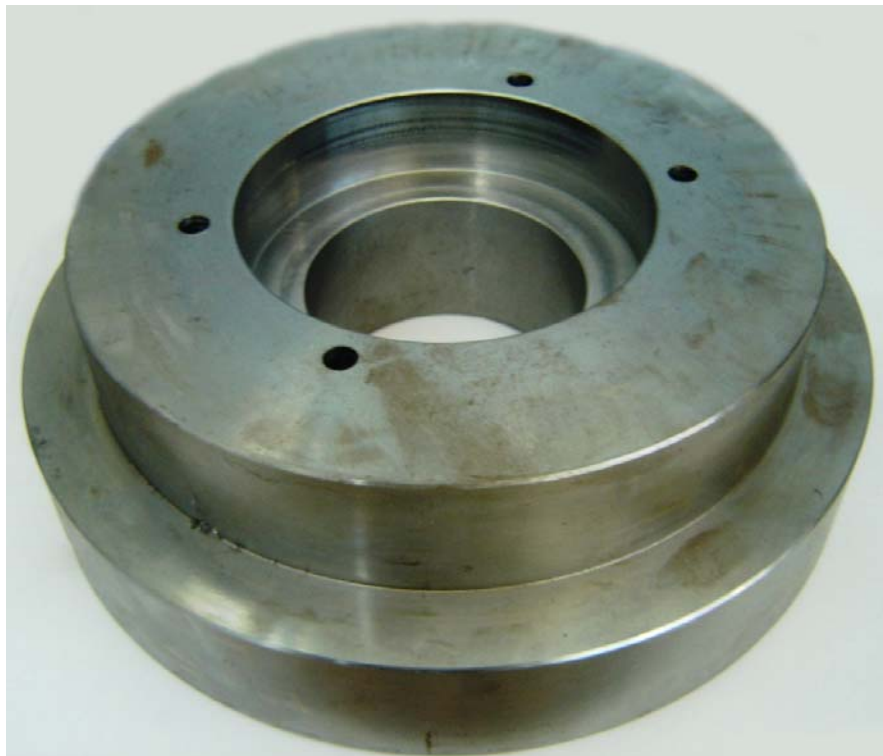
Figure 6.19 A view of Manufactured Lower Blanking Supporting Die
