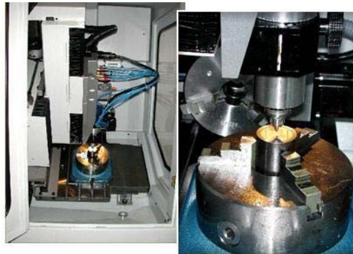
b) Manufacturing of guide die in the same machine
