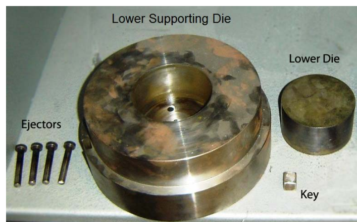
Figure 5.25 A view of Lower Coining Die Assembly Parts
