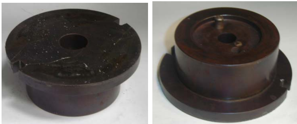
Figure 5.19 A view of Manufactured Fixed Part of Upper Coining Die
