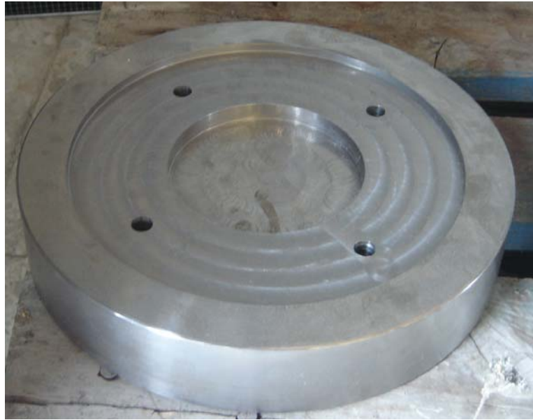
Figure 6.8 A view of Manufactured Upper Blanking Supporting Die
