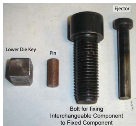
Figure 5.35 Lower Die Key, Pin, Bolts and Ejector for Coining Die Set
