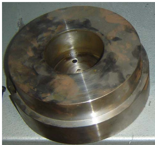
Figure 5.17 A view of Manufactured Upper Coining Supporting Die
