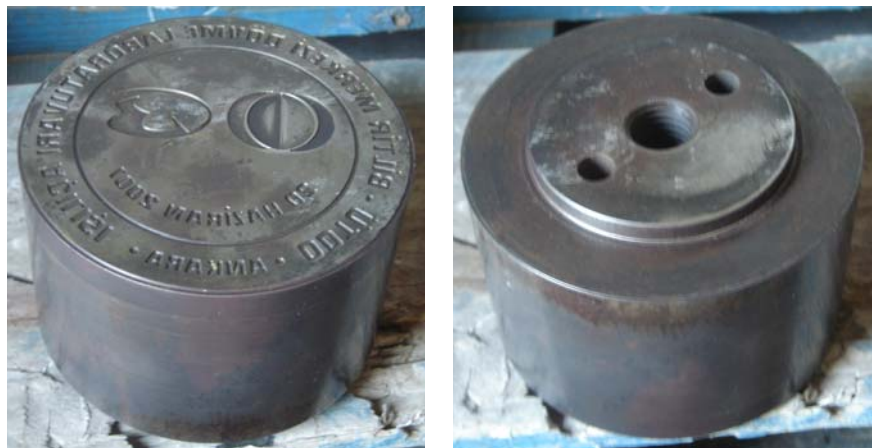
Figure 5.15 A view of Manufactured Interchangeable Part of Upper Coining Die
