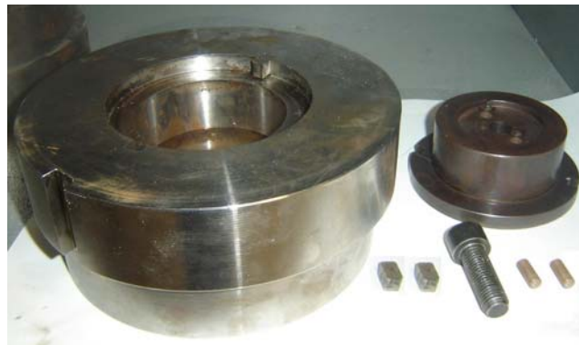
Figure 5.24 A view of Upper Coining Die Assembly Parts
