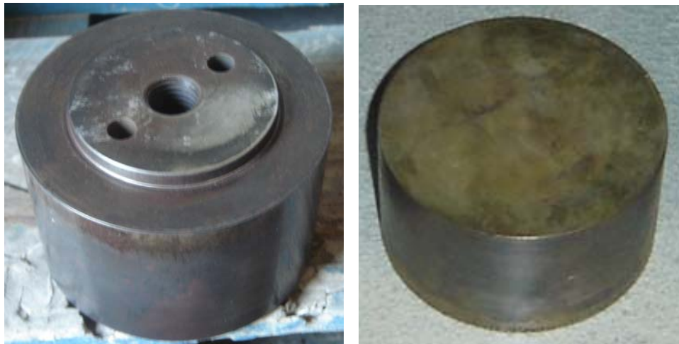
Figure 6.9 A view of Manufactured Interchangeable Component of Blanking Upper Die
