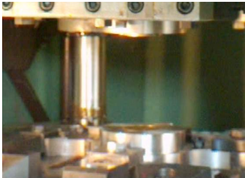
Figure 5.36 A view of Mounted Coining Dies on the Press
