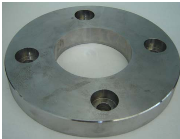
Figure 6.13 A view of Manufactured Upper Die Support of Blanking Die Set
