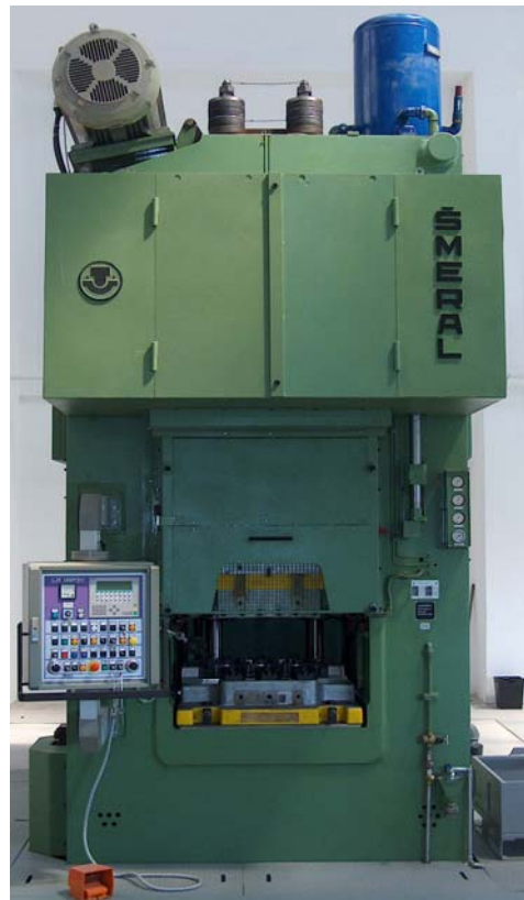
Figure 5.9 A view of Smeral 1000-ton Mechanical Press in METU-BILTIR Center Forging Research and Application Laboratory
