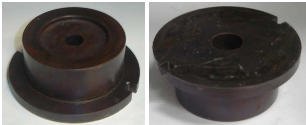
Figure 6.11 A view of Manufactured Fixed Component of Blanking Upper Die
