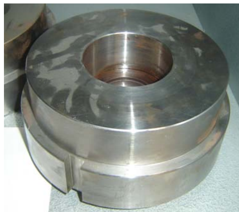
Figure 5.23 A view of Manufactured Lower Coining Supporting Die
