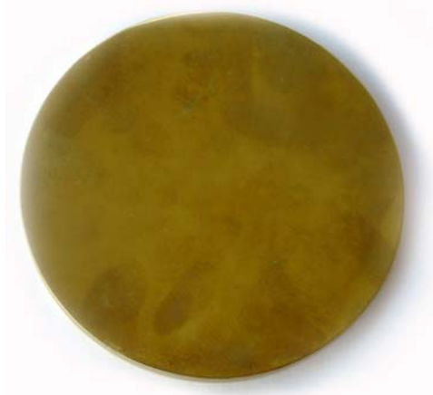
Figure 5.40 Circular Blanks Manufactured with W-EDM
