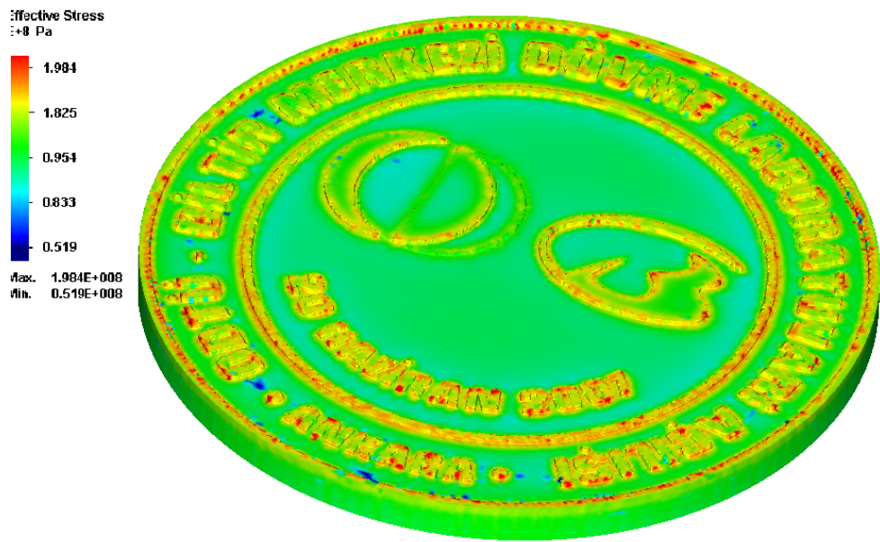
Figure 5.7 Effective Stress Distribution in the Blank with a Diameter of 89mm
