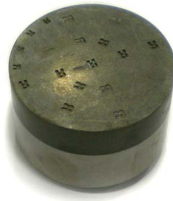
Figure 7.23 Manufactured Interchangeable Upper Die for Blanking Die Set
