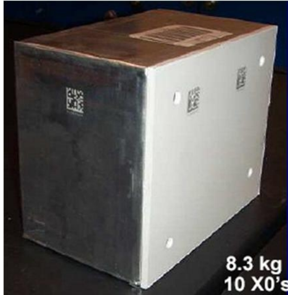
Figure 3.4: The OPERA experiment emulsion cloud chamber (ECC) and Changeable Sheet (CS) that is attached to ECC.
