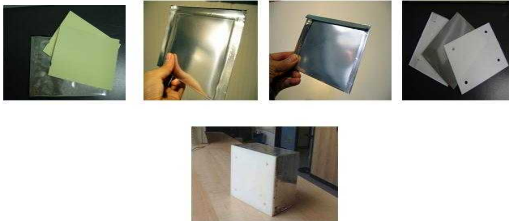
Figure 5.4: CS production steps, packing, clinching and installing. Finally CS is attached to the brick (ECC).
