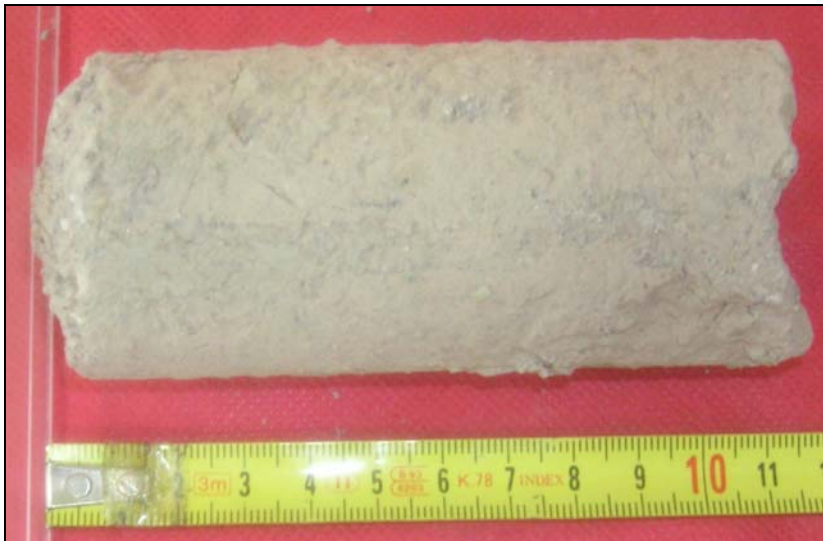
Figure 2.15 Photograph of altered core sample taken from BH-4.
