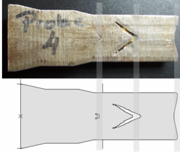
Figure 4.28: Comparison of the experimental and numerical cracks.
