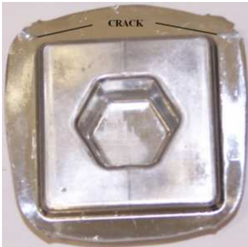
Figure 5.21 Crack Observation in the Flash Zone for the Forging Temperature of 250 °C
