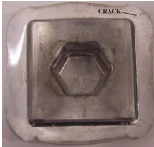
Figure 5.20 Crack Observation in the Flash Zone for the Forging Temperature of 300 °C
