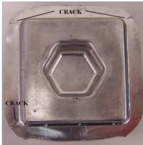
Figure 5.22 Crack Observation in the Flash Zone for the Forging Temperature of 200 °C
