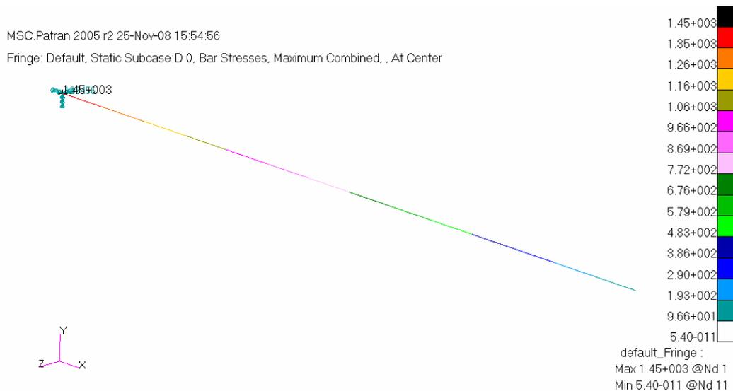
Figure 5.50 Cantilever I beam initial bending stress distribution
