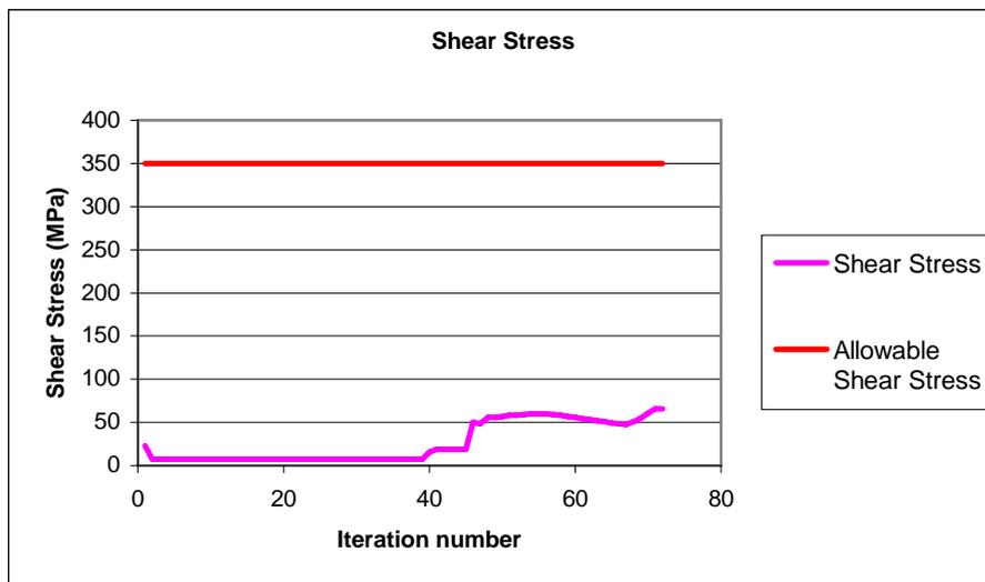
Figure 5.43 Variation of maximum shear stress at the root of the beam with respect to iteration number
