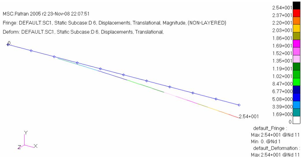
Figure 5.21 Displacement distribution in the optimized beam
