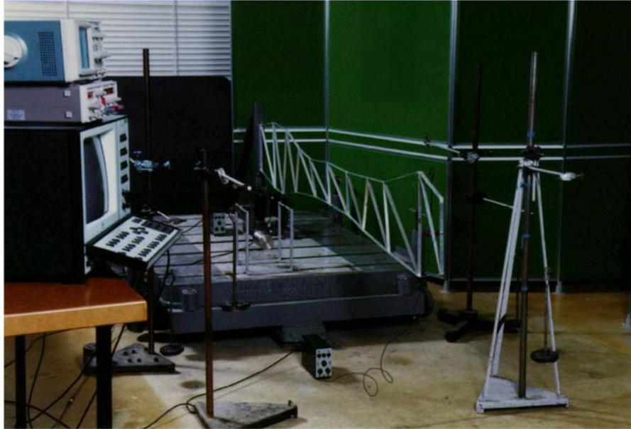
Figure 1.4 Optimized satellite structure on test [5]
