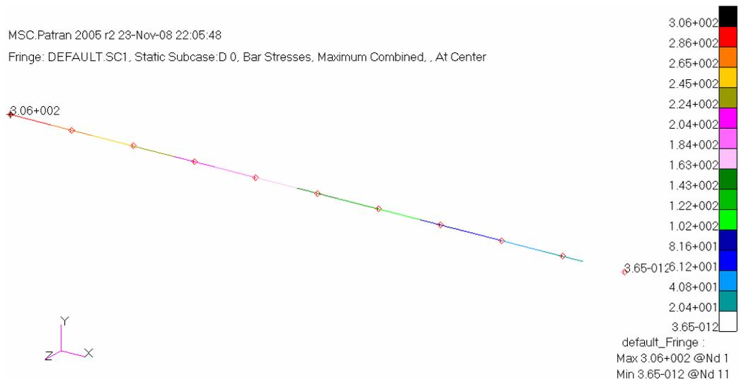
Figure 5.18 Cantilever beam initial stress distribution
