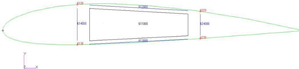
Figure 6.13 Elements of rib 6
