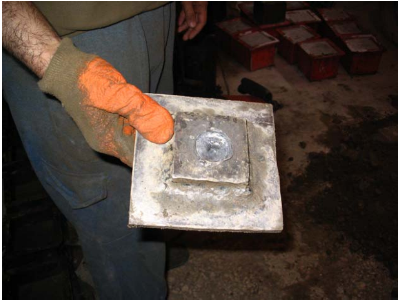
Figure 3.7 A view of the apparatus used for compaction of cubic specimens
