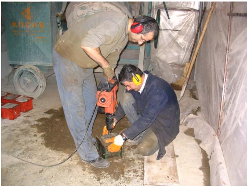
Figure 3.8 Typical view of the compaction process
