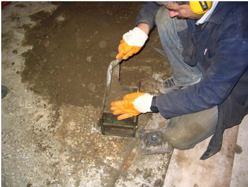
Figure 3.6 A view of the filling of moulds with RCC
