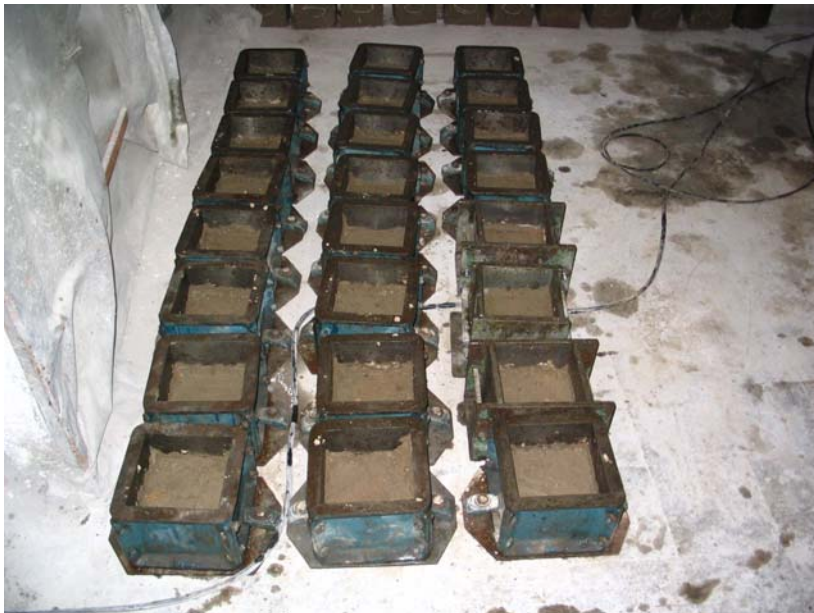
Figure 3.9 A view of the RCC specimens waiting for the application of the bedding mix and the second RCC layer
