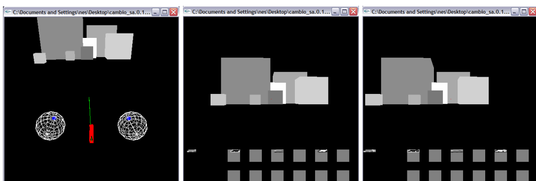
Figure 16 Robot in front of several different shaped and positioned cubes and the views from the left and the right eyes
