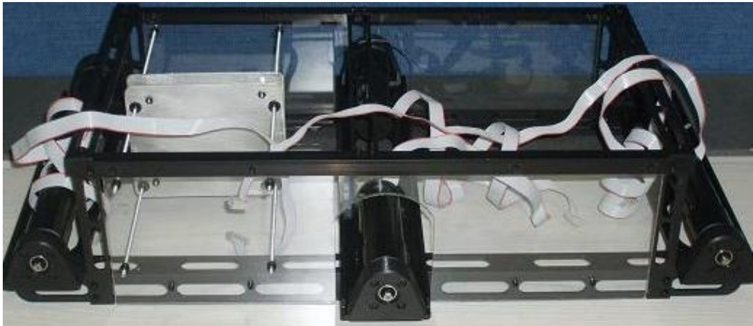
Figure 37 Final assembly of the manufactured parts
