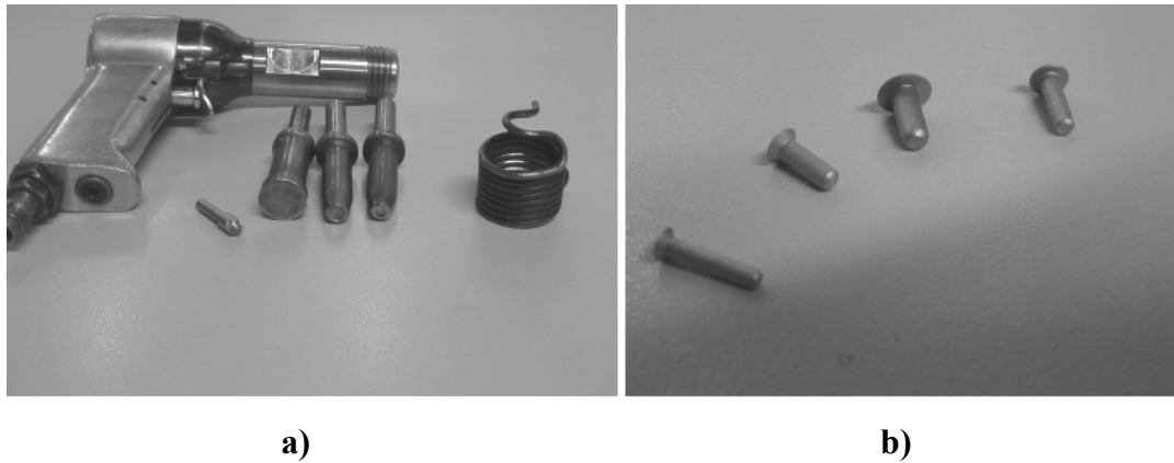
Figure 1.4 a) A view of the air gun used for deforming the rivet head, b) Rivet types [1]
