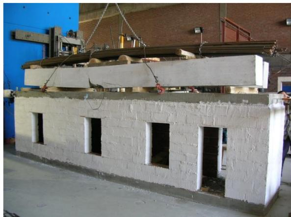
Figure 4.9 Second test with 50 kN of weight above the house
