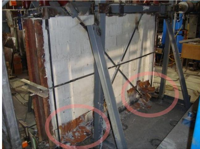
Figure 5.24 Deformed wall in the eighth test
