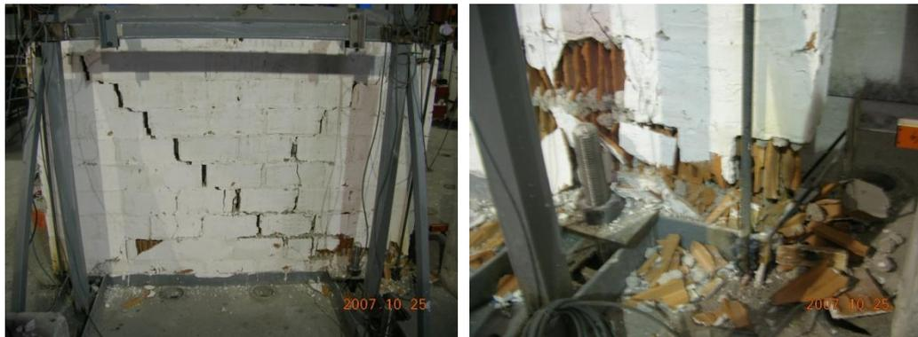
Figure 5.7 Deformed wall in the second test
