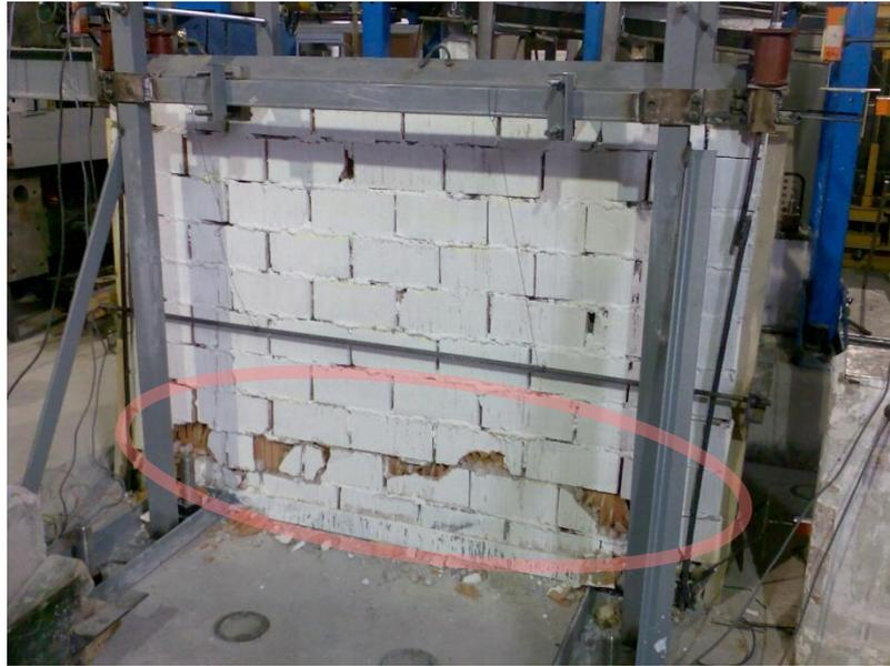
Figure 5.15 Deformed wall in the fifth test
