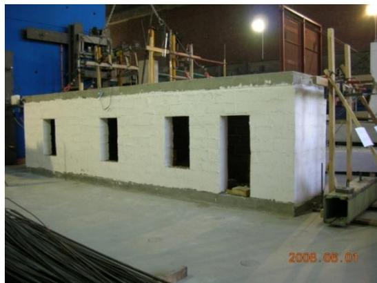
Figure 4.3 Original unstrengthened test specimen
