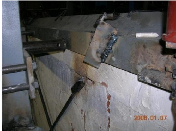
Figure 5.18 Failure at the diagonal rebar during the sixth test
