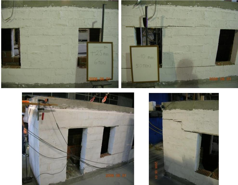
Figure 4.6 Cracks on the first specimen
