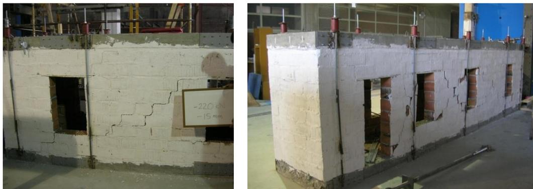
Figure 4.20 Cracks on the fourth test
