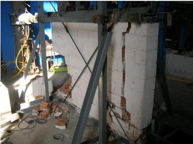
Figure 5.21 Deformed wall in the seventh test
