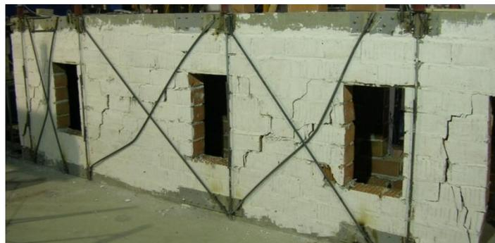
Figure 4.23 Cracks on the fifth test
