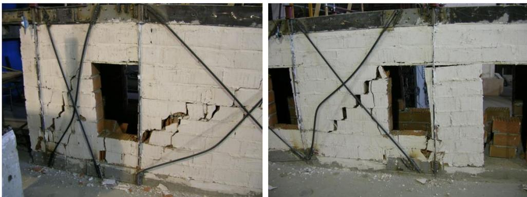
Figure 4.29 Cracks on the sixth test
