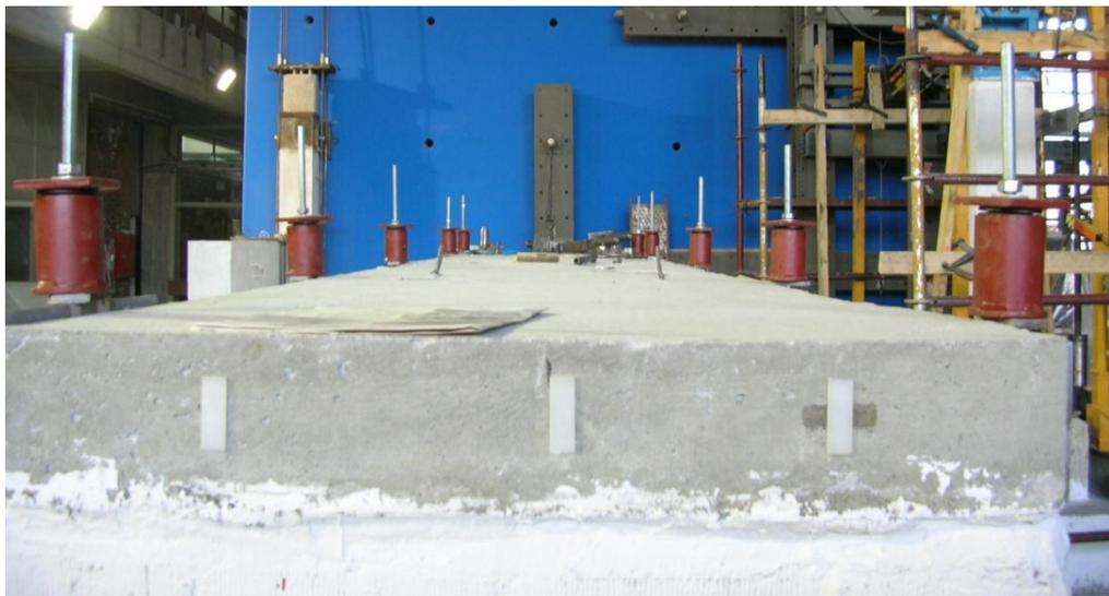
Figure 4.19 Unloaded springs due to wall crushing in the vertical direction
