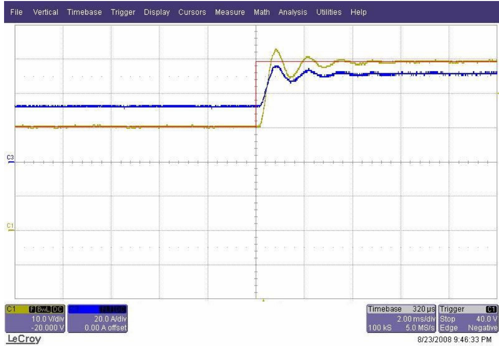
Figure 3.26 Reference tracking capability of the output voltage, output voltage (yellow), load current (blue), reference signal (red). (Scales : 10V/div, 20A/div, 2ms/div).
