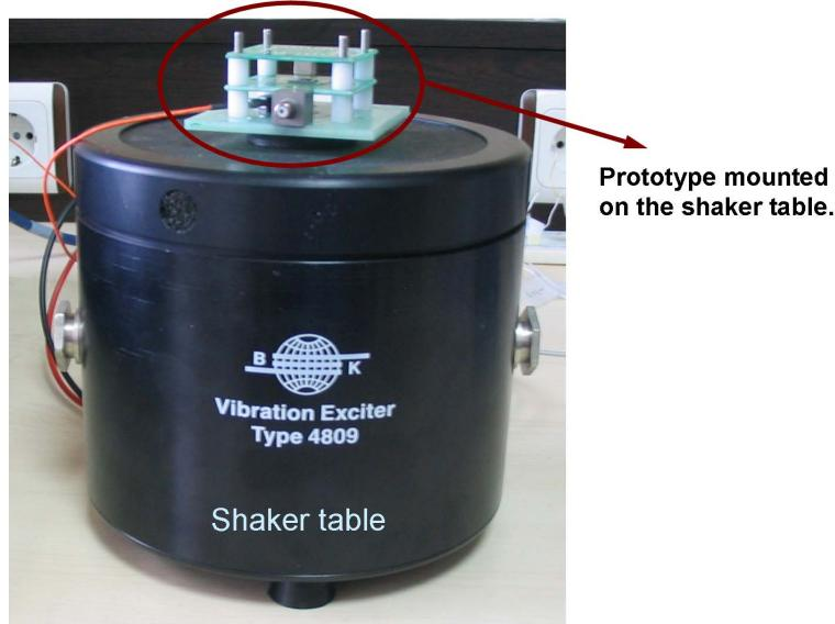
**Figure 4.5. Assembled sample mounted on the shaker table.**
