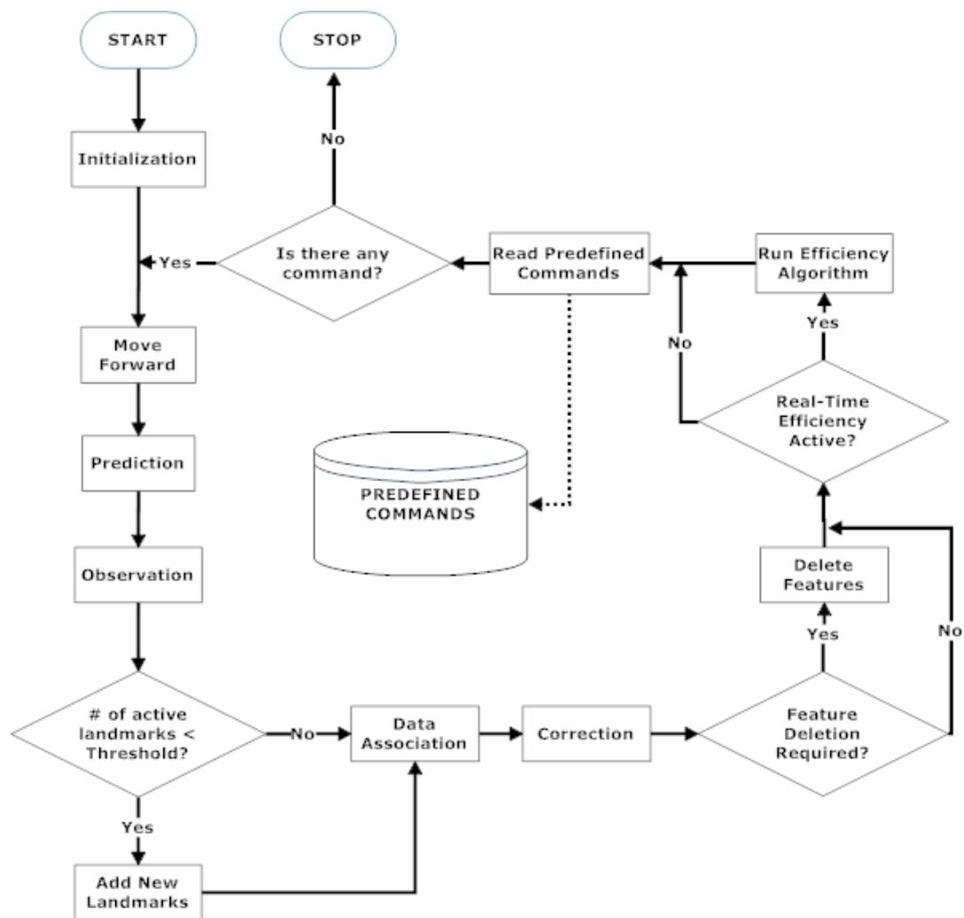
Figure 6-6 Flowchart of SLAM with Predefined Motion
