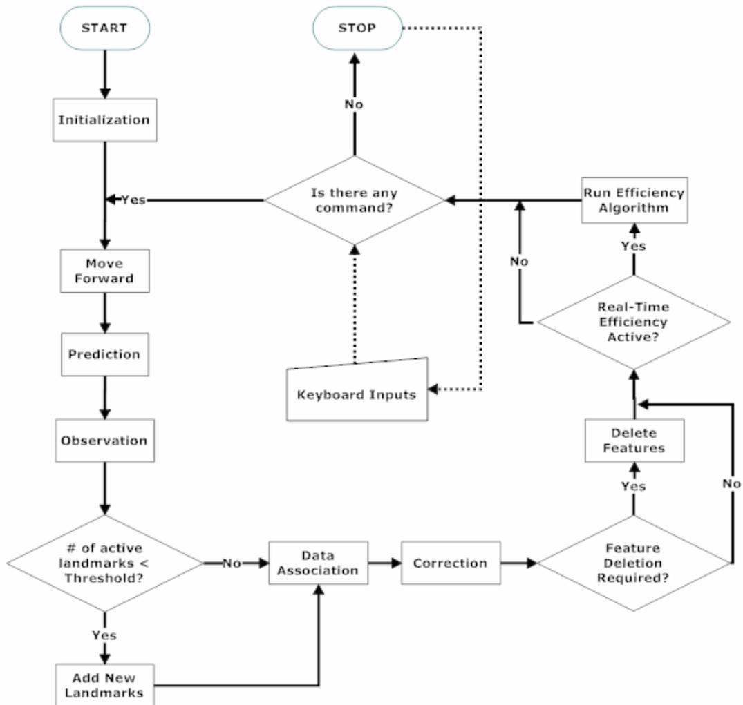
Figure 6-7 Flowchart of SLAM with Manual Inputs
