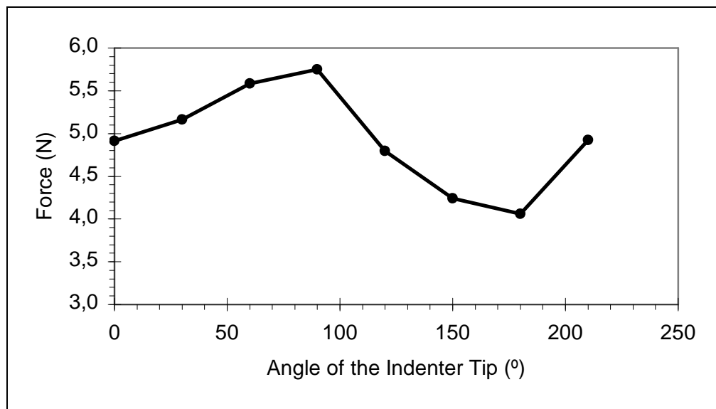
Figure 4.49 Anisotropic response attributed to relaxation behavior. In the test data a 22 mm displacement is applied
