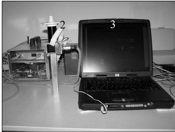
Figure 3.1 Indenter test device. Control box (1) test unit (2) portable computer (3)
