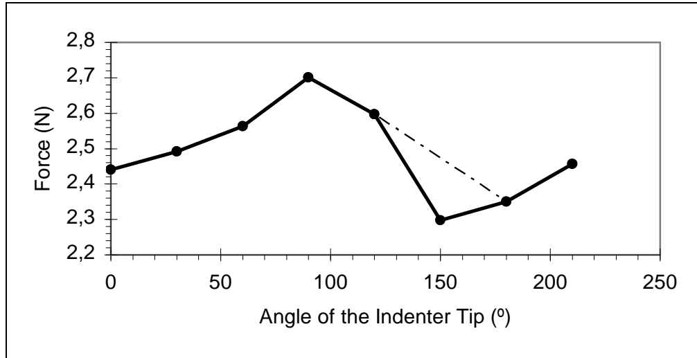
Figure 4.50 Anisotropic response attributed to relaxation behavior. In this test a 17 mm displacement is applied
