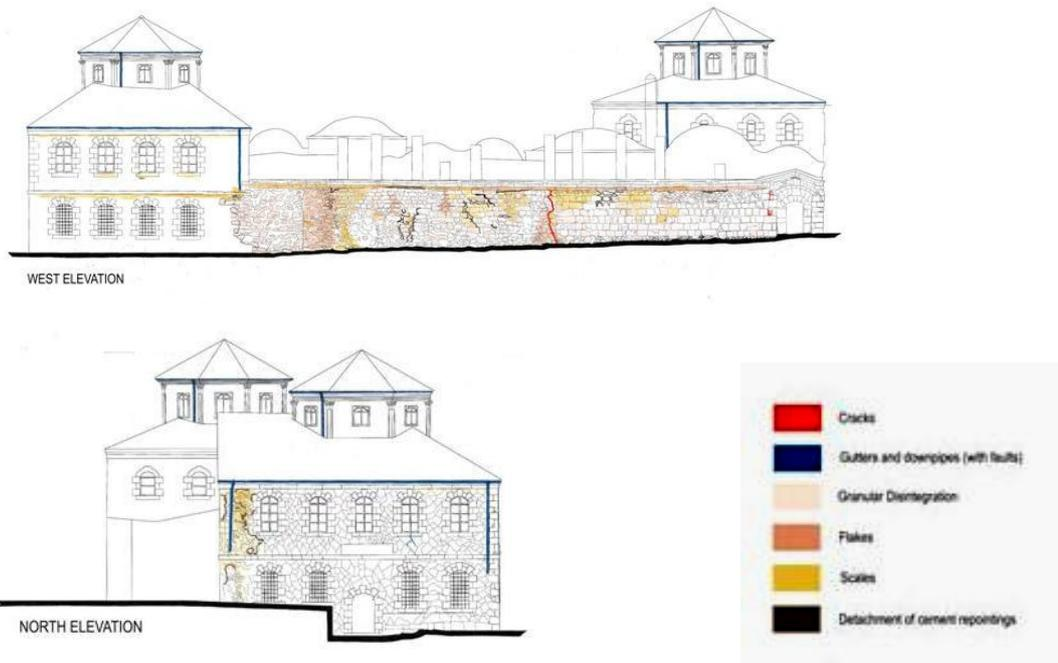
Figure 4.2 Elevations showing the distribution of the material detachment and cracks at the north and west façade of the building.
