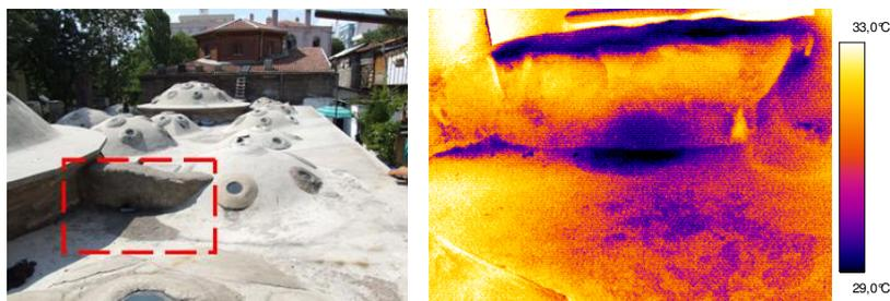
Figure 4.17 The infrared image of the parapet cutting the water flow and causing soil/dirt accumulation in front of its outlet; the gradual decrease of surface temperatures towards the outlet exhibited the potential for absorbing and retaining rainwater.
