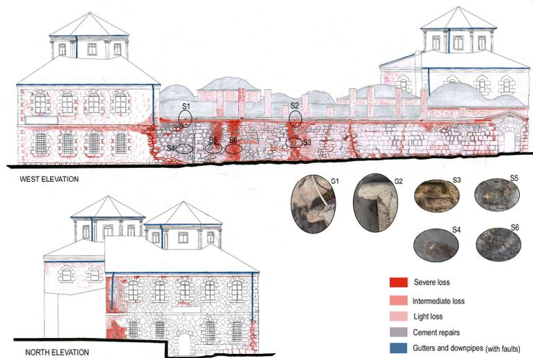
Figure 4.1 Elevations showing the distribution of the severe material loss at the north and west façade of the building. *S1, S2, S3, S4, S5 and S6 show the location of material samples taken from the west façade.* The severe loss and detachment on surfaces was observed together with white staining and salt deposits, especially at the lower parts of the rainwater pipes at both sides of the façade and stone courses at the top, underneath the eaves gutter.
