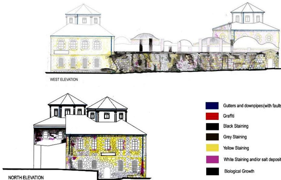
Figure 4.3 Elevations showing the distribution of discoloration and deposits on surfaces of the north and west façade of the building.
