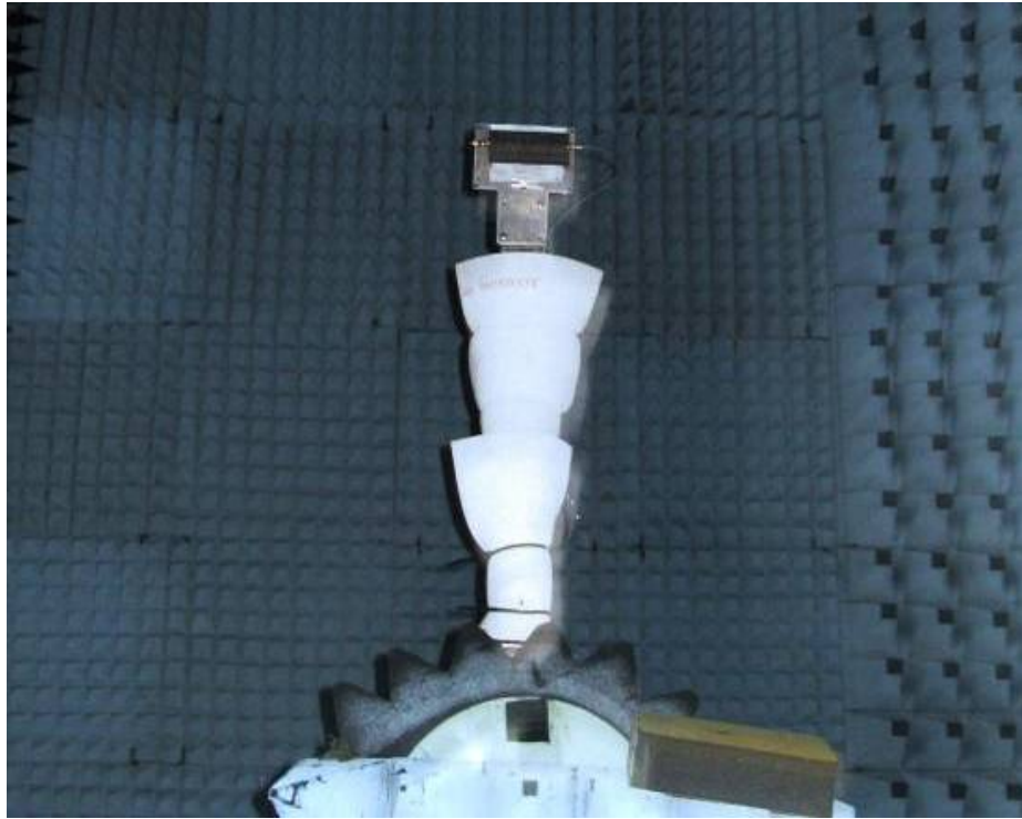
Figure 4.11 Linearly Polarized Meanderline Array under Test in Tapered Anechoic Chamber at ASELSAN Facilities
