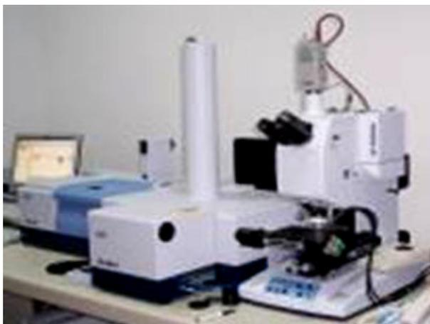
**Figure 2.4** FTIR Spectrometer with ATR objective
