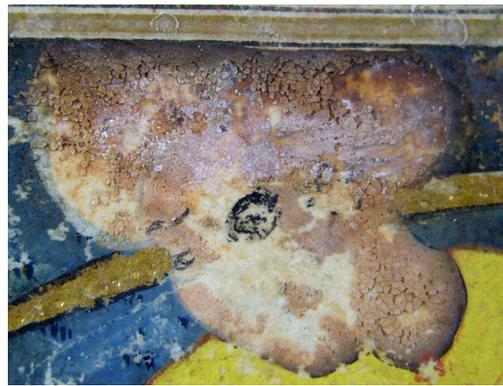
**Figure 1.11** Corroded white lead pigment, black colored regions show occurrence of PbS
