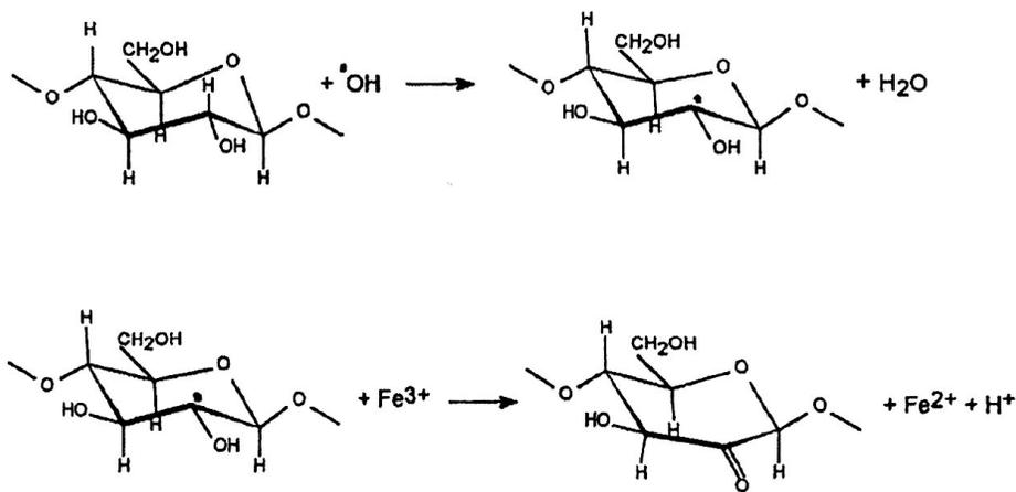
**Figure 1.25** Formation of carbonyl groups in cellulose oxidation by OH radicals in the presence of Fe (II) ions (Gibert *et al.*, 1999).
