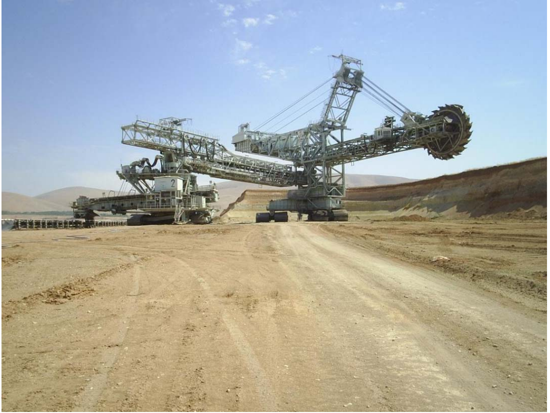
Figure 3.3 Bucket wheel excavator being used in Kışlaköy open cast mine. (Akbulut et al., 2007)
