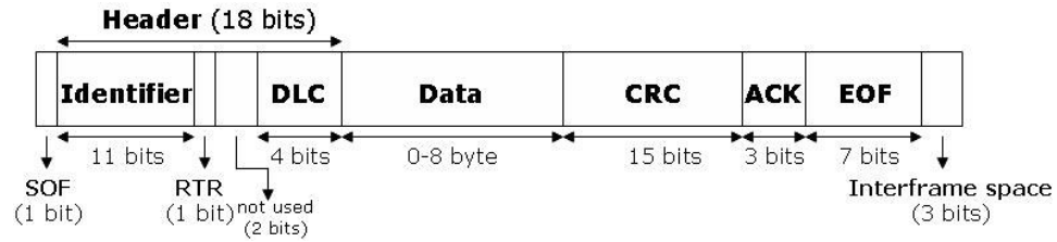
Figure 2.3 CAN 2.0A message format
