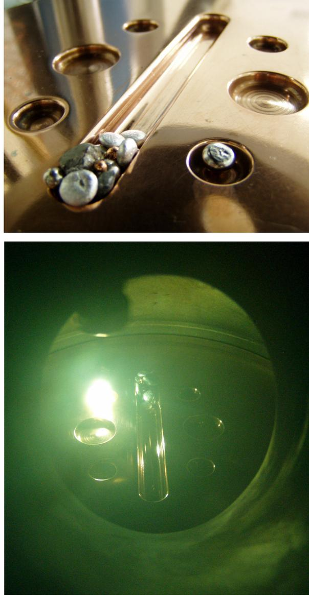
**Figure 4.3** The copper tray and chamber of the Arc-Melting device is cleaned and polished prior to every melting. Zirconium metal standing solely in a small reservoir next to the -to be prepared- alloy is melted in advance to justify the removal of any trace amount of oxygen.
