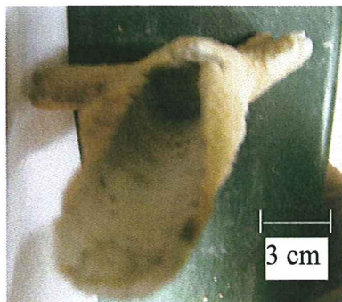
Figure 4.54 Grout masses exposed from the soil specimens of lower density having 25 % of kaolinite (water/solids ratio = 1.5)
