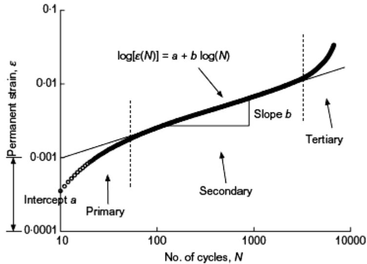
**Figure 2.5 Permanent strain vs. number of cycles in log–log scale (Kanitpong et. al., 2006)**
