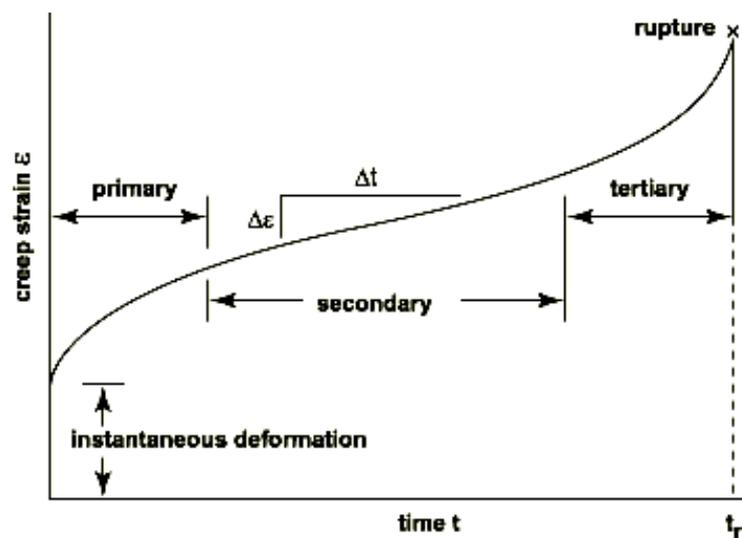
Figure 2.3 Creep Curve (Martin Tarr, “Stress and its effect on materials”)
