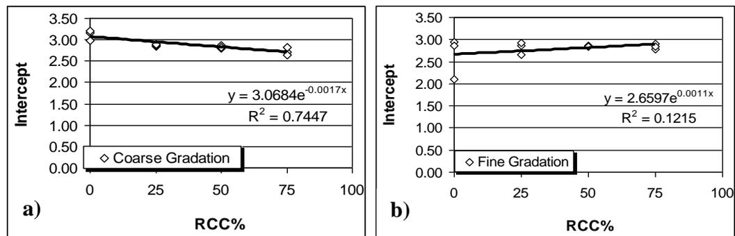
**Figure 5.3 Intercept constant vs. RCC content a) for coarse graded specimens, b) for fine graded specimens**
