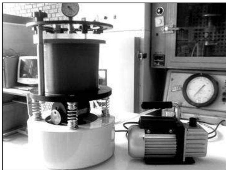
**Figure 3.8** A picture of Rice test measurement system
