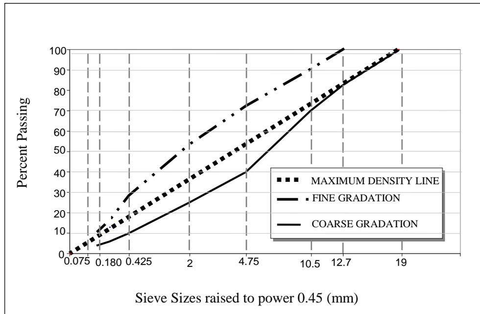
**Figure 3.13 Gradation limits according to the General Directorate of Highways (2006)**
