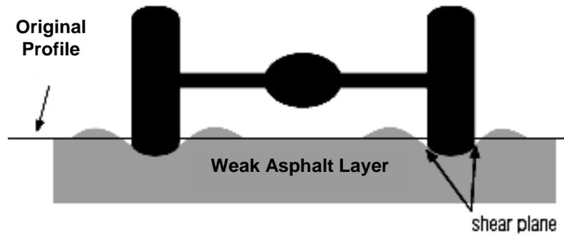
**Figure 2.8 Rutting due to plastic flow (Superpave Mix Design Superpave Series No. 2 (SP-2), Asphalt Institute)**
