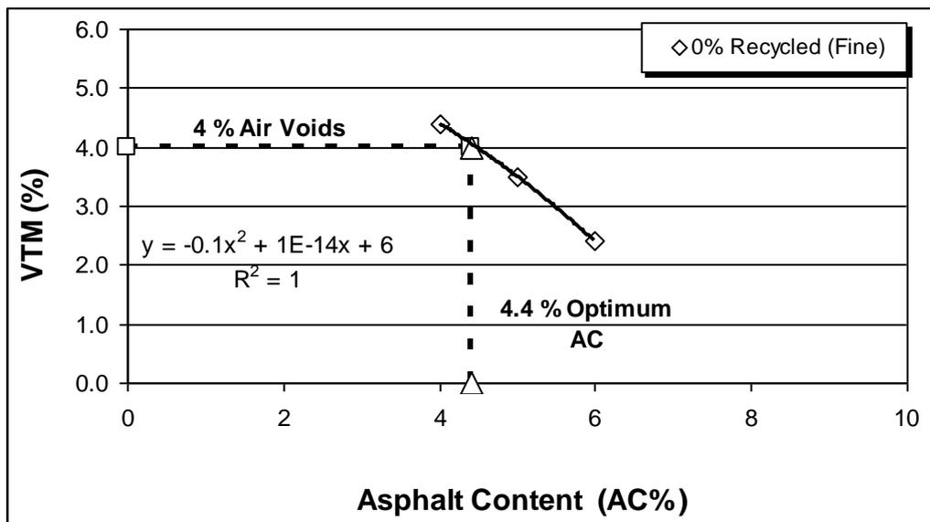
Figure D5 Optimum asphalt content calculation for fine graded tall specimen with 0 % recycled cement concrete
