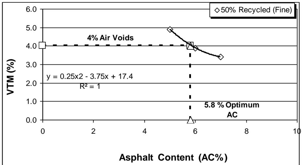
**Figure D3 Optimum asphalt content calculation for fine graded tall specimen with 50 % recycled cement concrete**
