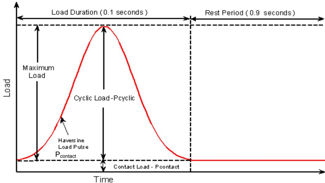
**Figure 2.4 Haversine loading pattern applied in a permanent deformation test (National Cooperative Highway Research Program, Research Results Digest Number 285, 2004)**
