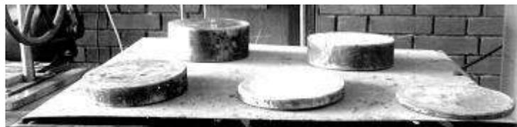
**Figure 3.7 Plates used to maintain constant height in modified Marshall specimens**
