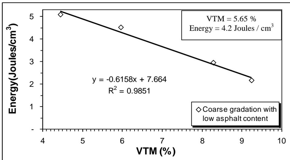
Figure A9 Graph for coarse graded tall specimen with low asphalt content, replicate 2
