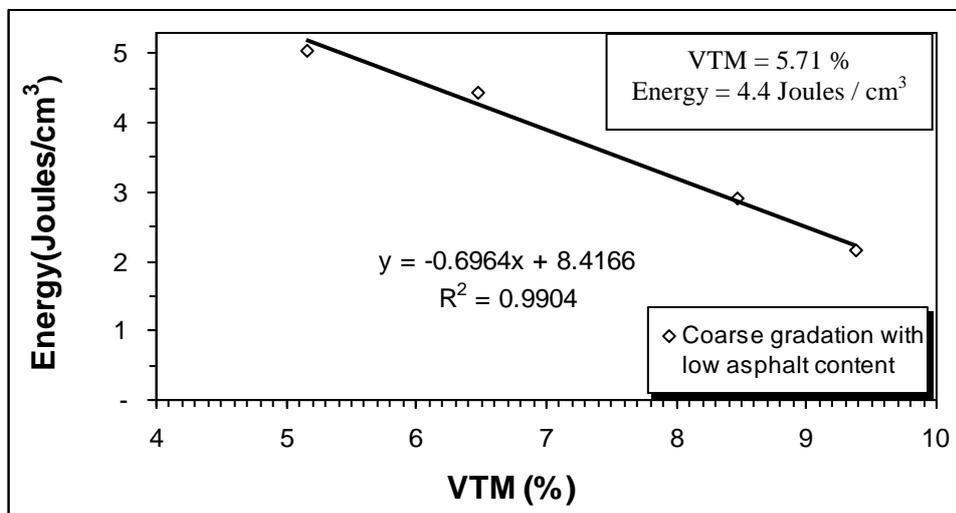
Figure A7 Graph for coarse graded tall specimen with low asphalt content,
