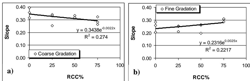
**Figure 5.2 Slope constant vs. RCC content a) for coarse graded specimens, b) for fine graded specimens**
