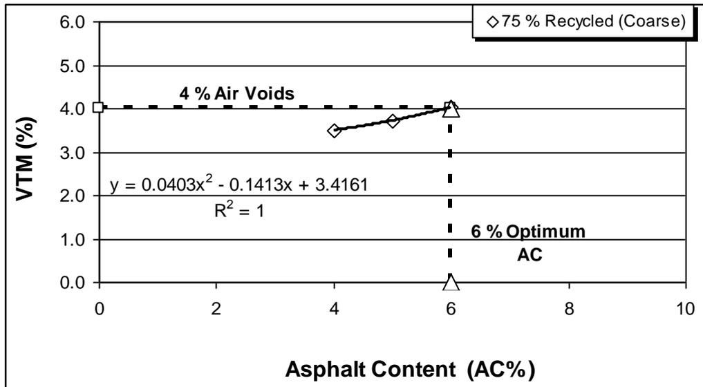
Figure D4 Optimum asphalt content calculation for coarse graded tall specimen with 75 % recycled cement concrete
