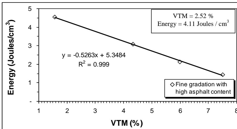
Figure A15 Graph for fine graded tall specimen with high asphalt content, replicate 1
