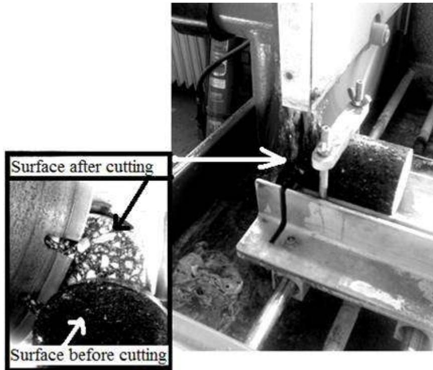
**Figure 3.15 Specimen cutting process**
