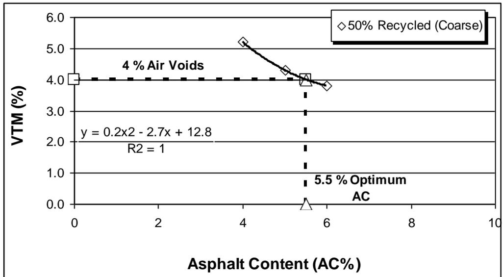
**Figure D2 Optimum asphalt content calculation for coarse graded tall specimen with 50 % recycled cement concrete**
