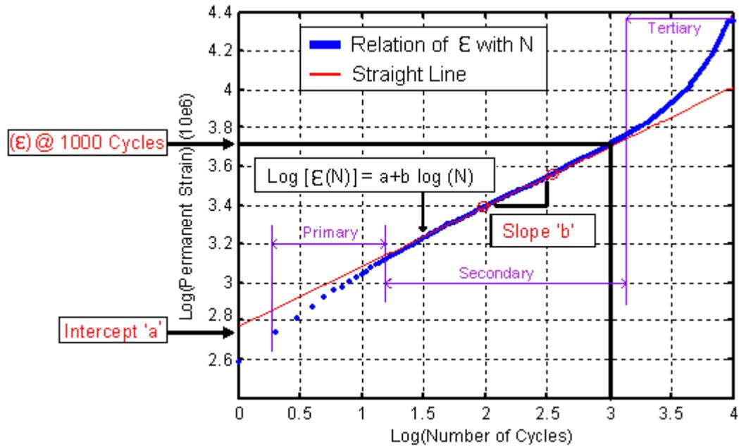
**Figure 3.11 Calculation of slope, intercept and  $(\epsilon)$  @ 1000 cycles for fine graded tall specimen with 75 % RCC content**
