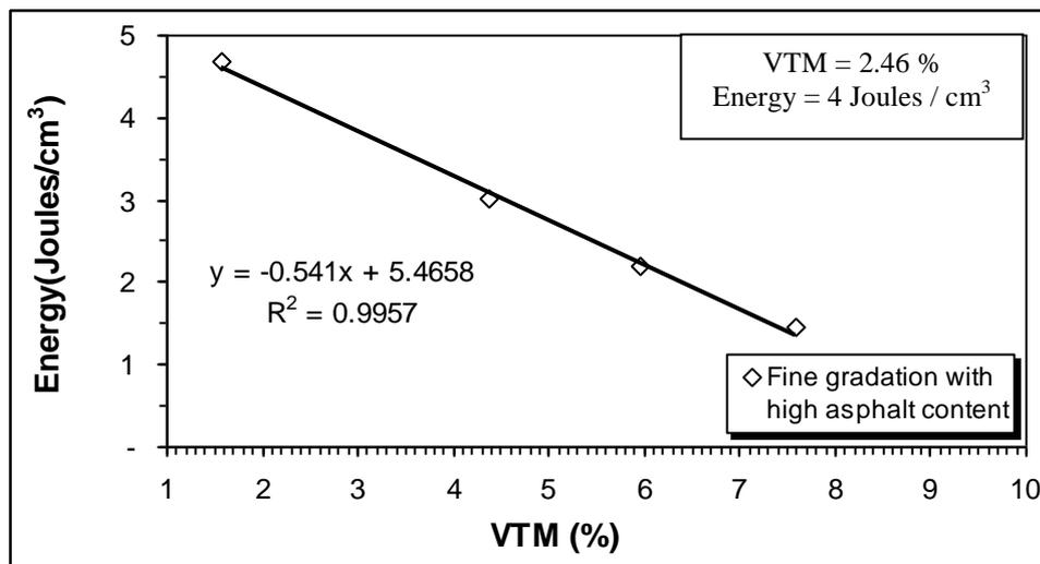
Figure A1 Graph for fine graded short specimen with high asphalt content,
