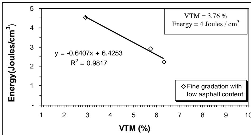
Figure A3 Graph for fine graded tall specimen with low asphalt content,
