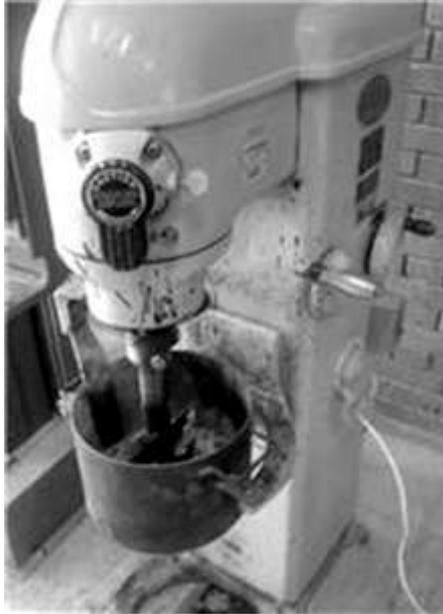
**Figure 3.2 Mixer used for mixing bitumen with blended aggregates**
