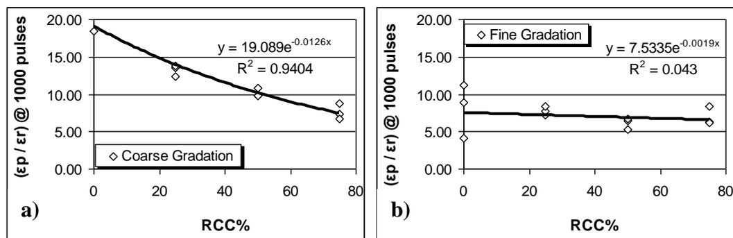
**Figure 5.5  $\epsilon_p / \epsilon_r$  @ 1000 cycles vs. RCC content a) for coarse graded specimens, b) for fine graded specimens**
