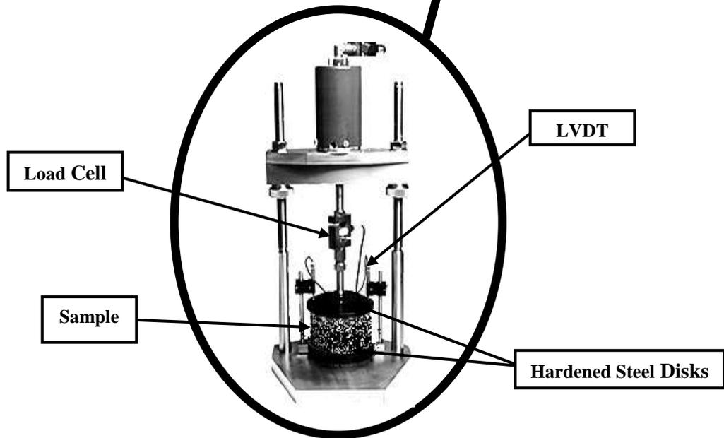
Figure 3.16 Repeated creep test setup
