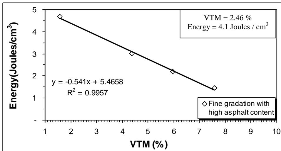
Figure A11 Graph for fine graded tall specimen with high asphalt content,
