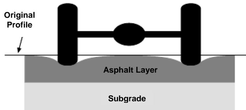
**Figure 2.6 Rutting due to consolidation (Superpave Mix Design Superpave Series No. 2 (SP-2), Asphalt Institute)**
