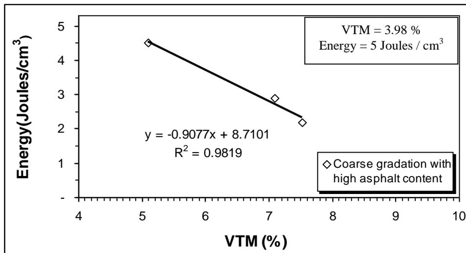
Figure A5 Graph for coarse graded tall specimen with high asphalt content,
