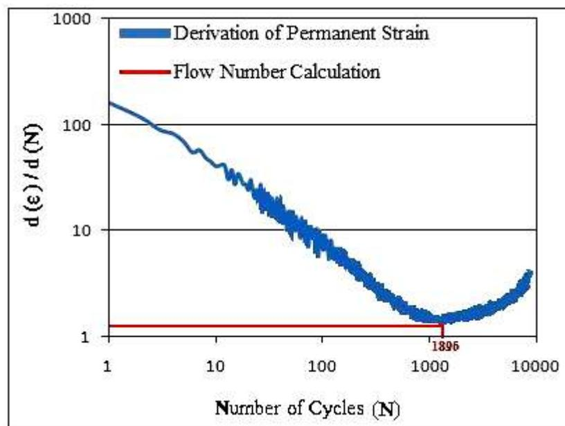
**Figure 3.12 Calculation of flow number for fine graded specimen with 75 %
