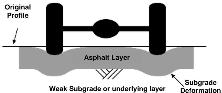
**Figure 2.9 Structural rutting (Superpave Mix Design Superpave Series No. 2 (SP-2), Asphalt Institute)**
