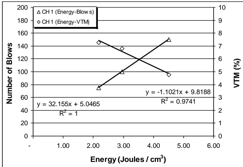
Figure A14 Graph for coarse graded tall specimen with high asphalt content, replicate 1
