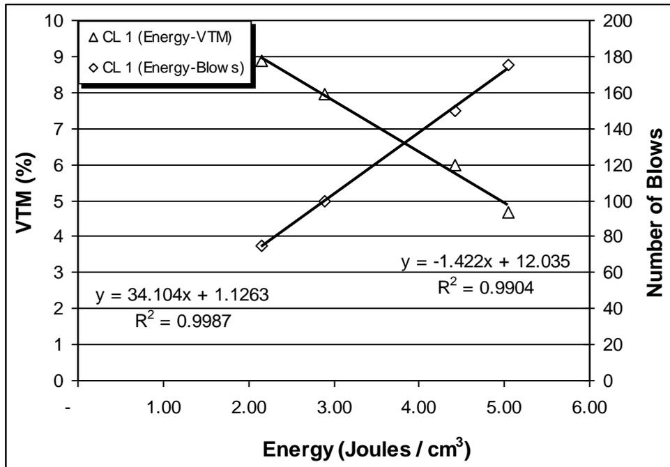
Figure A8 Graph for coarse graded tall specimen with low asphalt content, replicate 1
