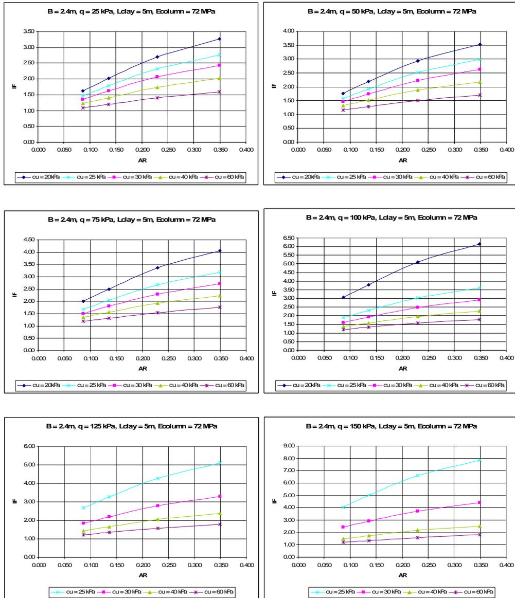
Figure B.2 Settlement improvement factor (IF) vs. area ratio (AR) charts for a rigid square footing ( $B=2.4\text{m}$ ) resting on end bearing rammed aggregate piers ( $L=5\text{m}$ ,  $E=72\text{ MPa}$ )
