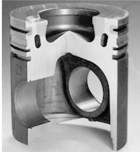
**Figure 1.1** Partially short  $\text{Al}_2\text{O}_3$  fiber reinforced aluminum diesel piston [4].
