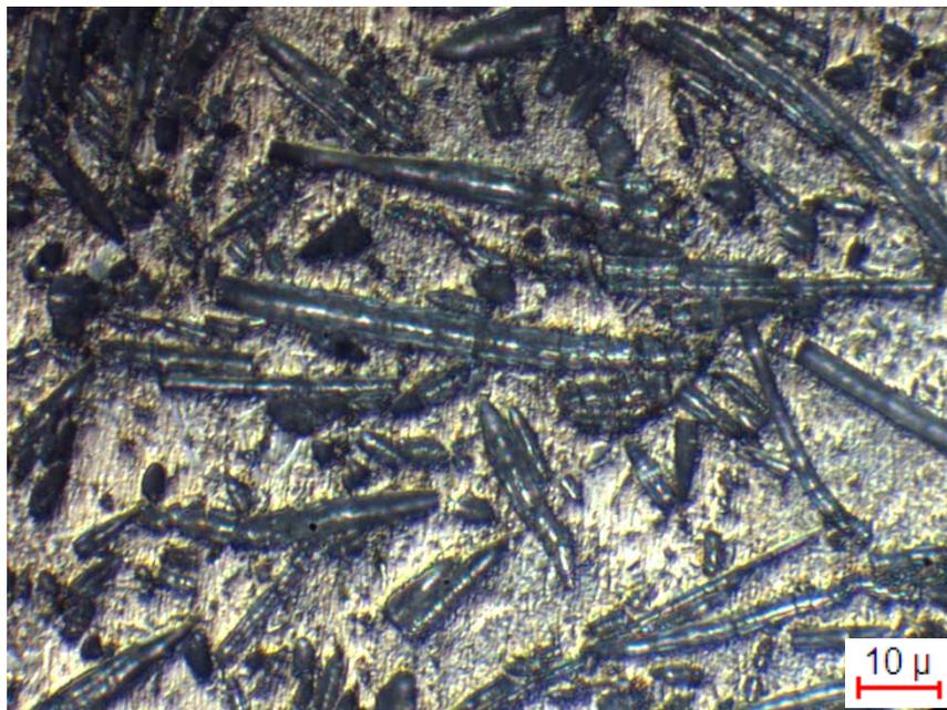
**Figure 4.54** Optical micrograph showing 30 vol% alumina fiber reinforced composite vertical to the fiber orientation at 500X magnification.
