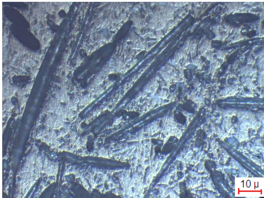
**Figure 4.42** Optical micrograph showing 20 vol% alumina fiber reinforced composite vertical to the fiber orientation at 500X magnification.
