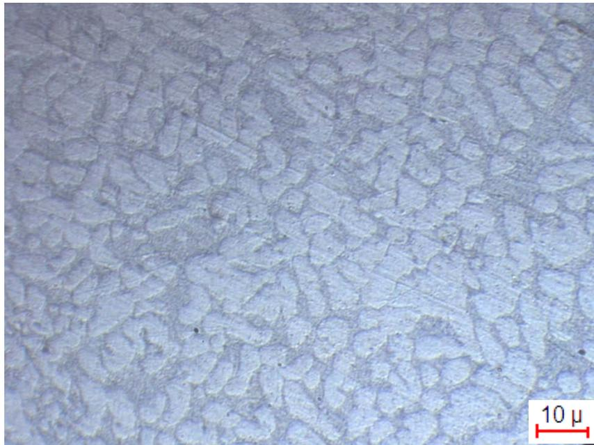
**Figure 4.60** Optical micrograph showing non-reinforced alloy at 500X magnification.
