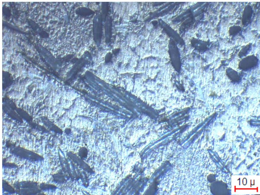
**Figure 4.30** Optical micrograph showing 10 vol% alumina fiber reinforced composite vertical to the fiber orientation at 500X magnification.
