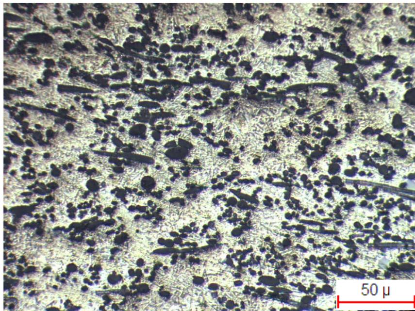
**Figure 4.50** Optical micrograph showing 25 vol% alumina fiber reinforced composite parallel to the fiber orientation at 200X magnification.
