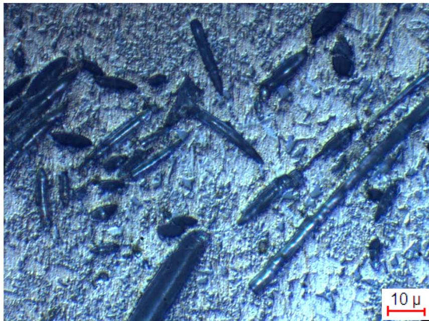
**Figure 4.36** Optical micrograph showing 15 vol% alumina fiber reinforced composite vertical to the fiber orientation at 500X magnification.
