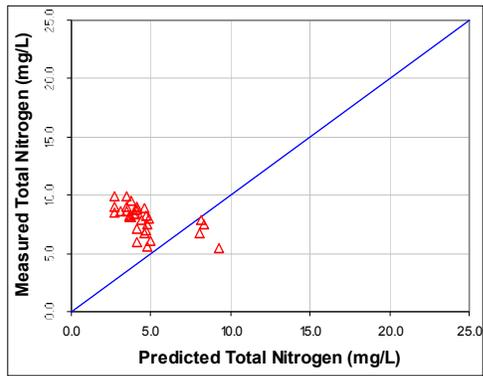
**Figure E.34 Predicted Total N versus Measured Total N for Relative Sum of Squares Results**
