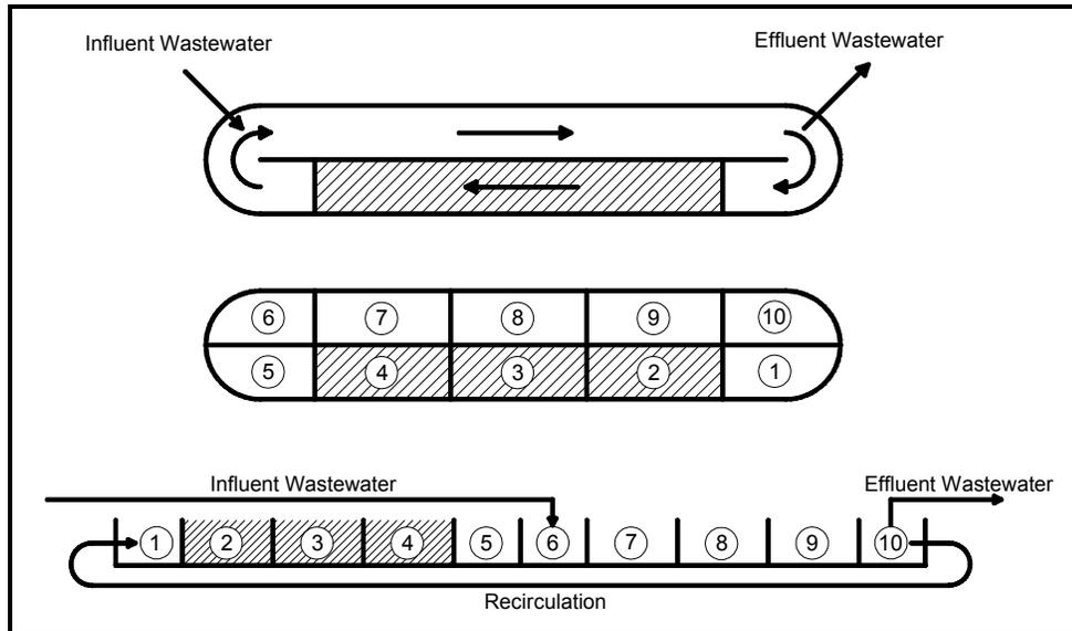
**Figure 6.24 Conceptual Internal Layout of the Aeration Tanks**
