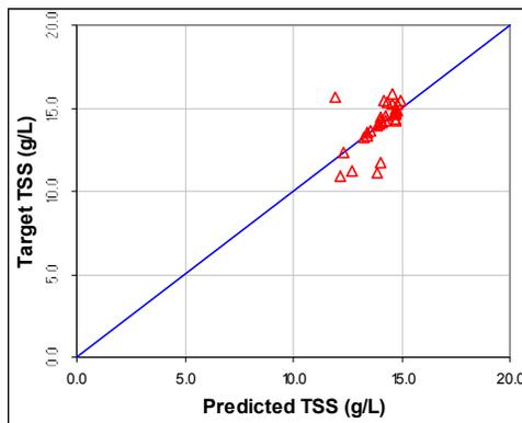
**Figure C.12 Predicted TSS versus Measured TSS for Maximum Likelihood Results**
