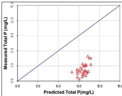
**Figure I.9 Predicted versus Measured Total Phosphorus in the Final Effluent**
