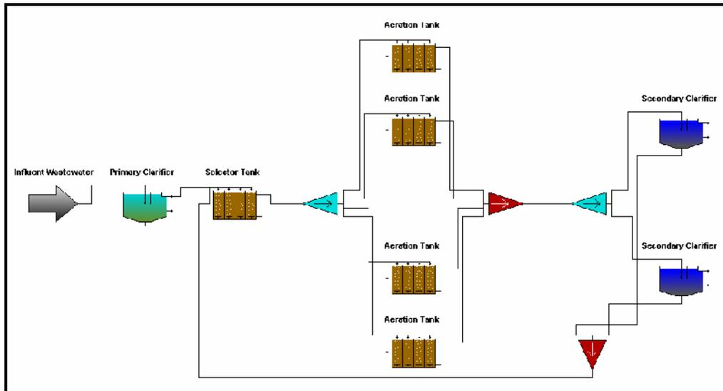
Figure 6.45 Layout of the Treatment Plant
