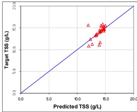
**Figure C.10 Predicted TSS versus Measured TSS for Relative Sum of Squares Results**
