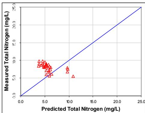
**Figure E.36 Predicted Total N versus Measured Total N for Maximum Likelihood Results**
