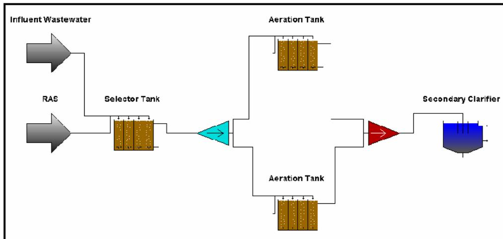
Figure 6.12 Layout for Secondary Clarifier
