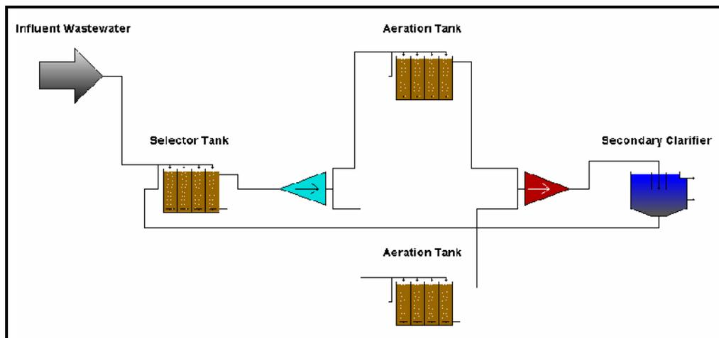
Figure 6.23 Layout for Selector Tank and Aeration Tanks
