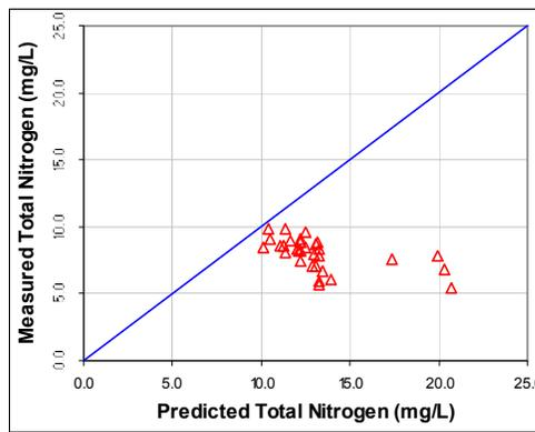
**Figure E.26** Predicted Total N versus Measured Total N for Default Values
