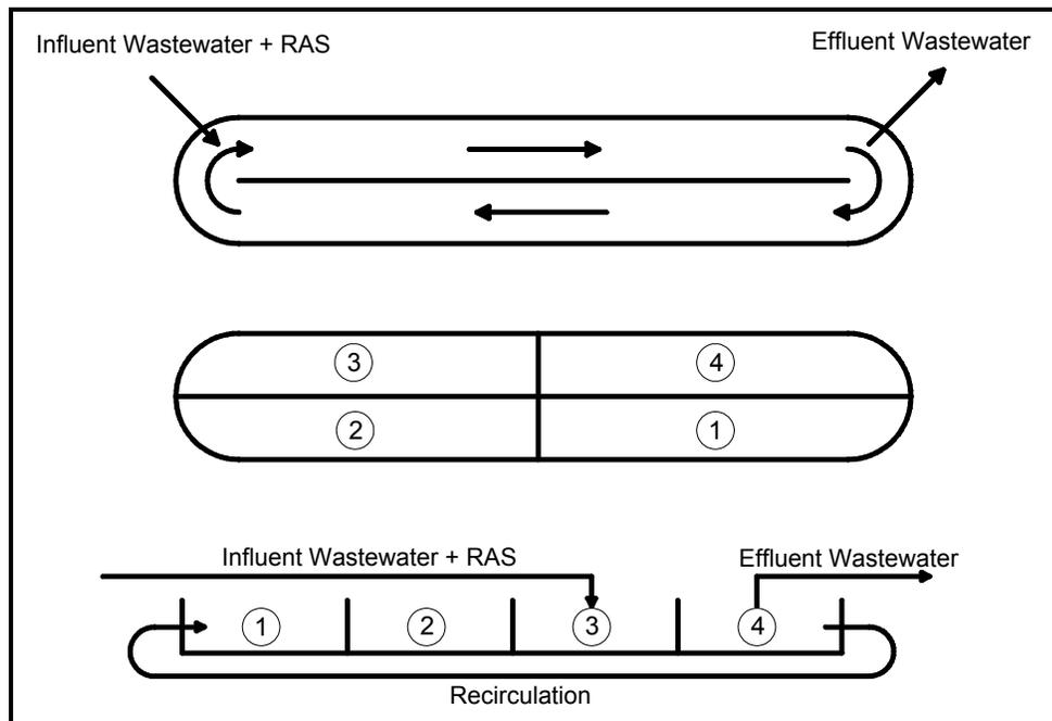
Figure 6.44 Conceptual Internal Layout of the Selector Tank
