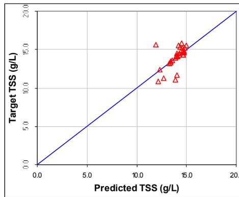
**Figure C.8 Predicted TSS versus Measured TSS for Sum of Squares Results**
