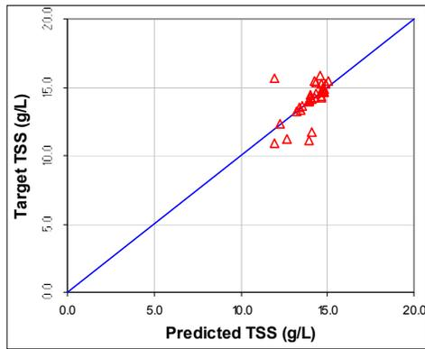
**Figure C.4 Predicted TSS versus Measured TSS for Absolute Difference Results**
