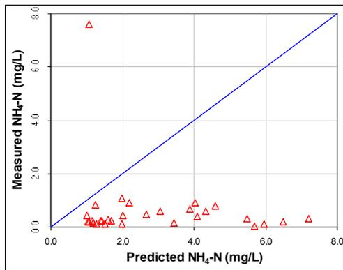
**Figure I.8 Predicted versus Measured  $\text{NH}_4\text{-N}$  in the Final Effluent**
