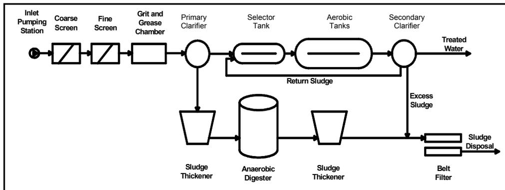
Figure 4.1 Flow Diagram of the Treatment Plant
