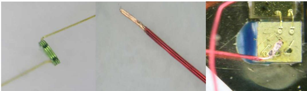
**Figure 4.2 An Air Core Coil, A Shelled Tip, And Wedge Bonding On A Capacitor**
