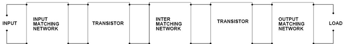
**Figure 3.5 The General Transistor Amplifier Circuit**
